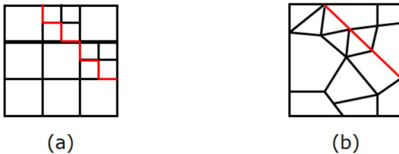
Figure 2.2. Representation of geological feature using structured Cartesian grid with refinement (a) versus unstructured grid (b) (after Moog, 2013).
