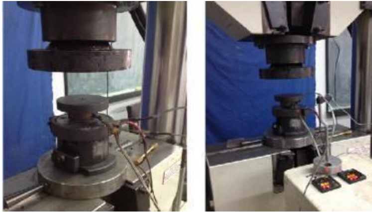
Figure 13: The die system used in surface modification
