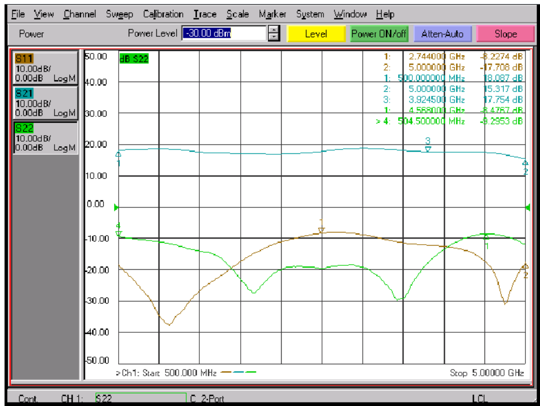
Figure 76 S-parameters Measurement of Cascaded Feedback Amplifier
