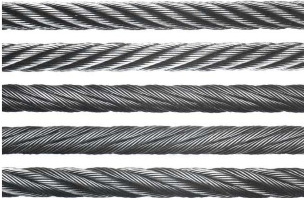
Figure 53. Strand lay configurations [24]
