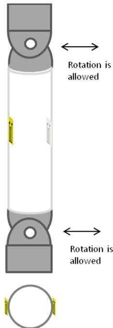
**Figure 42. Circular hollow section column bridge configuration**
