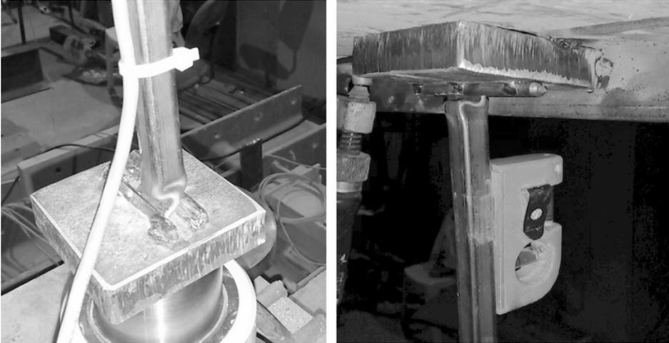
**Figure 34. End crushing of the column before plastic buckling load is reached**
