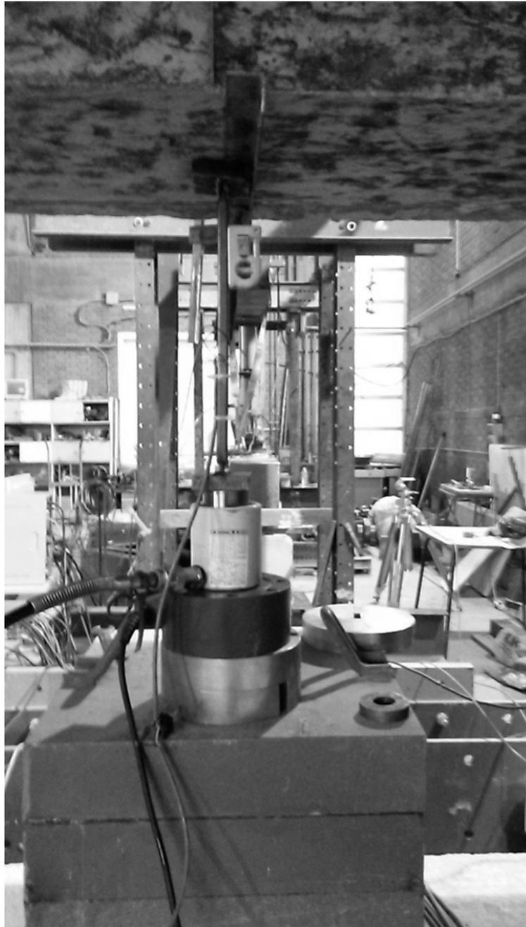
**Figure 33. Final test setup for plastic buckling**
