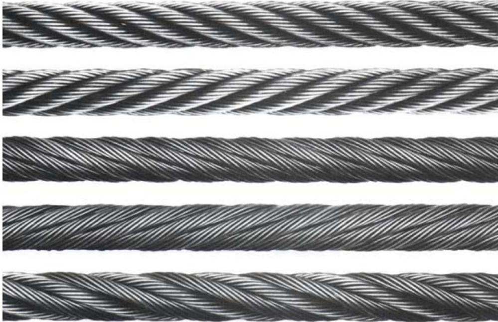
Figure 53. Strand lay configurations [24]
