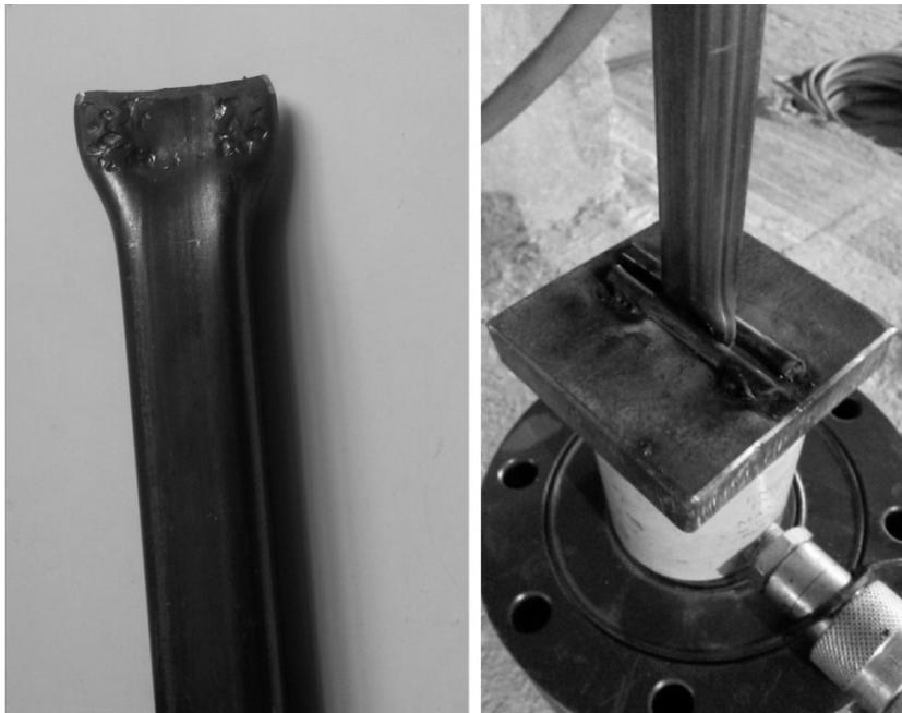
Figure 27. Hammered tip of column and guide plates
