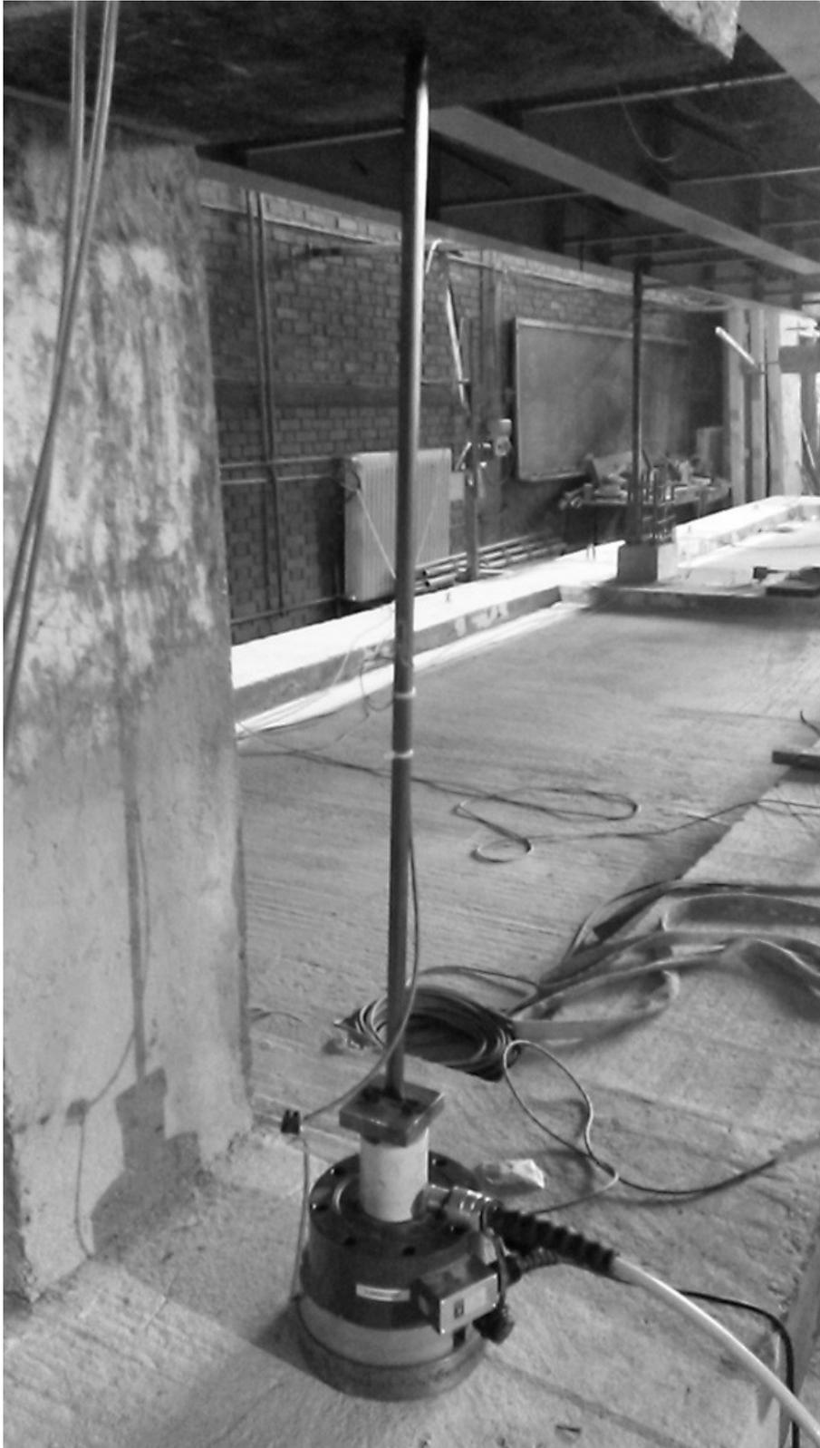
**Figure 30. Elastic buckling test setup**
