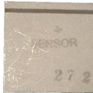
**Figure 3.4** Piezoelectric Patch (SensorTech - BM500 PZT Patch)
