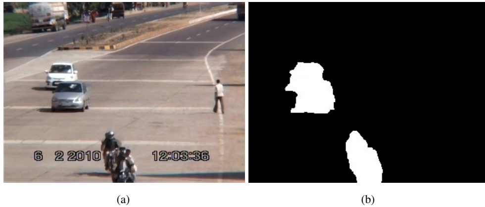
Figure 2.16: Binary mask under partial occlusion
