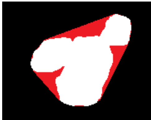
(c) Convex Hull and Defects
