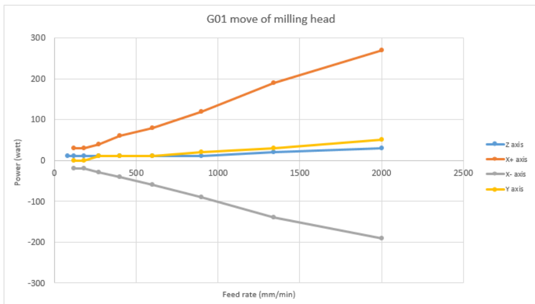
Figure 21 Average power consumption-feed rate graph for feed axis of milling head (G01)
