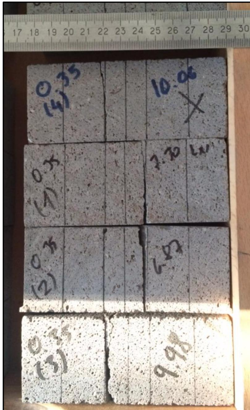
Figure B. 10  $W= 50$  mm  $a/W= 0.35$  specimens after test
