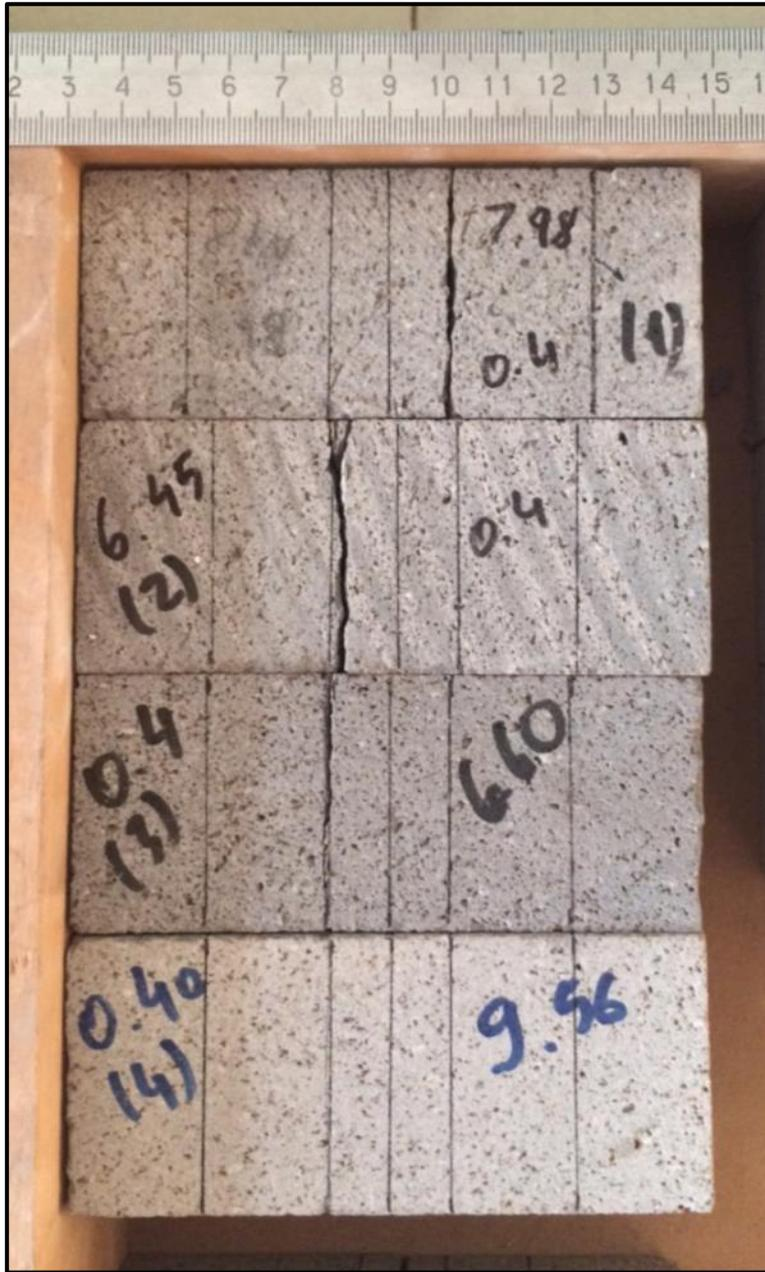
Figure B. 11  $W= 50$  mm  $a/W= 0.40$  specimens after test
