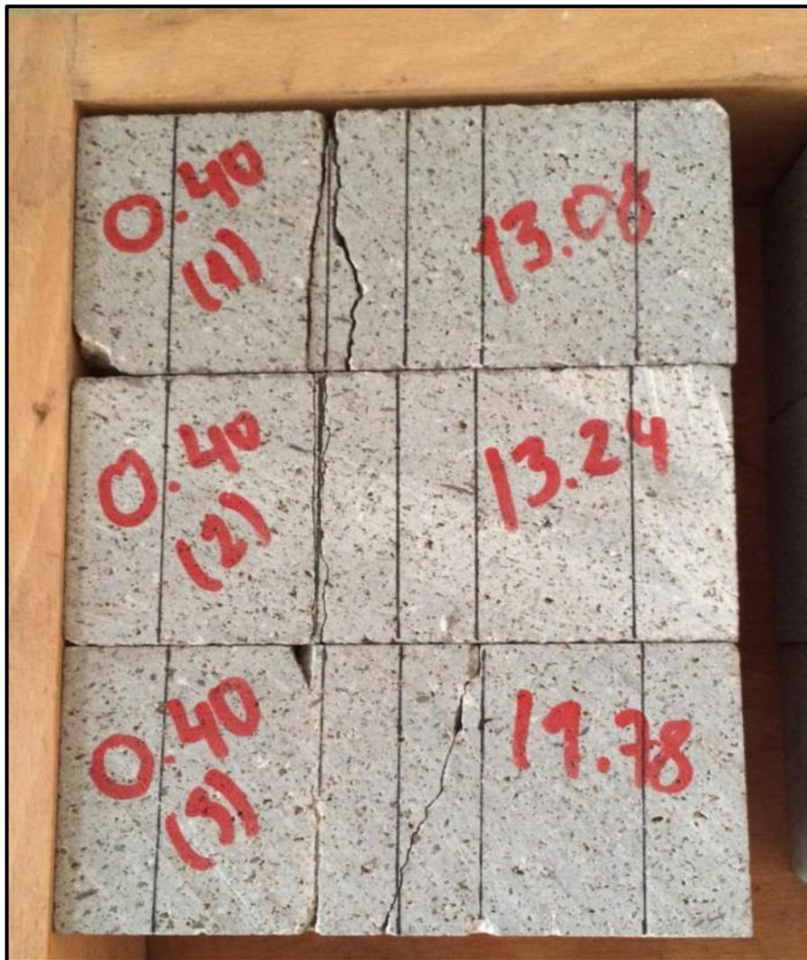
Figure B. 18  $W=60\text{ mm}$   $a/W=0.40$  specimens after test
