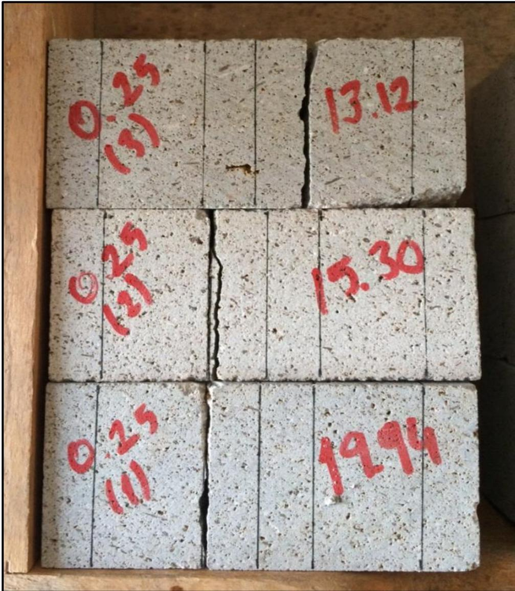
Figure B. 15 W= 60 mm a/W= 0.25 specimens after test
