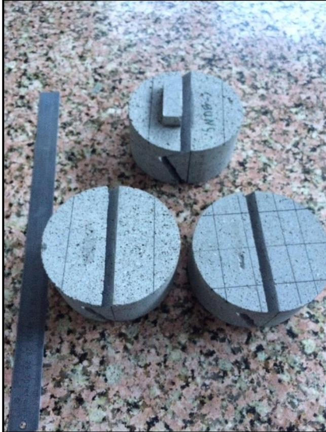
Figure 6. 13 Tested SNDB specimens
