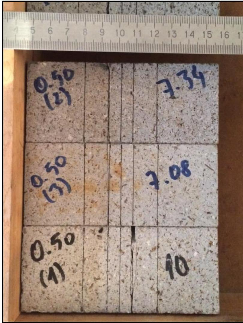
Figure B. 6  $W=40$  mm  $a/W=0.50$  specimens after test
