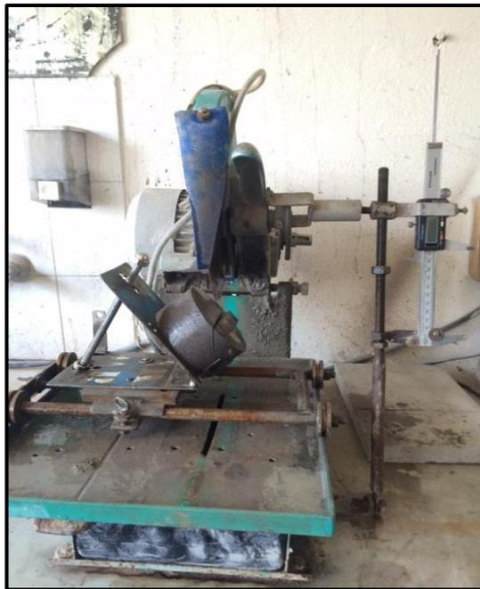
Figure 5. 3 Digital caliper adapted diamond circular saw
