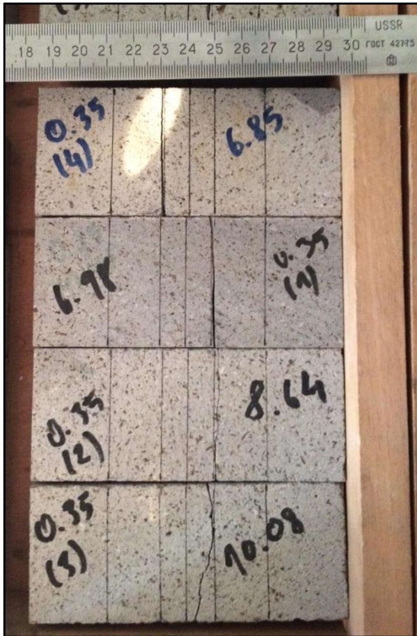
Figure B. 4  $W = 40$  mm  $a/W = 0.35$  specimens after test
