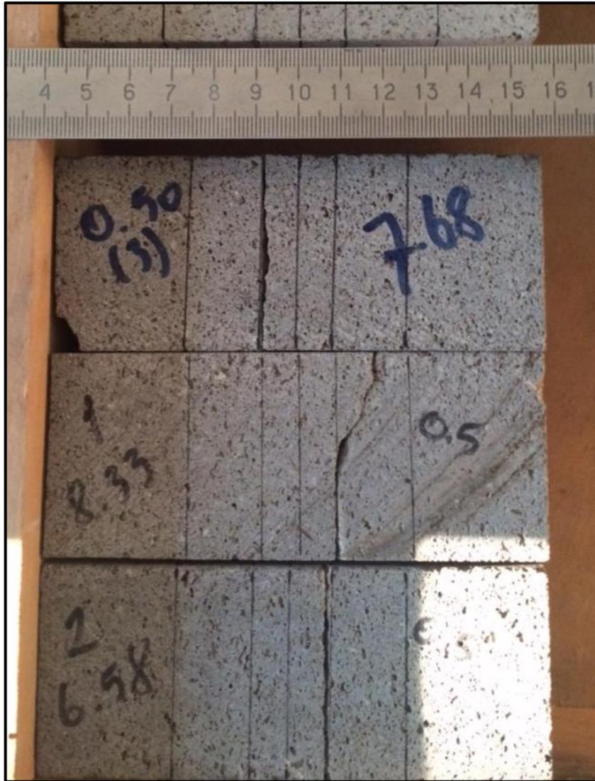
Figure B. 12  $W=50\text{ mm}$   $a/W=0.50$  specimens after test
