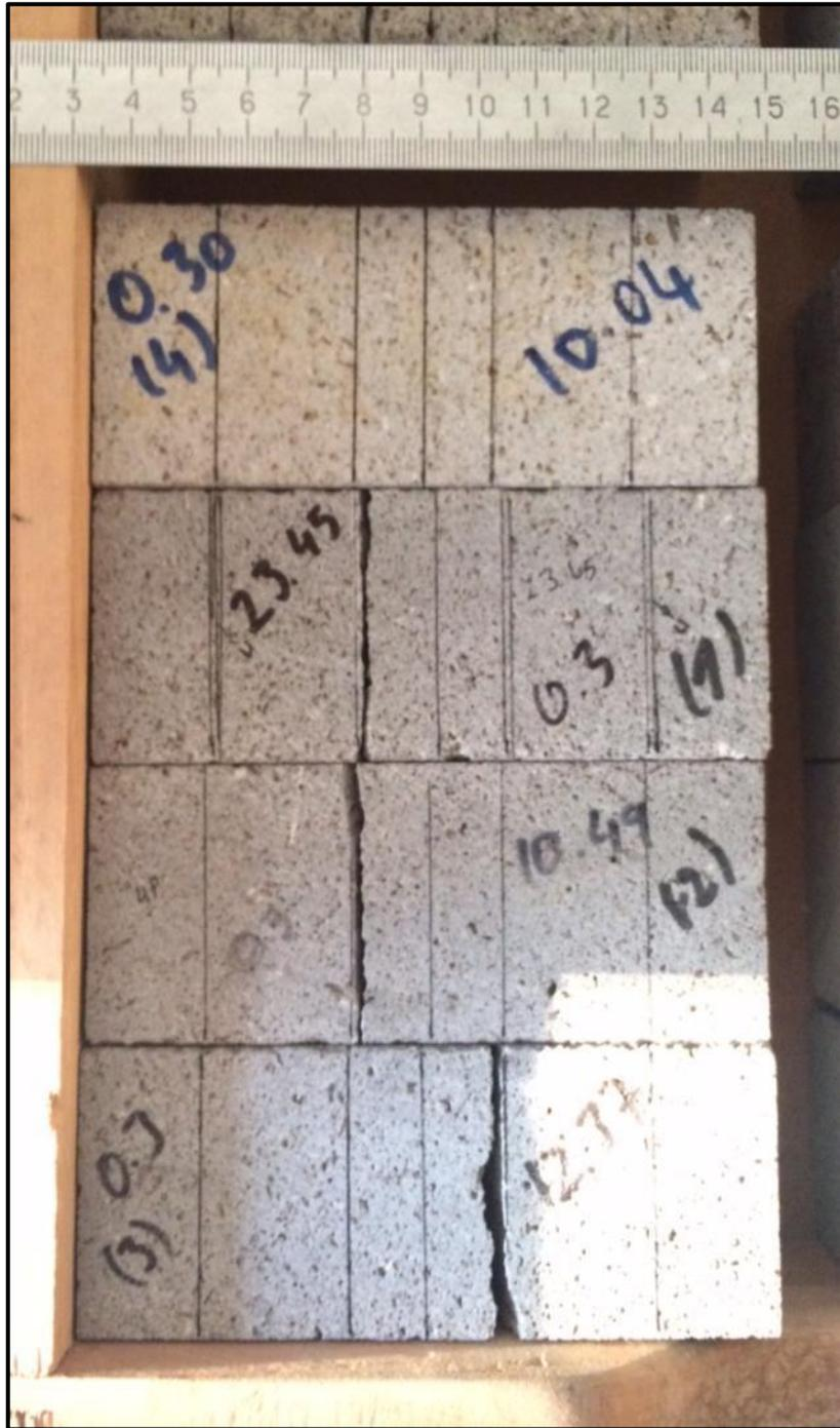
Figure B. 9  $W = 50 \text{ mm}$   $a/W = 0.30$  specimens after test
