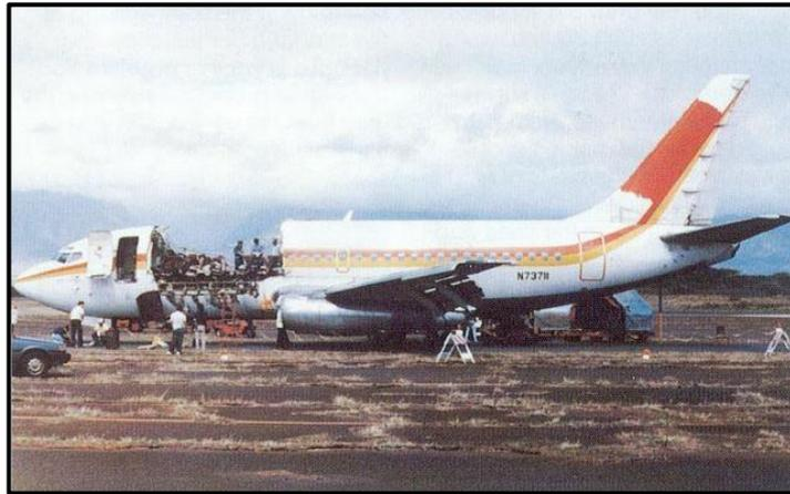
Figure 1. 3 Ripped off roof of Aloha's Aircraft (Adapted from National Geographic Channel documentary series “*Air Crash Investigation*” episode “*Hanging by Thread*”)
