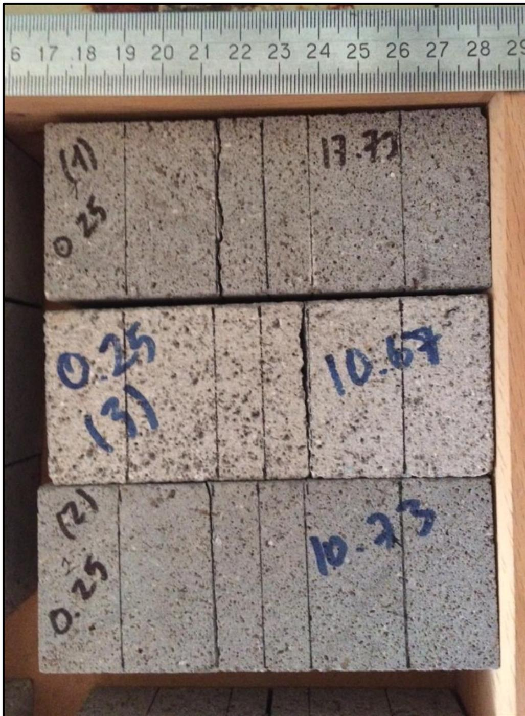
Figure B. 8  $W = 50$  mm  $a/W = 0.25$  specimens after test
