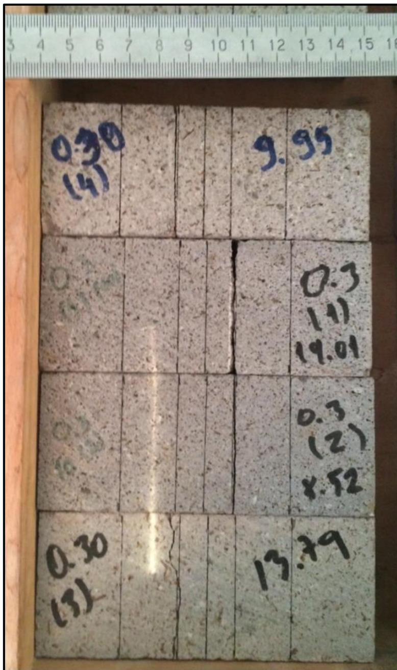
Figure B. 3  $W = 40$  mm  $a/W = 0.30$  specimens after test
