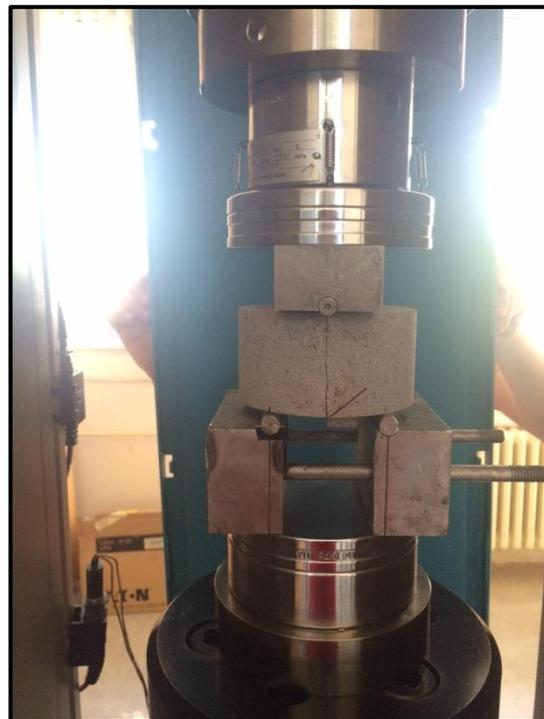
Figure 6. 12 Installation of SNDB test geometry
