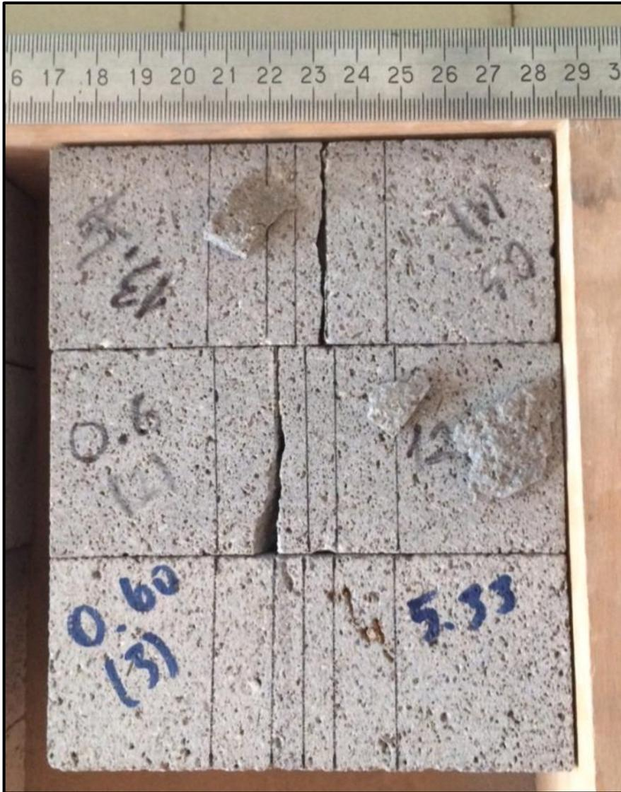
Figure B. 13  $W= 50 \text{ mm}$   $a/W= 0.60$  specimens after test
