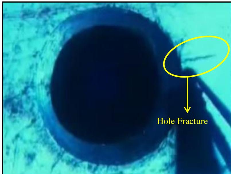
Figure 1. 5 Rivet hole fracture (Adapted from National Geographic documentary series “*Air Crash Investigation*” episode “Hanging by Thread
