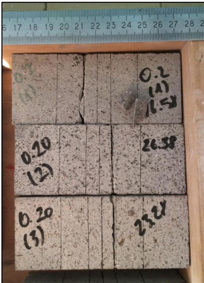
Figure B. 1 W= 40 mm a/W= 0.20 specimens after test
