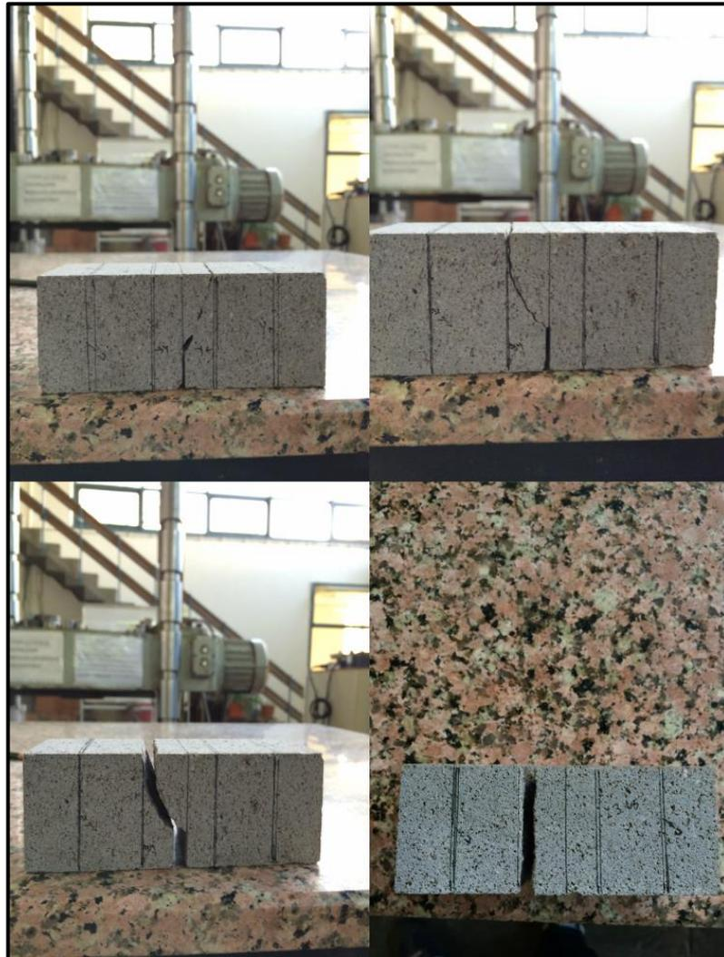
Figure 5. 14 FPAB test specimen after testing
