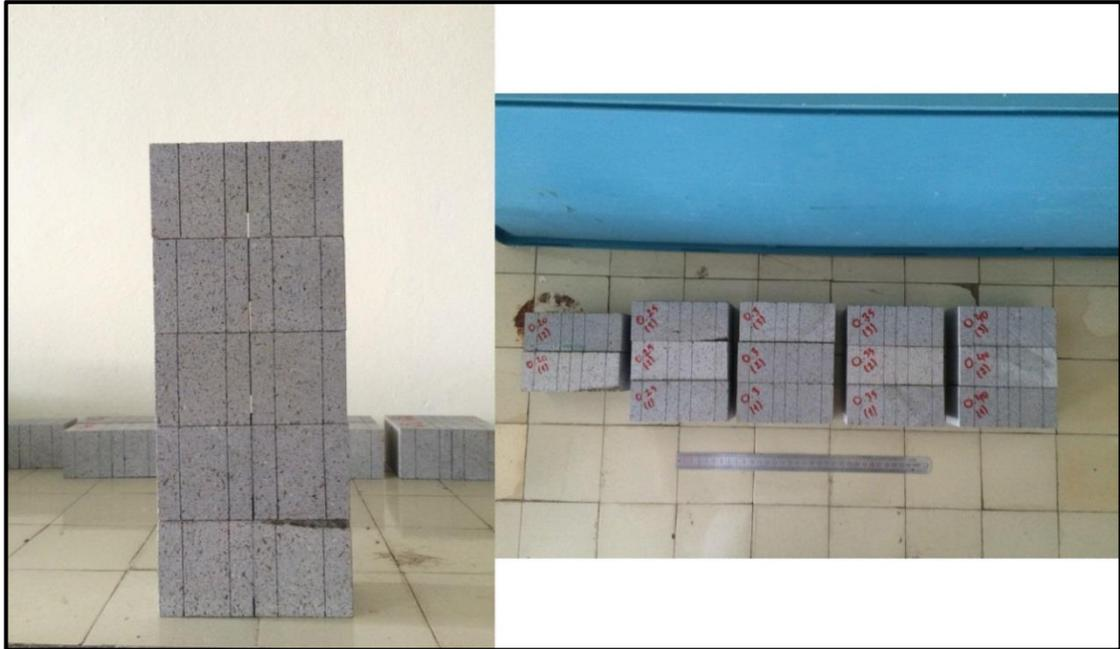
Figure 5. 10 Different notch lengths for beam depth group  $W= 60$  mm
