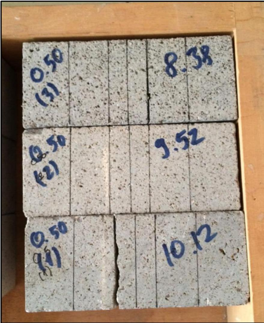
Figure B. 19  $W = 60$  mm  $a/W = 0.50$  specimens after test
