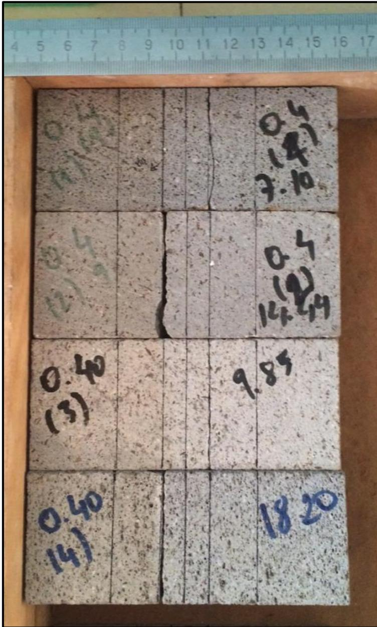
Figure B. 5  $W=40\text{ mm}$   $a/W=0.40$  specimens after test
