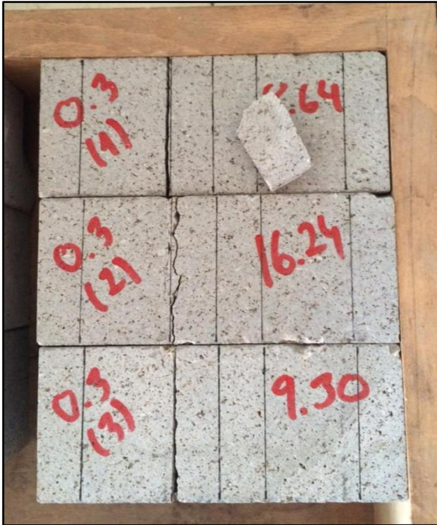
Figure B. 16  $W=60\text{ mm}$   $a/W=0.30$  specimens after test
