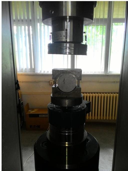
Figure 5. 8 Installation of Brazilian test
