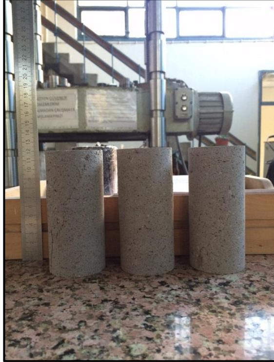
Figure 5. 5 After static deformability test rock core samples
