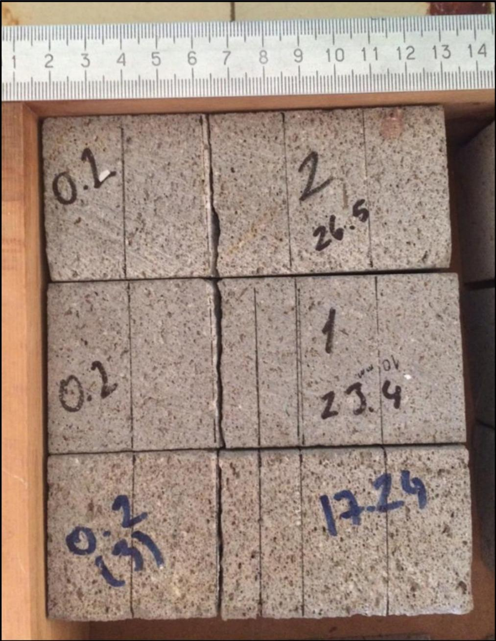
Figure B. 7 W= 50 mm a/W= 0.20 specimens after test
