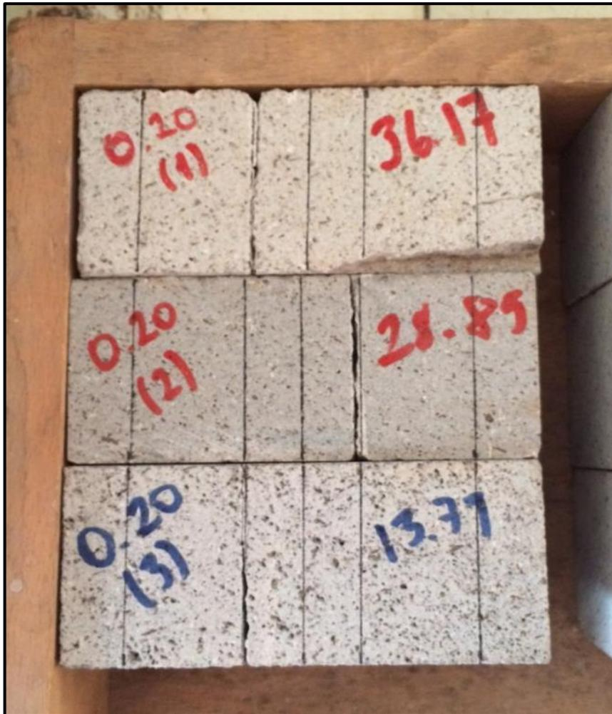
Figure B. 14 W= 60 mm a/W= 0.20 specimens after test
