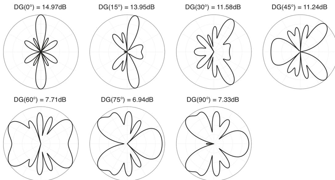
Figure 3.26: Radiation patterns obtained by dual-frequency optimizations of the array in Figure 3.21 at 5.80 GHz.
