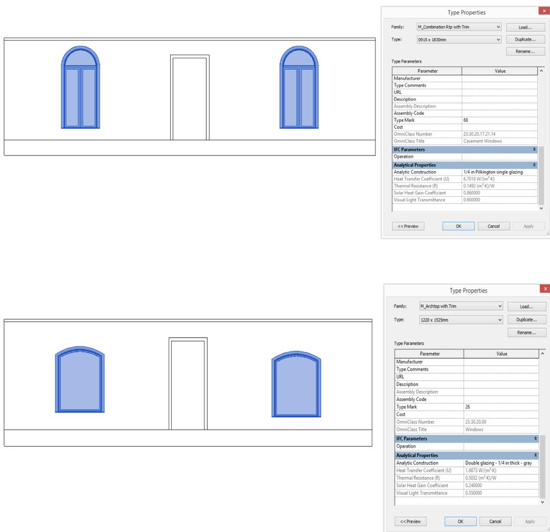
**Figure 5.19.** Window Property Change in BIM via Dynamo
