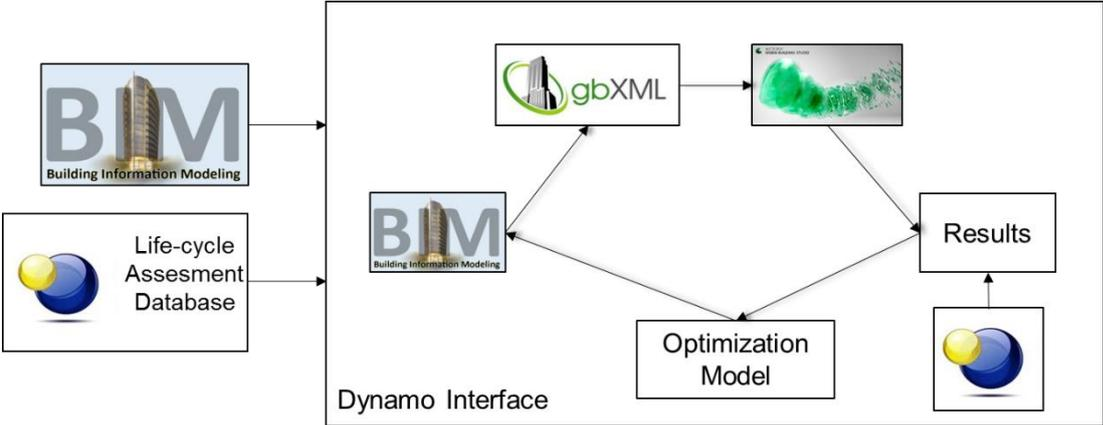
**Figure 5.22.** General Description of Dynamo based BIM Integrated Optimization Framework
