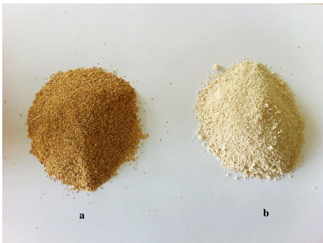
Figure D.1 Images of milled corn cobs a) Control b) Alkaline Pretreated
