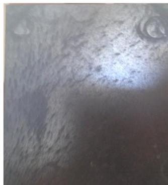
**Figure 68: Textured wafer with a solution consisting of 40ml IPA, 3.33wt % KOH, 15 min at 70°C**
