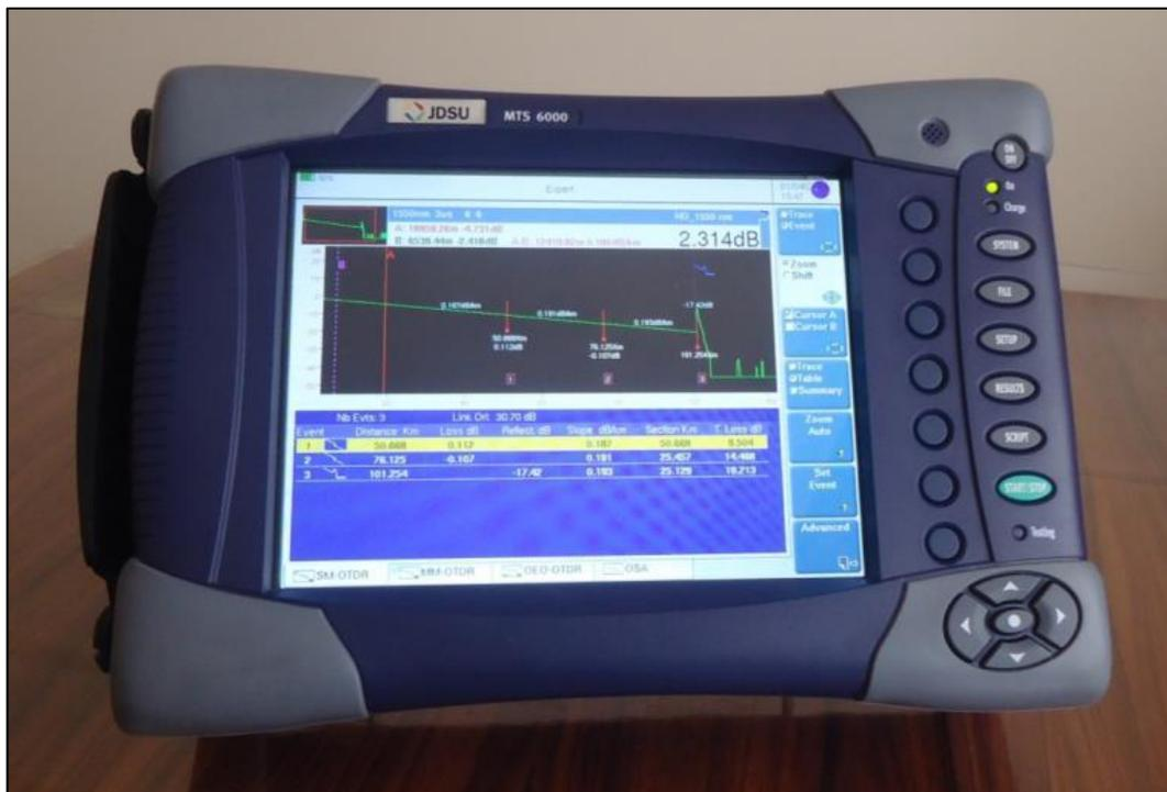
Figure 34: Optical Time Domain Reflectometer (OTDR)
