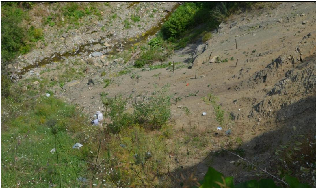
**Figure 52: Layout of the deployed fiber cables and fixing points (from scarp to toe)**
