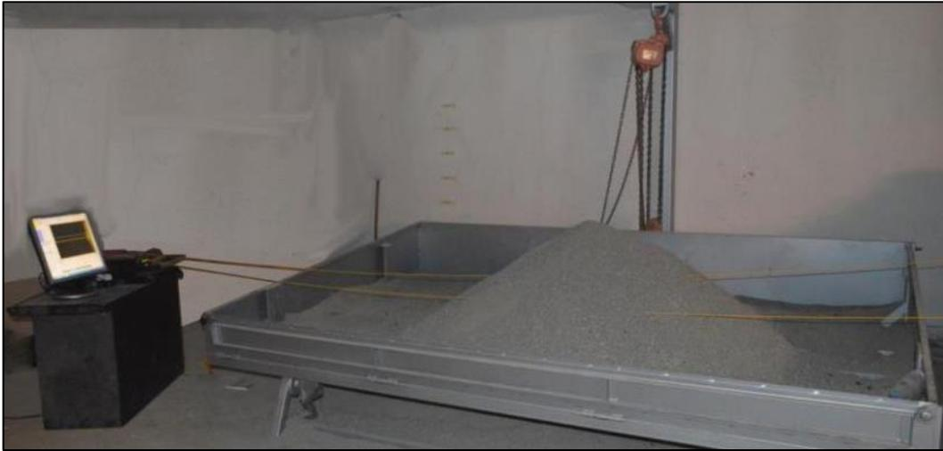
**Figure 46: Initial state of the BOTDA system on the laboratory simulator before sliding**
