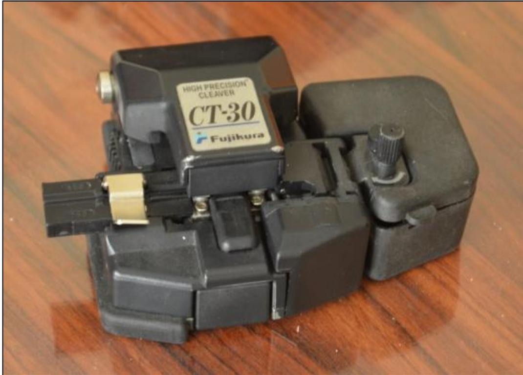
**Figure 37: Cleaver used to cut the fiber cables properly**
