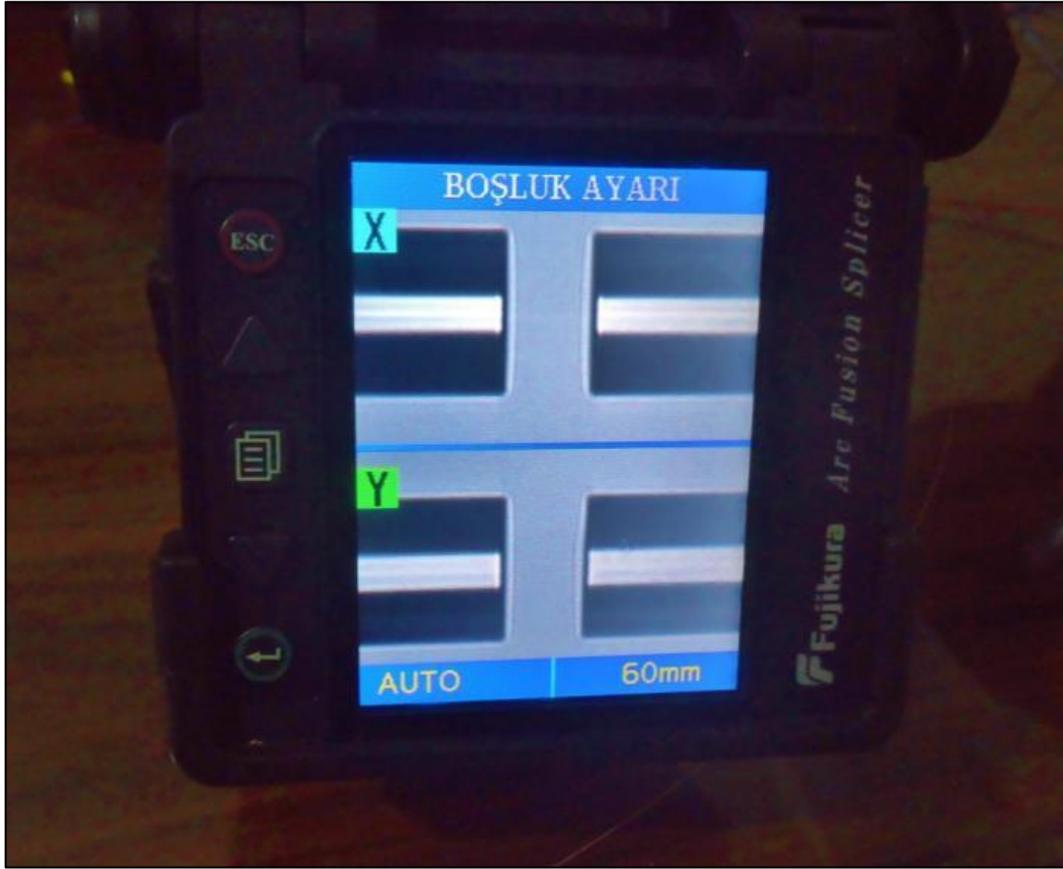
**Figure 36: The utilized fusion splicer (Fujikura FSM 60S) to fuse two cables without signal loss**
