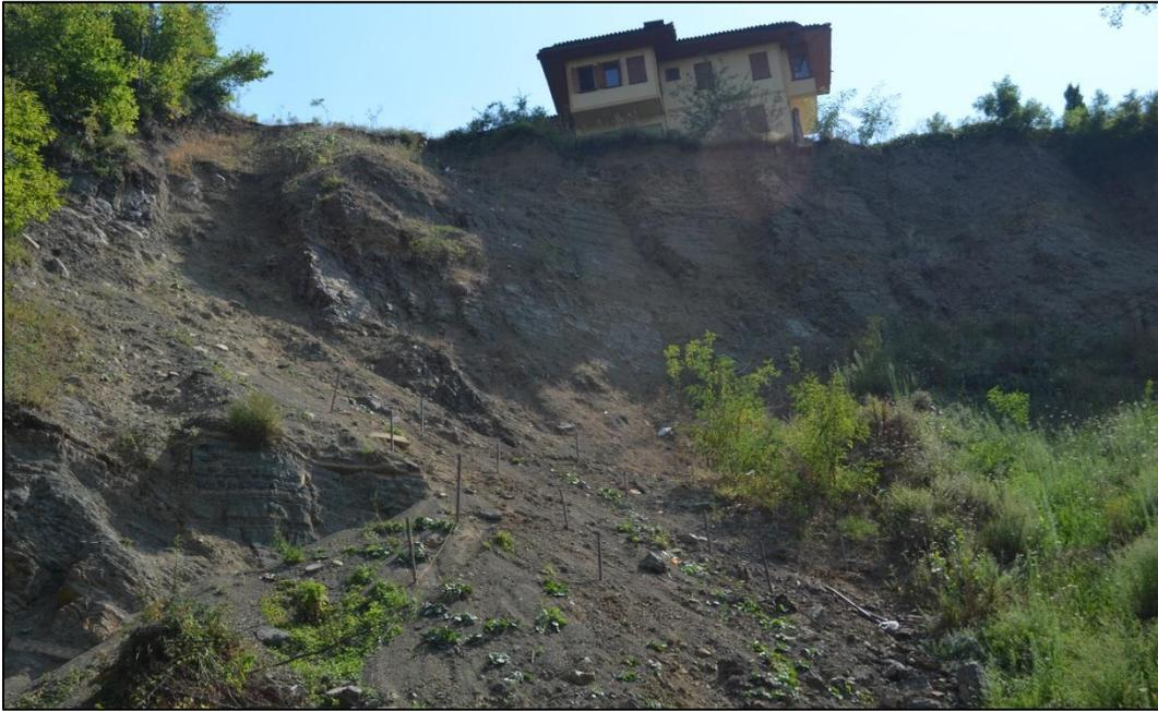
**Figure 51: Layout of the deployed fiber cables and fixing points (from toe to scarp)**
