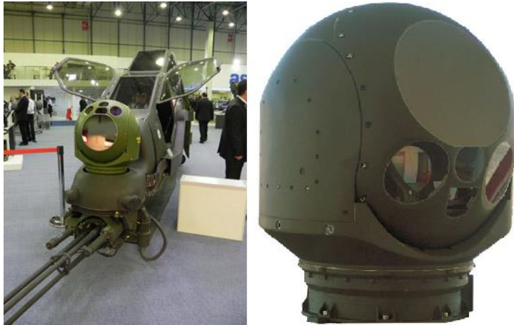
Figure 1.2 Integration of a turret system to a helicopter
