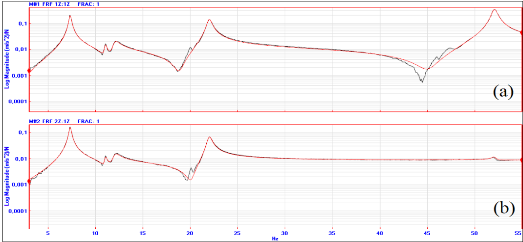
Figure 5.29 Synthesized and measured FRFs at nodes (a) 1 and (b) 2
