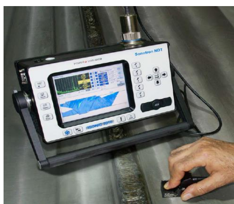
Figure 2.4 Manual Phased Array Equipment Sonotron Isonic 2010
