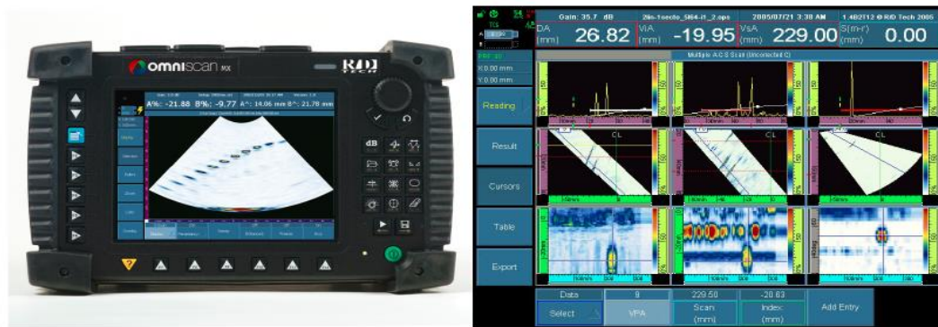
Figure 1.19 A commercial Phased Array instrument [11]
