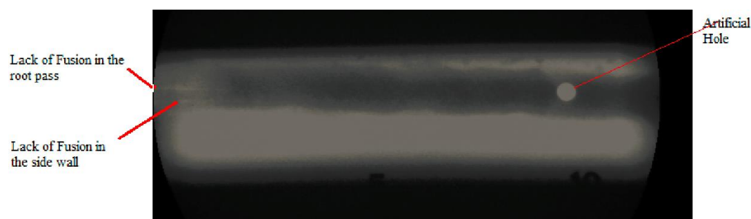
Figure 3.28 Radioscopic image of the specimen type 3 (200 kV)
