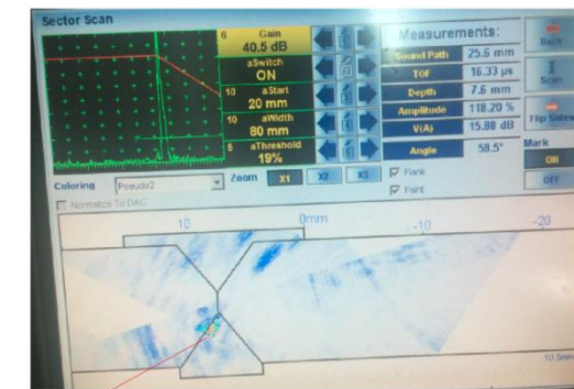
Figure 2.13 Manual Phased Array inspection
