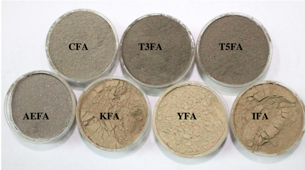
Figure 3.1 Fly ash samples.
