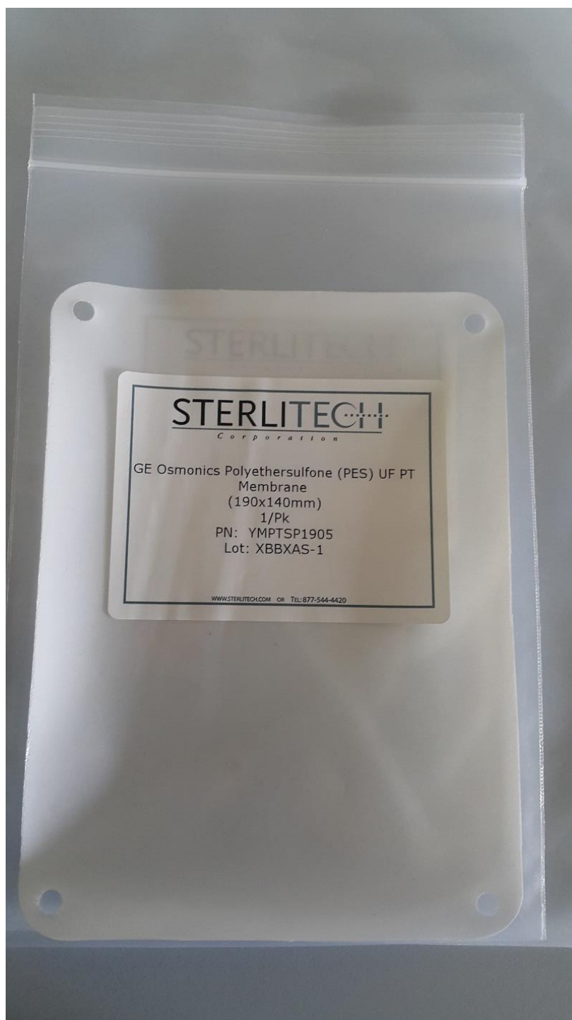
Figure 3.8. GE/Osmonics PT Membrane, Purchased from Sterlitech
