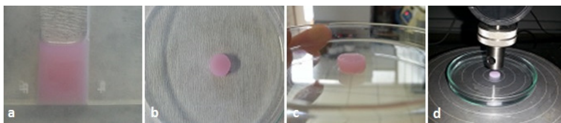
Figure 12. Sample preparation for mechanical test. a) Gelation in glass mold with 4 mm thickness. b) Punching disc shaped samples with 1 cm diameter. c) 3D structure of disc shaped sample. d) Uniaxial unconfined compression test in PBS.
