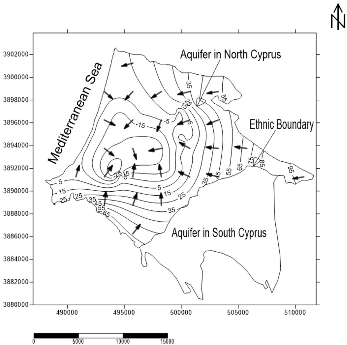
Figure 4.11 A flow net diagram representing groundwater flow in the wet season of 2013 in the study area.
