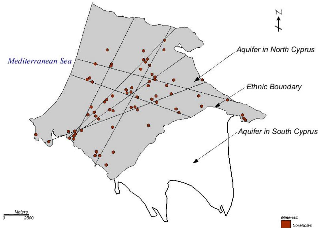
Figure 3.19 The seven transacts and the corresponding boreholes used to determine the areal distribution of aquifer material thickness.
