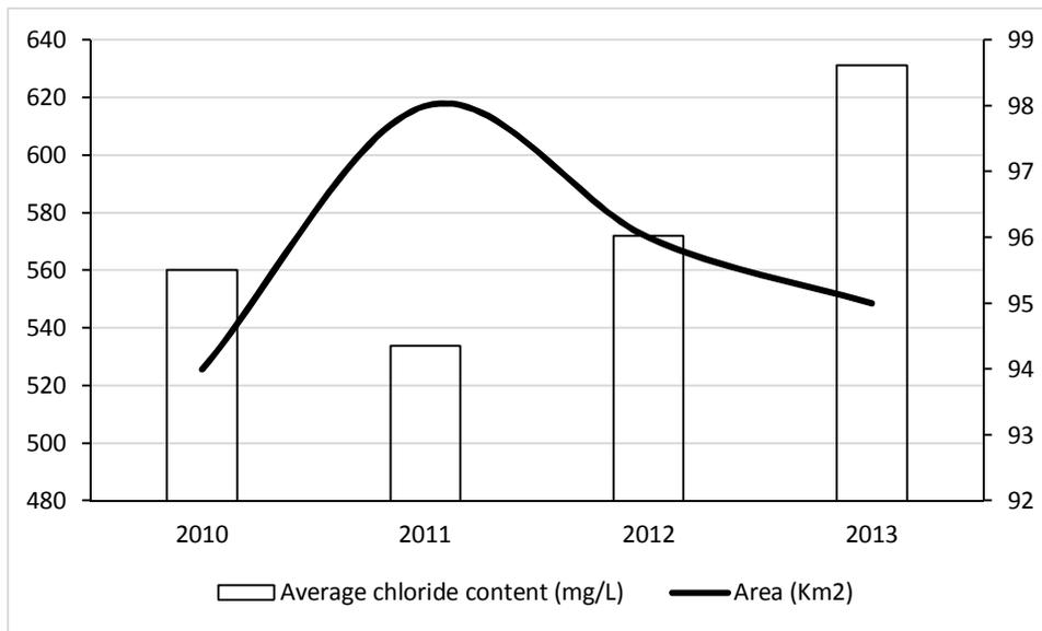
Figure 4.6 Average chloride concentration in mg/L from 2010 through 2013.
