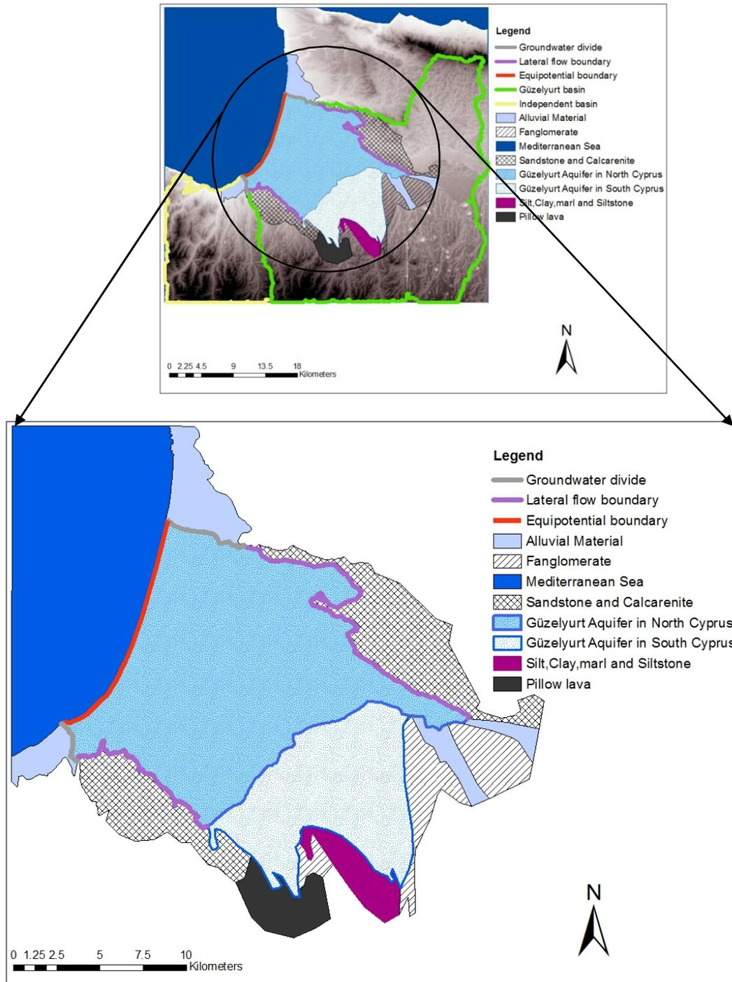
Figure 4.9 Güzelyurt Aquifer physical and hydraulic boundaries
