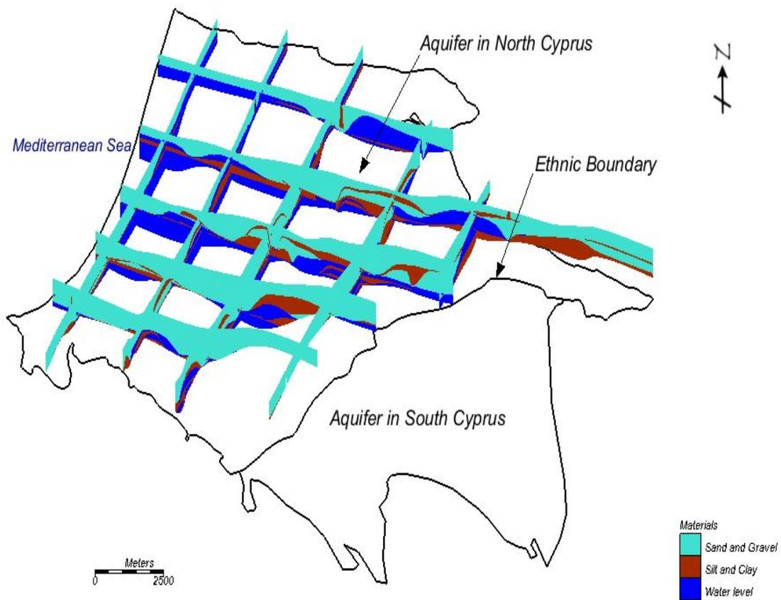
Figure 4.5 Saturated thickness of the aquifer generated using GIS for wet season water level data of 2013.
