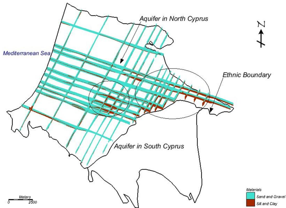
Figure 5.3 Identification of heterogeneous zones in Güzelyurt Aquifer (i.e., indicated by finer grids within the circled zones)
