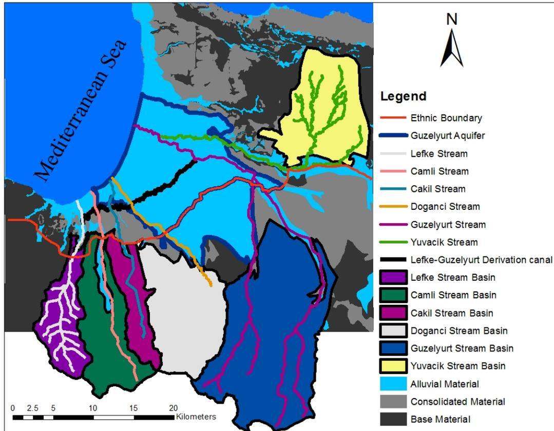
Figure 4.10 The six watershed basins delineated on impermeable formations where precipitation results in a direct runoff.
