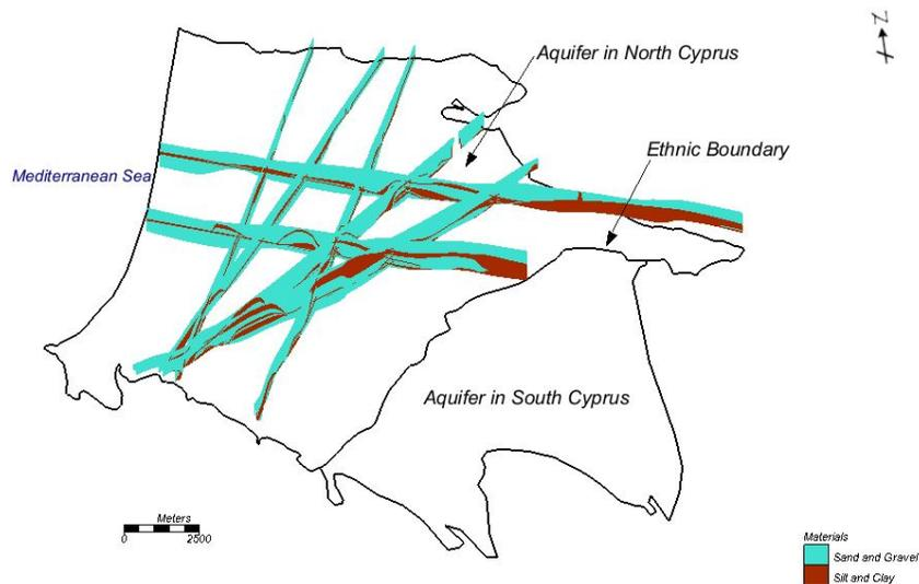
Figure 4.2 The cross-section of subsurface material showing aquifer material thickness in the study area
