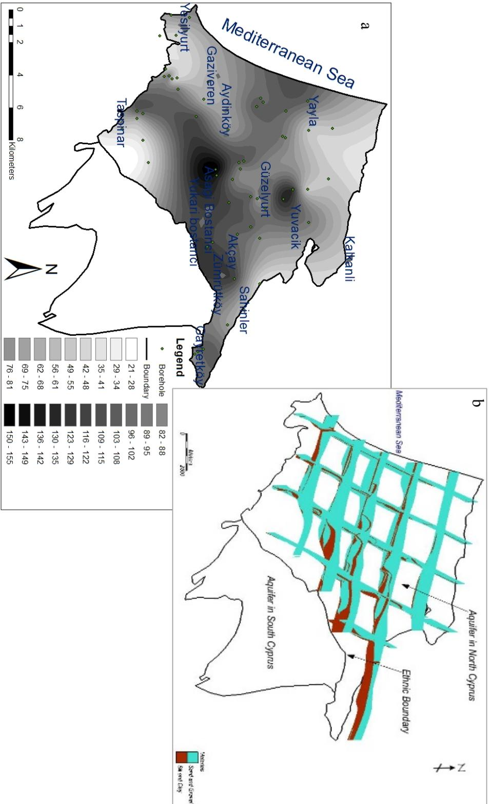
Figure 4.3 The aquifer material thickness distribution (a) and the cross-section of subsurface material showing aquifer material thickness (b) in the study area.
