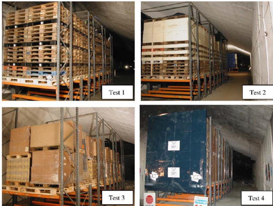
Figure 2.7 Photos of the test commodity used in the large-scale tests (Ingason & Lönnemark, 2005)
