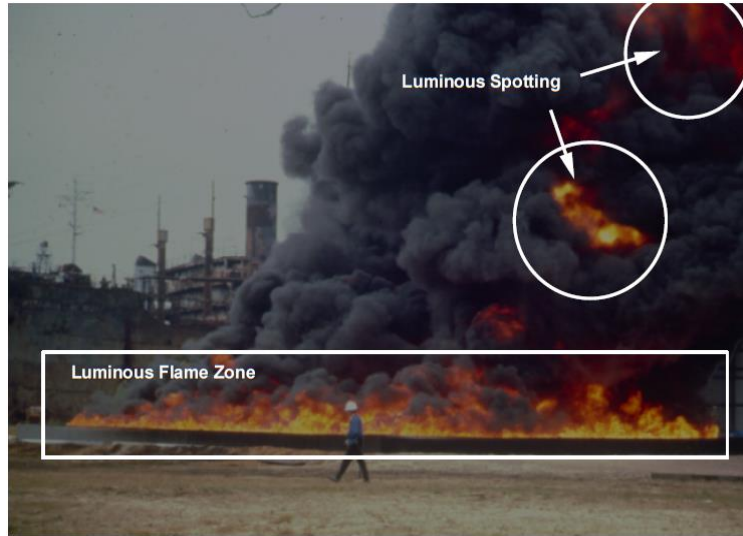
Figure 2.15 Photograph of a 15 m square fire of diesel fuel on water (McGrattan, Baum, & Hamins, 2000)
