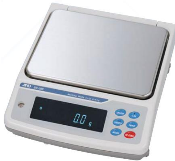
Figure 3.6 A&D GX-K series precision balance
