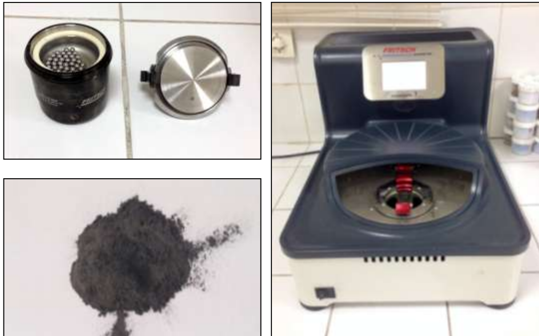
Figure 7. Fritsch Pulveristte 7 Premium Line High Energy Ball Mill, stainless steel bowl / balls and Ni-B powder mixture
