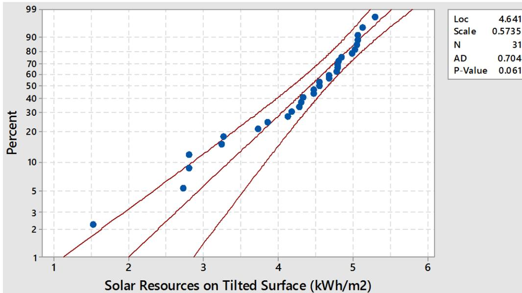
Figure D.2 Fitted Extreme Value distribution for solar resources on tilted surface for May
