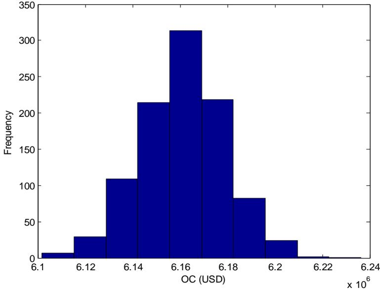
Figure 5.3 OC distribution for 1 MW solar PV plant at METU NCC with constant electricity prices
