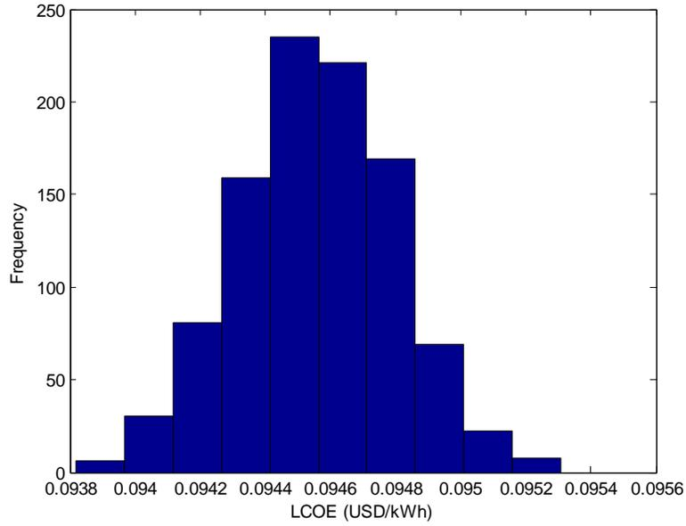
Figure 5.5 LCOE distribution for 1 MW solar PV power plant at METU NCC for increasing electricity prices at 12 % annual rate
