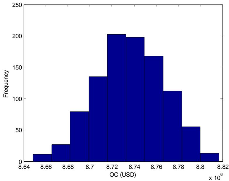
Figure 5.15 OC distribution for 1 MW solar PV power plant at METU NCC for constant demand and increasing electricity prices at 12 % annual rate
