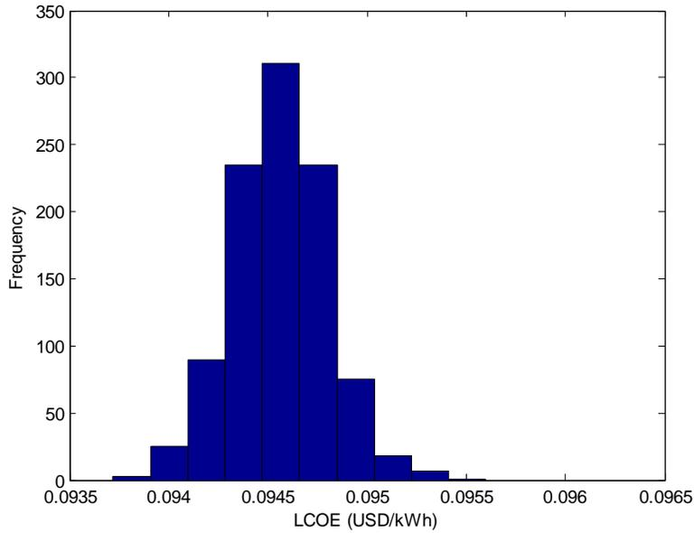
Figure 5.1 LCOE distribution for 1 MW solar PV plant at METU NCC with constant electricity prices
