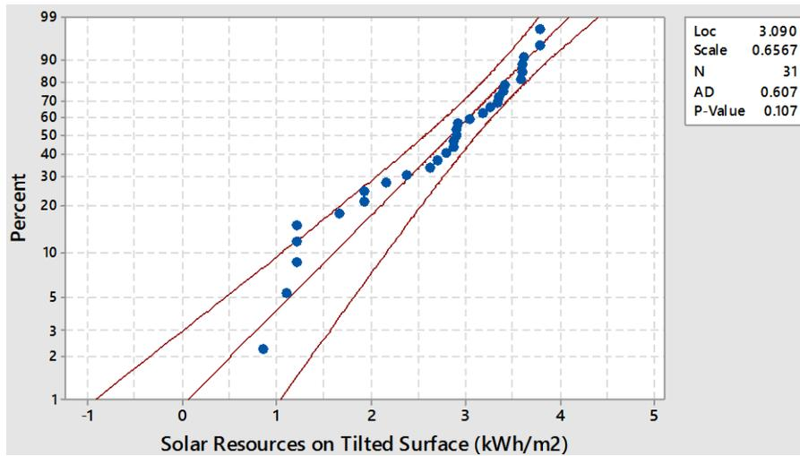
Figure 3.3 Fitted Extreme Value distribution for solar resources on tilted surface for January
