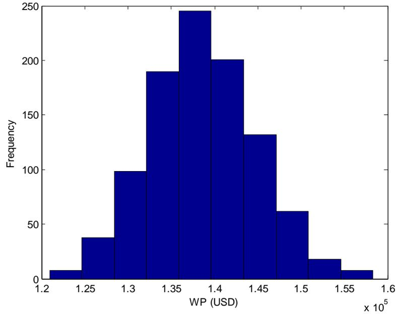
Figure 5.16 WP distribution for 1 MW solar PV power plant at METU NCC for constant demand and increasing electricity prices at 12 % annual rate
