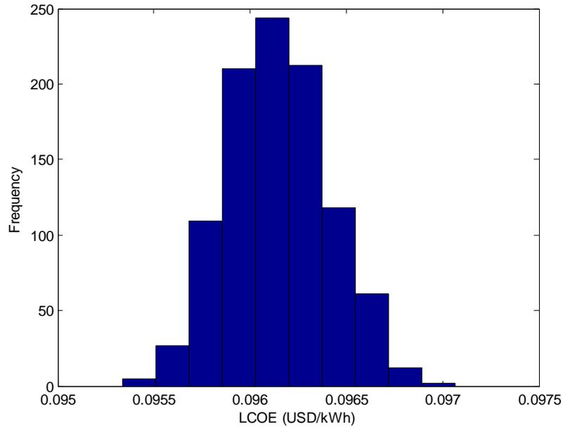
Figure 5.13 LCOE distribution for 1 MW solar PV power plant at METU NCC for constant demand and increasing electricity prices at 12 % annual rate
