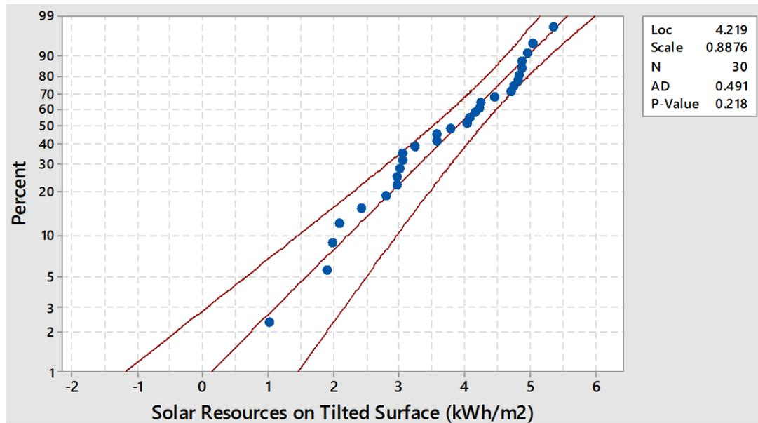
Figure D.8 Fitted Extreme Value distribution for solar resources on tilted surface for November
