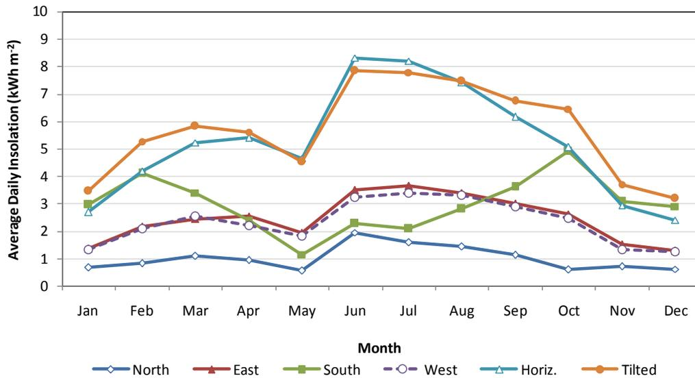
Figure 3.1 Trends in daily insolation for METU NCC. For the tilted surface  $\beta=24.67^\circ$  and  $\gamma=0^\circ$ .
