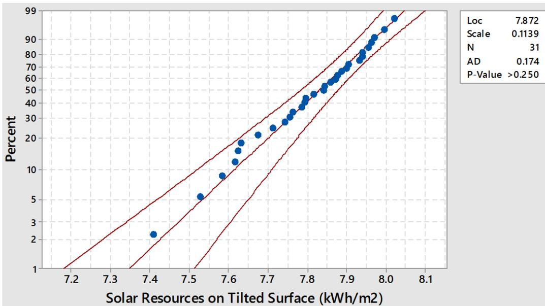
Figure D.4 Fitted Extreme Value distribution for solar resources on tilted surface for July
