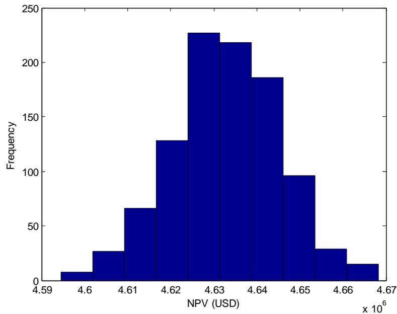
Figure 5.14 NPV distribution for 1 MW solar PV power plant at METU NCC for constant demand and increasing electricity prices at 12 % annual rate
