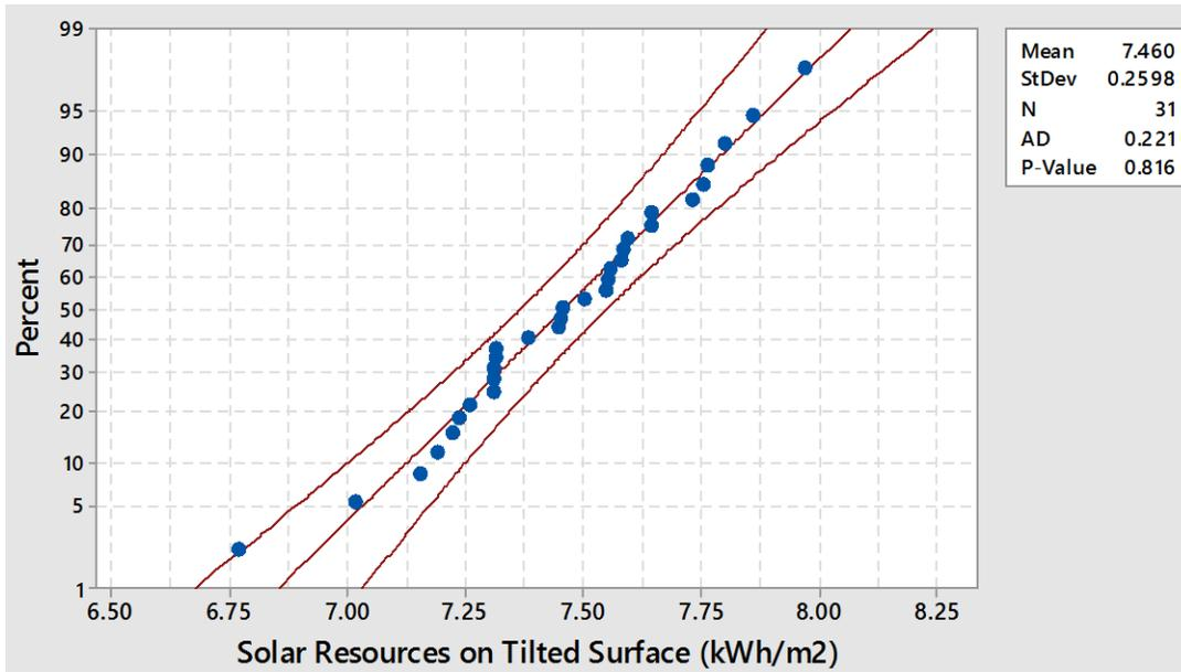
Figure D.5 Fitted Normal distribution for solar resources on tilted surface for August
