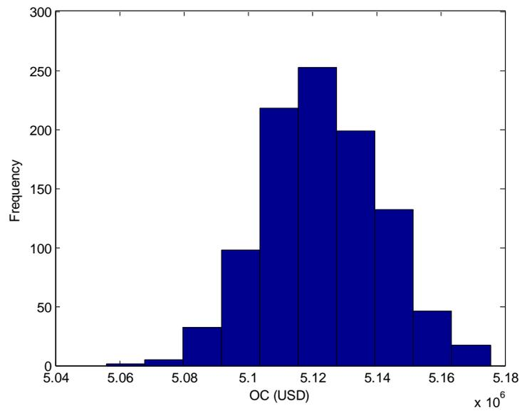
Figure 5.19 Distribution of OC for stepwise installation of solar PV plant at METU NCC with constant electricity prices
