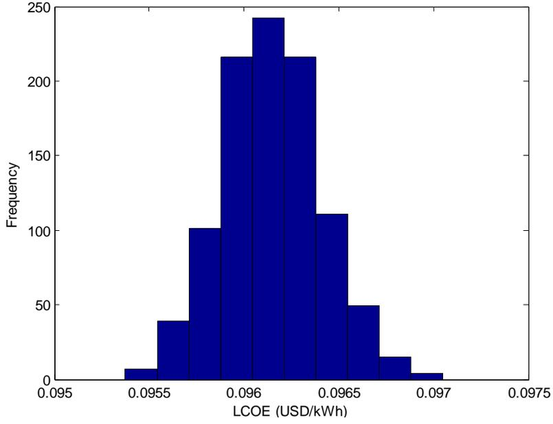
Figure 5.9 LCOE distribution for 1 MW solar PV power plant at METU NCC for constant electricity prices and demand
