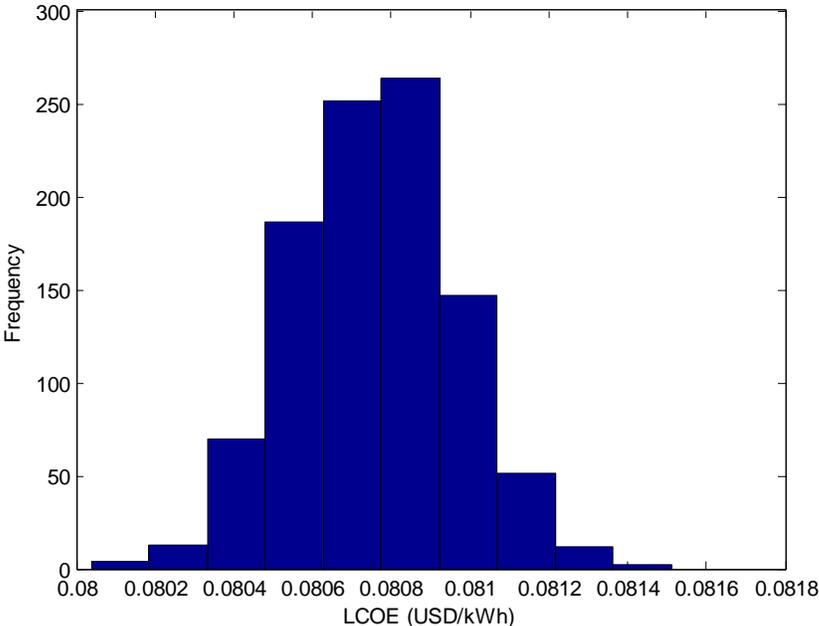
Figure 5.29 LCOE distribution for stepwise installation of solar PV power plant at METU NCC for constant demand and increasing electricity prices at 12 % annual rate
