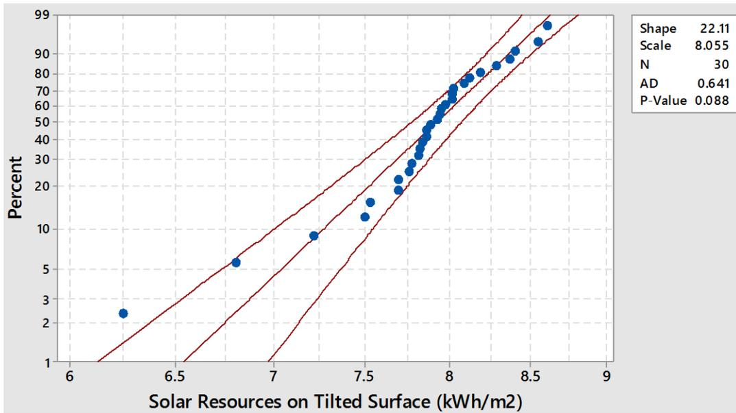
Figure D.3 Fitted Weibull distribution for solar resources on tilted surface for June
