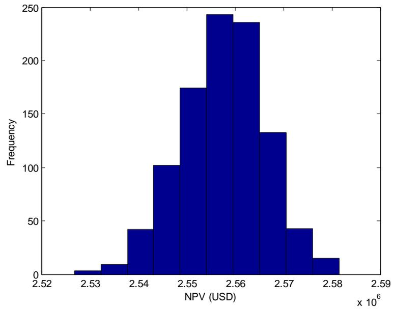
Figure 5.18 Distribution of NPV for stepwise installation of solar PV plant at METU NCC with constant electricity prices
