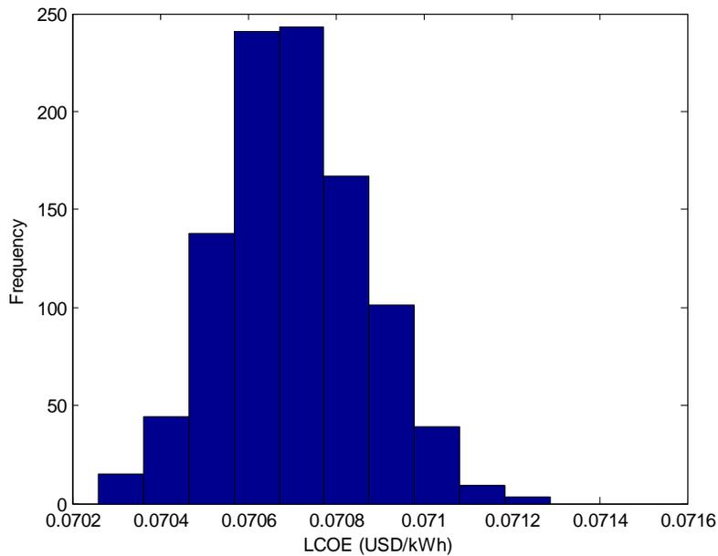
Figure 5.17 Distribution of LCOE for stepwise installation of solar PV plant at METU NCC with constant electricity prices
