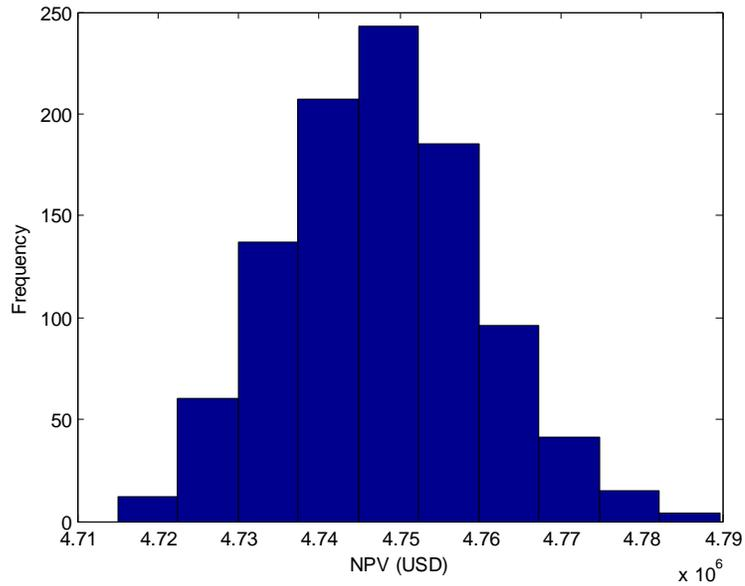
Figure 5.6 NPV distribution for 1 MW solar PV power plant at METU NCC for increasing electricity prices at 12 % annual rate
