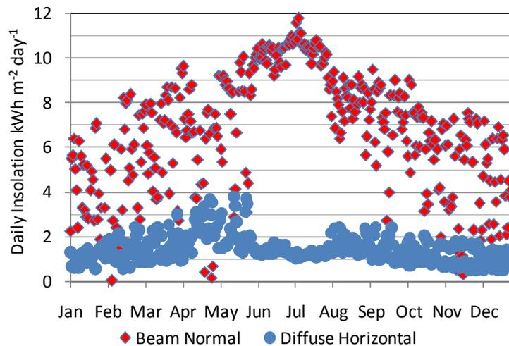
Figure 3.2 Daily beam (direct) normal and diffuse horizontal insolation for METU NCC
