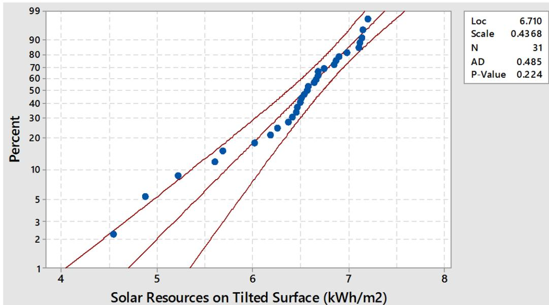
Figure D.7 Fitted Extreme Value distribution for solar resources on tilted surface for October
