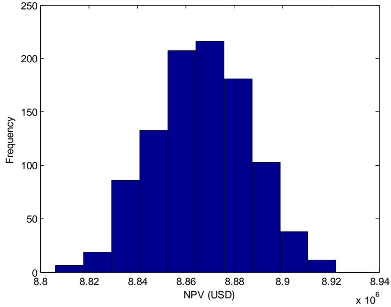
Figure 5.22 Distribution of NPV for stepwise installation of solar PV plant at METU NCC with increasing electricity prices at 12% annual rate
