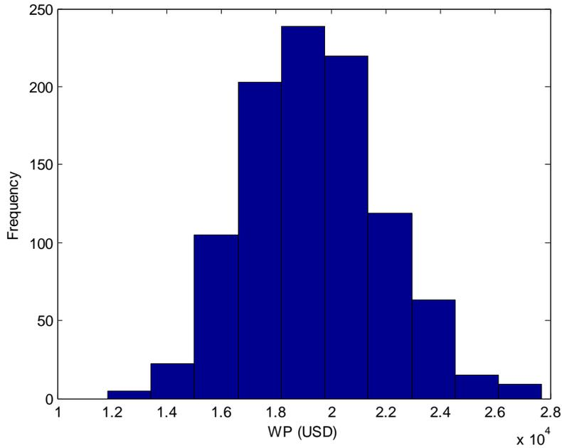
Figure 5.4 Distribution of WP for 1 MW solar PV plant at METU NCC with constant electricity prices
