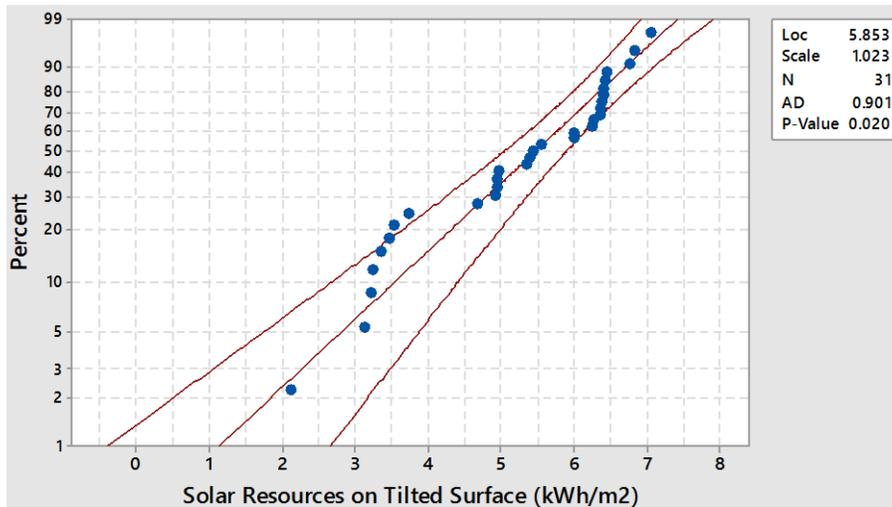
Figure 3.5 Fitted Normal distribution for solar resources on tilted surface for March
