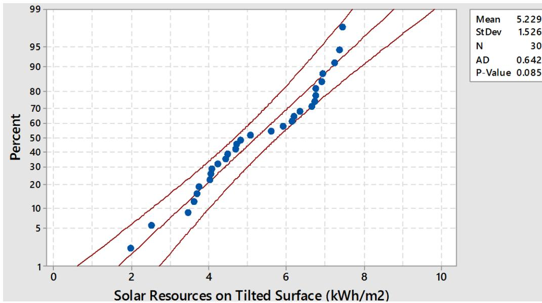
Figure D.1 Fitted Normal distribution for solar resources on tilted surface for April
