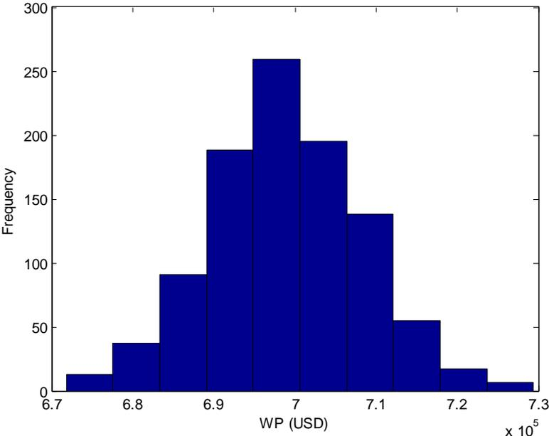
Figure 5.24 Distribution of cost of excess production for stepwise installation of solar PV plant at METU NCC with increasing electricity prices at 12% annual rate
