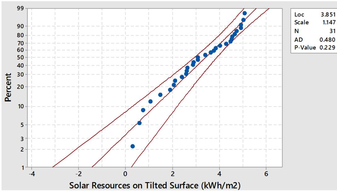
Figure D.9 Fitted Extreme Value distribution for solar resources on tilted surface for December
