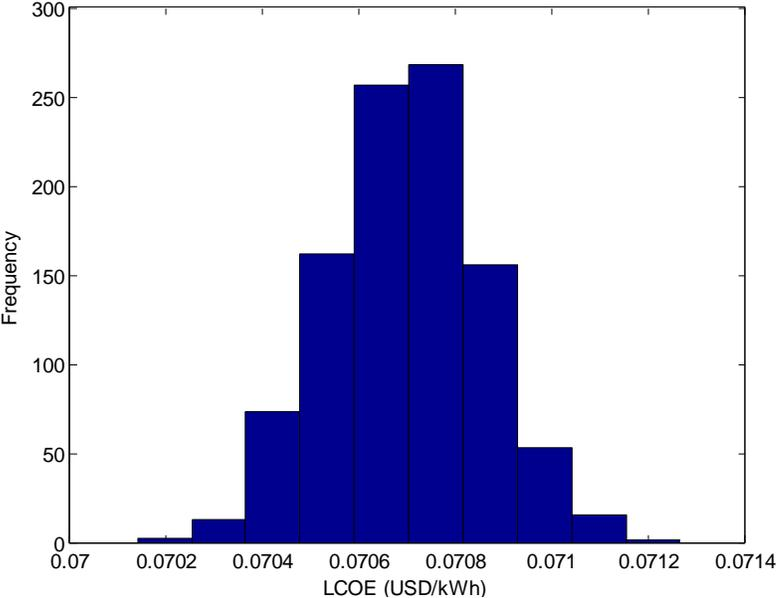
Figure 5.21 Distribution of LCOE for stepwise installation of solar PV plant at METU NCC with increasing electricity prices at 12% annual rate
