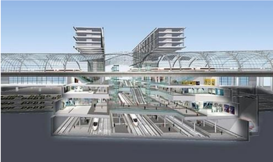
Figure 3.6 Berlin New Central Station Section: Daylight penetrate from all levels (Source DB Lehrter Bahnhof Report, 2005)
