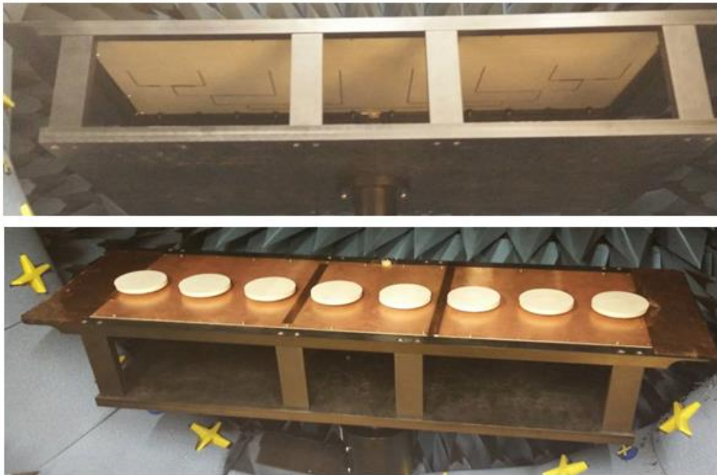
Fig. 84 Array support structure
