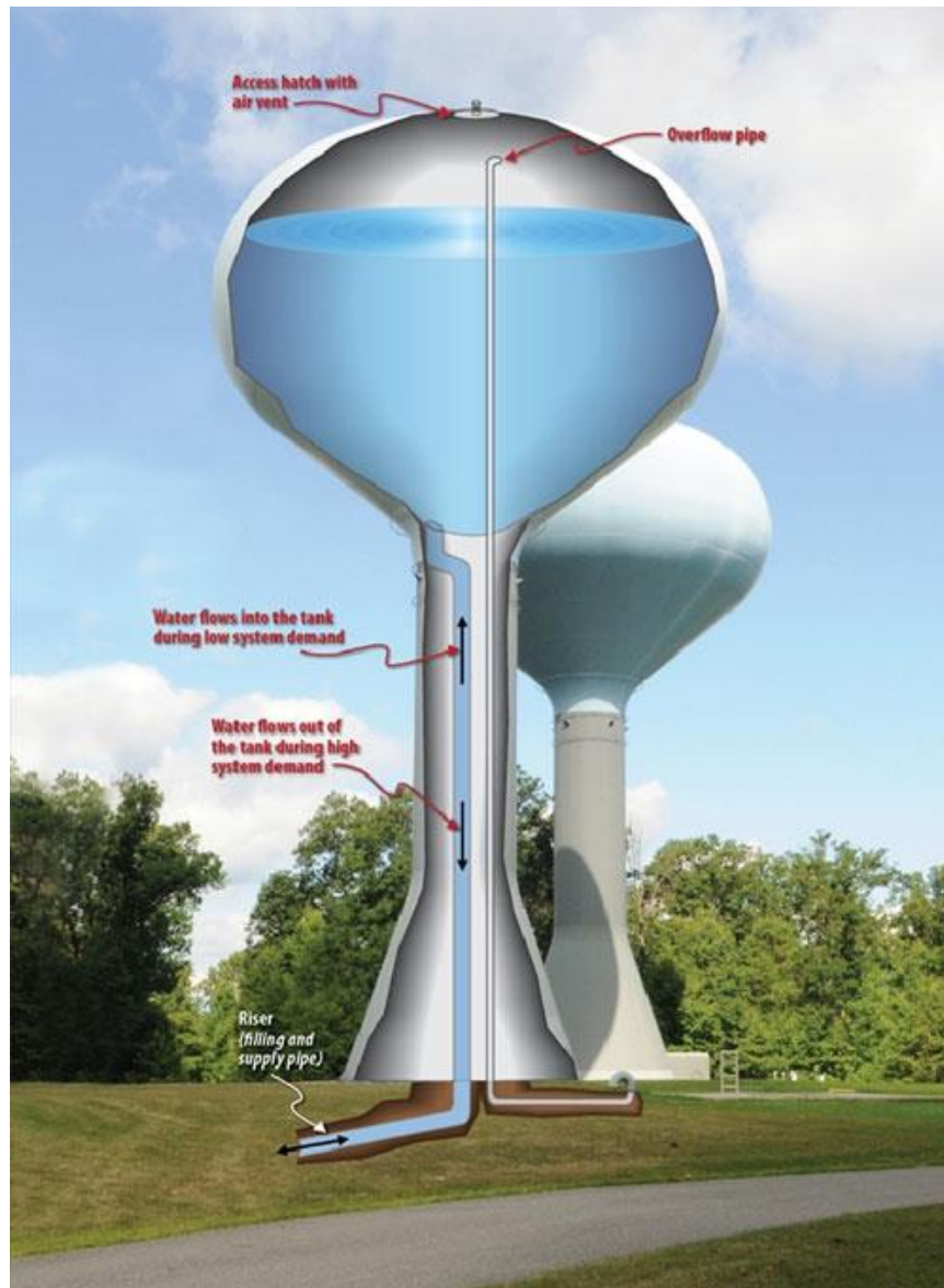
Figure 2.2. Elevated Water Storage Tank (WSSC, 2014)
