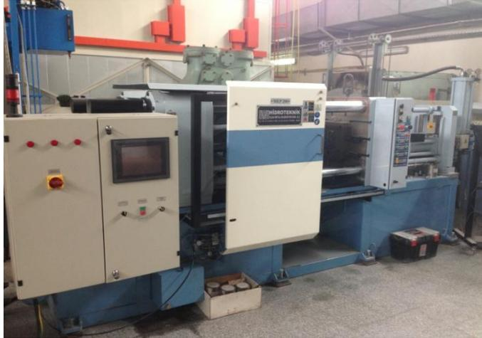
**Figure 29.** The high pressure die casting (HPDC) machine used in semi-solid metal casting.
