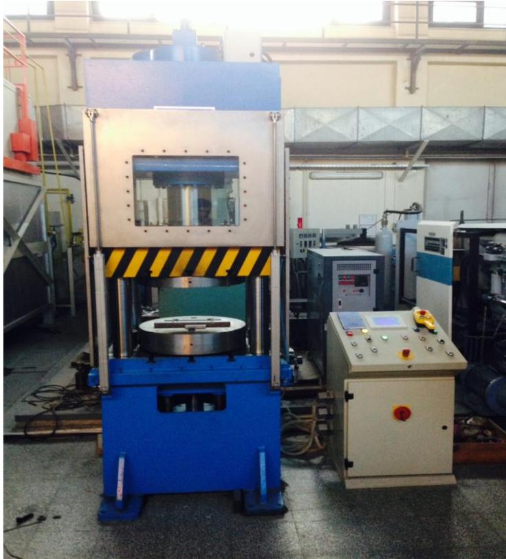
**Figure 16.** Vertical squeeze casting machine used in experiments.
