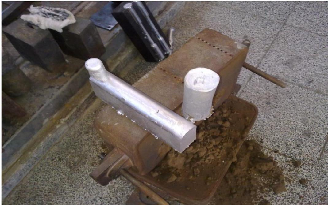
**Figure 23.** 7075 aluminum alloy casting after shake out of sand.
