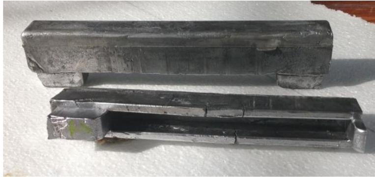
**Figure 28.** Produced hollow shaped parts after T6 heat treatment.
