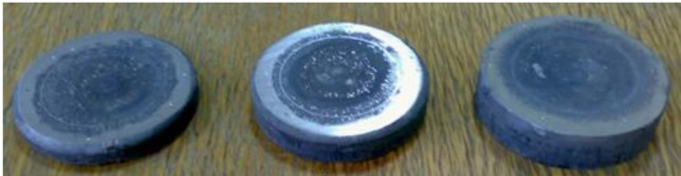
**Figure 17.** Squeeze cast 7075 alloy discs. First, second and third from left to right.
