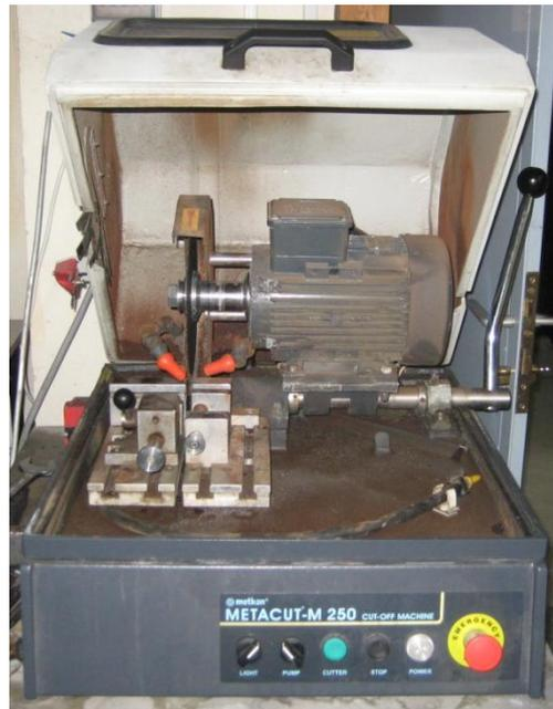
**Figure 40.** Metacut-M 250 Cut-Off Machine [51].
