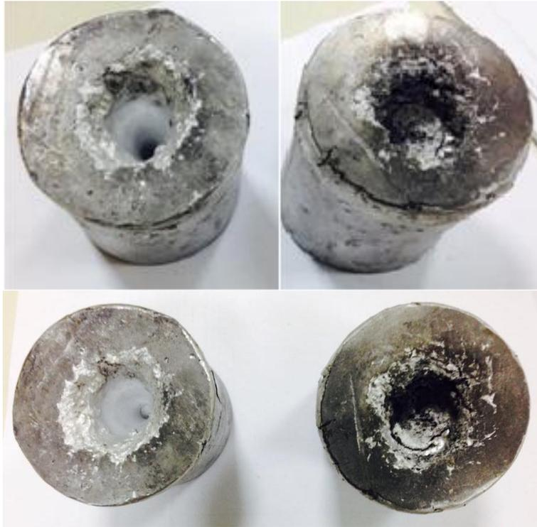
**Figure 31.** Cylindrical shaped alloy billets produced (left: ultrasonic stirring, right: mechanical stirring).
