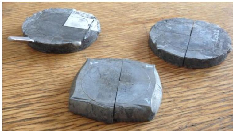
**Figure 26.** Produced disks after T6 heat treatment.
