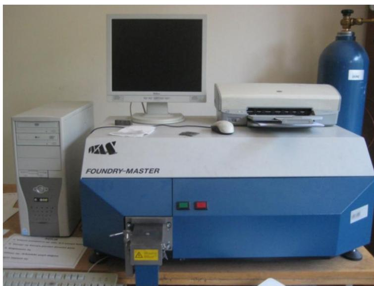
**Figure 42.** Foundry Master UV Vacuum CCD optical emission spectrometer.
