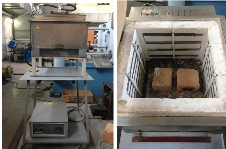
**Figure 19.** Muffle furnace used for heat treatment in experiments.
