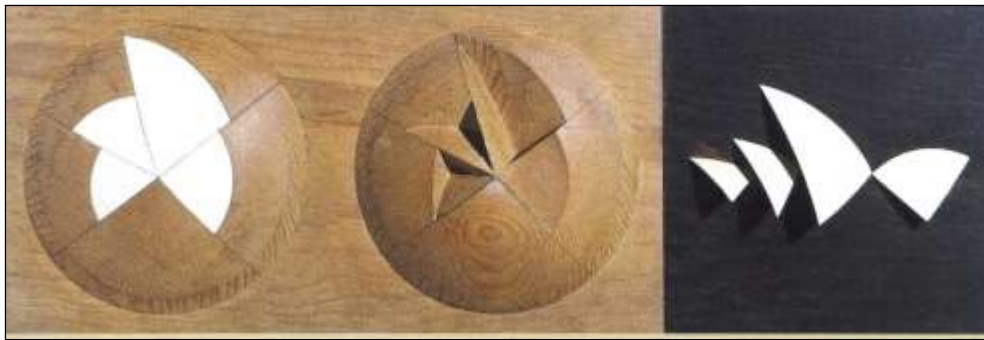
Figure 2.3: Wooden Concept model of Sydney Opera House by Danish architect Jørn Utzon, 1958. This model represents the geometrical solution for the pre-cast concrete shells. (Dunn, N. 2010)
