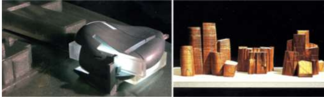
Figure 2.4: (left picture) Morphosis Experimental media and performing Arts centre, 2002-03. 3D printed resin. (Right picture) Gehry Partners, Düsseldorf's Media Harbour. 1996. CNC milled design-process, layered paper and resin. (Moon, k. 2005)
