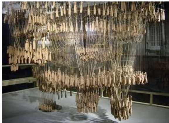
Figure 2.1: Antonio Gaudi, reproduced model of “La Sagrada Família”, 1983-1926. Up side down structural analysis made from strings and weighted sacks. (Source: https://www.flickr.com/photos/tillnm/3209875667/in/photostream/ )
