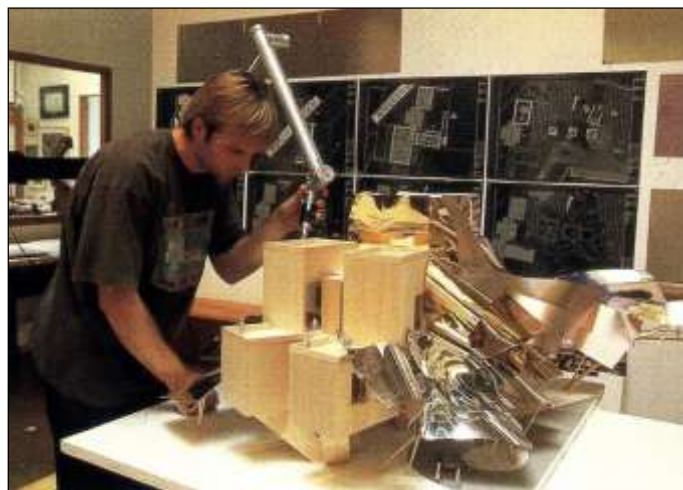
Figure 2.5: Final design model for Marques de Riscal Winery, 2000 Spain, being digitized by a Gehry partners. (Moon, k. 2005)
