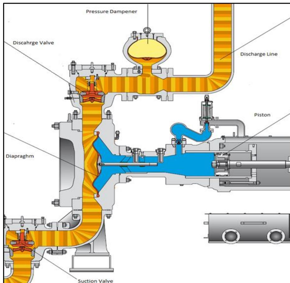
Figure 2.4 Single-Stage Positive Displacement Diaphragm Pump in Mine Dewatering
