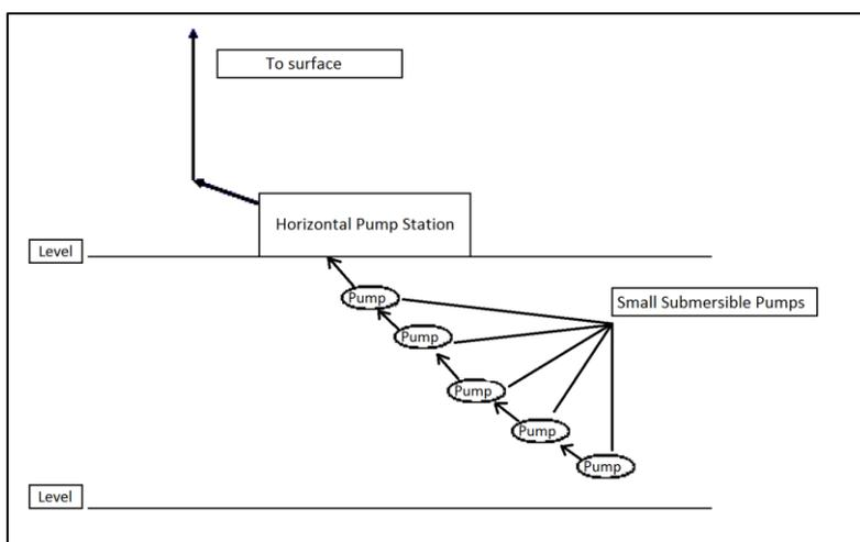
Figure 2.2 Underground Mine Dewatering
