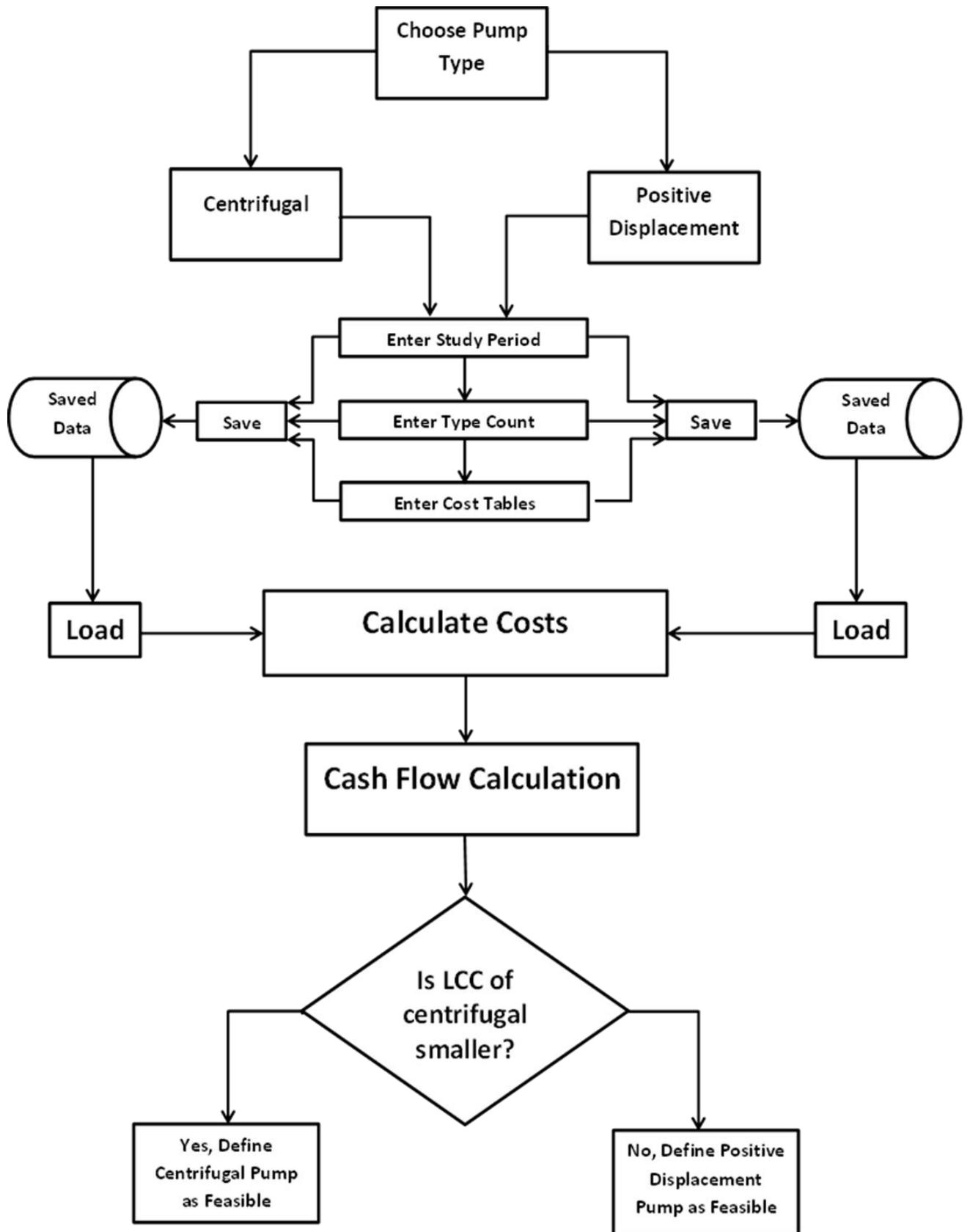
Figure 3.1 Flow chart algorithm of program
