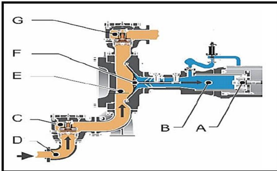
Figure 2.8 Suction Position of Positive Displacement Pump (Weir Minerals, 2012)
