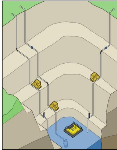
Figure 2.1 Schematic Diagram of Open Pit Mine Dewatering operation (Weir Minerals, 2015)
