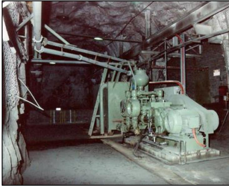
Figure 2.5 Dewatering with positive displacement pump (Weir Minerals, 1996)
