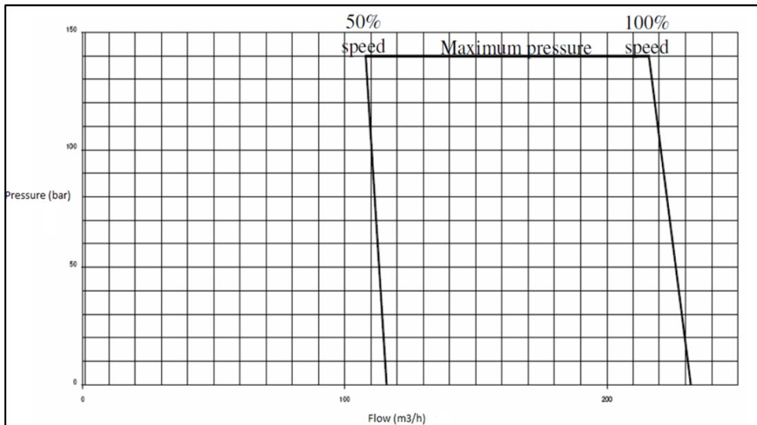
Figure 2.11 Positive Displacement Pump Curve (Kuenen, 2010)
