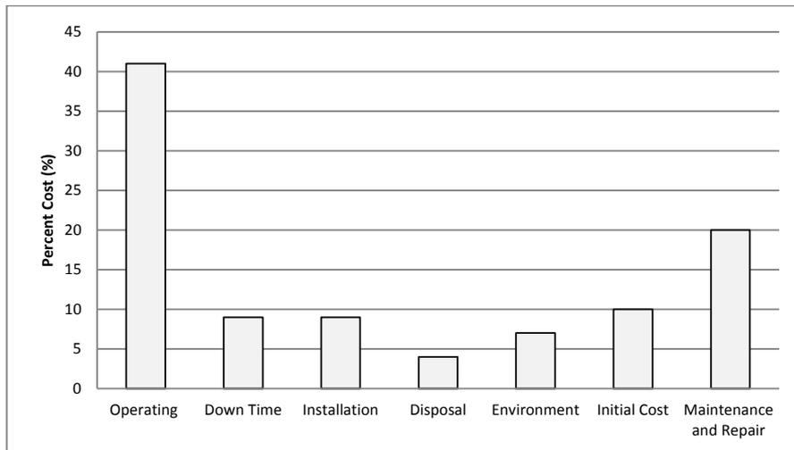
Figure 2.13 Life Cycle Cost Structure of a Pump (Kernan, 2013)
