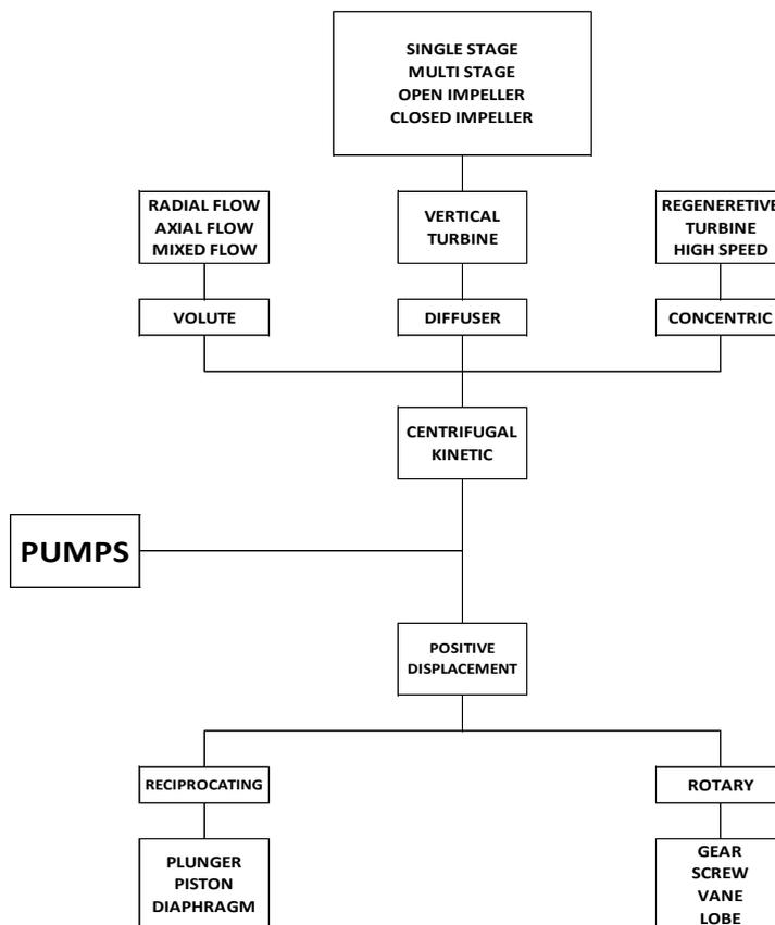
Figure 2.10 General Pump Classification (Modified after Bachus and Custodio, 2003)
