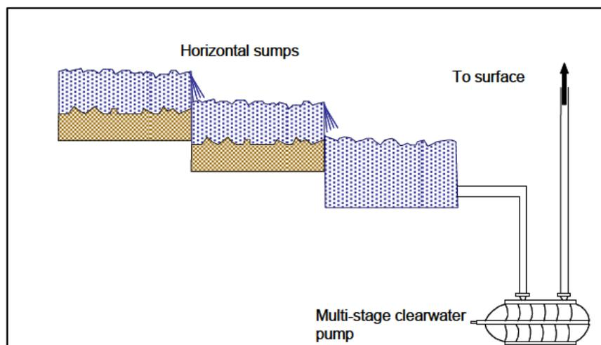
Figure 2.3 Centrifugal Pumps in Mine Dewatering (Weir Minerals, 2015)
