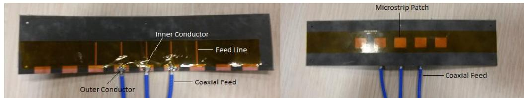
Figure 4-3 Produced aperture coupled patch antenna array
