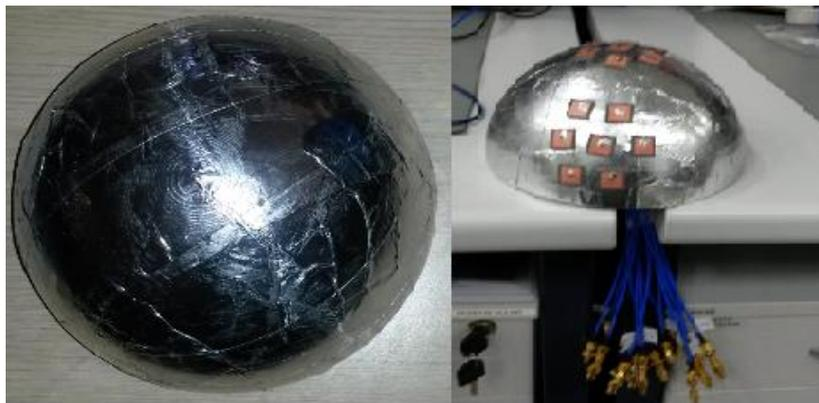
Figure 6-2 Produced spherical antenna array
