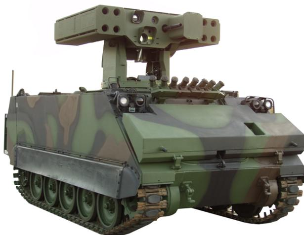
Figure 1.2: Another example of a motion platform: Pedestal Mount Stinger Launching System - PMS ATILGAN<sup>®</sup>.(In this system the payload is eight land-to-air missiles and optics to detect and track possible threats.(Photo Courtesy of Aselsan Inc.)
