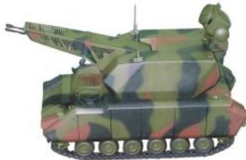
Figure 1.4: In the KORKUT air defense system developed by Aselsan Inc. there are independent motion platforms on the same system (one for optics / RADARs and other for the gun) (Photo Courtesy of Aselsan Inc.)
