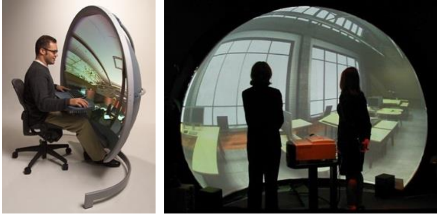
Figure 25 Examples of VR domes. Left: the VisionStation of 1.5m in diameter, designed for single-user immersive viewing. (Retrieved in 2011, from: http://www.vrealities.com/visionstation.html ) Right: the VisionDome3, of 3m in diameter, for mid-size workgroups, small audiences, or larger single-user applications. (Retrieved in 2011, from http://www.vrealities.com/visiondome3.html ).
