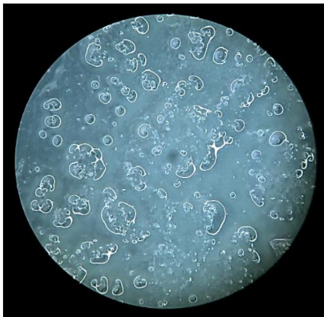
Figure 3. 4 Light reflection microscopy image of PULL microspheres with 10% (w/w) NaCl porogen (11.25 X magnification) after water leaching.
