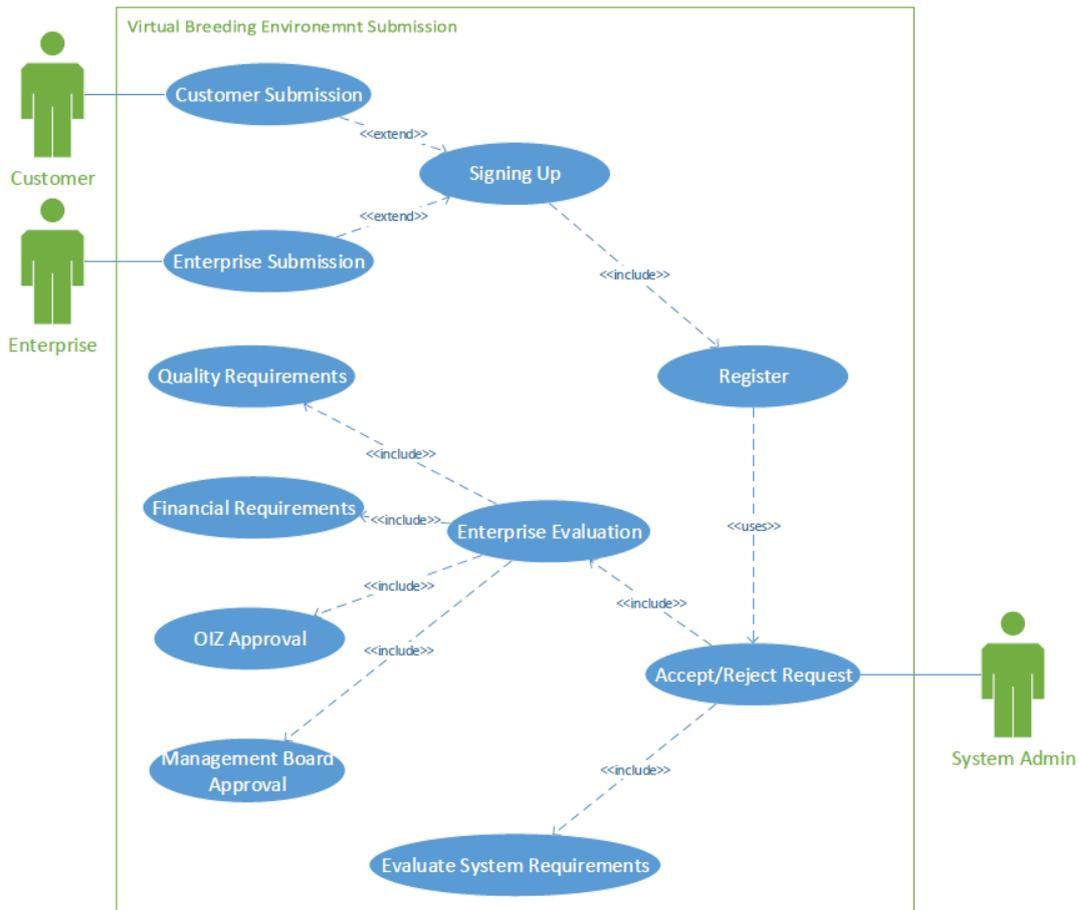
Figure 3.19: Virtual Breeding Environment Submission Use Case Diagram
