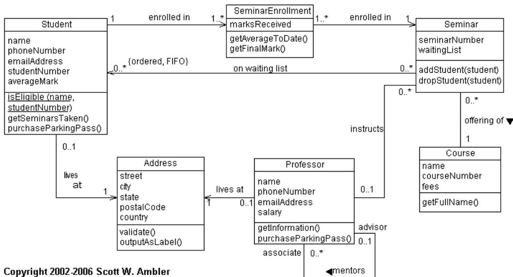
Figure 3.14: Sample Class Diagram [8]
