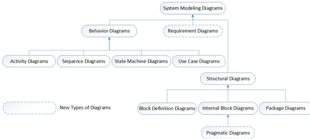
Figure 3.1: UML Diagrams Hierarchy [43]
