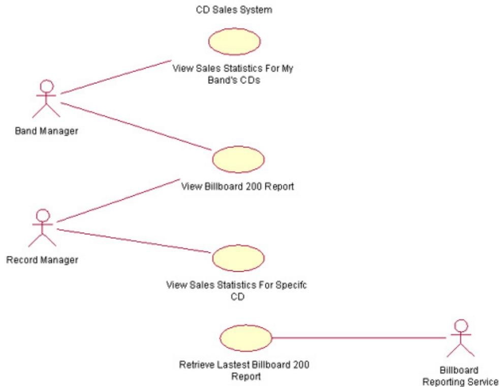
Figure 3.18: Use Case Diagram Sample [8]
