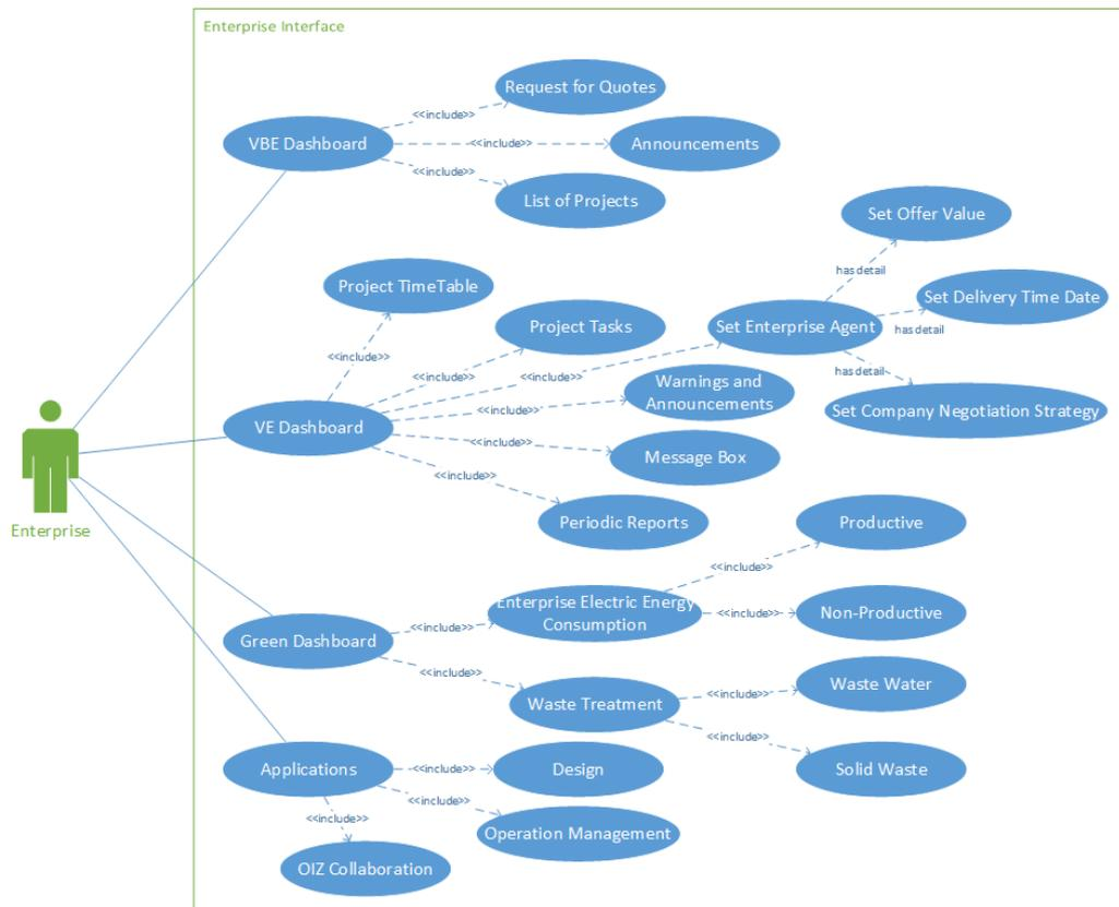
Figure 3.21: VE enterprises Use Case Diagram
