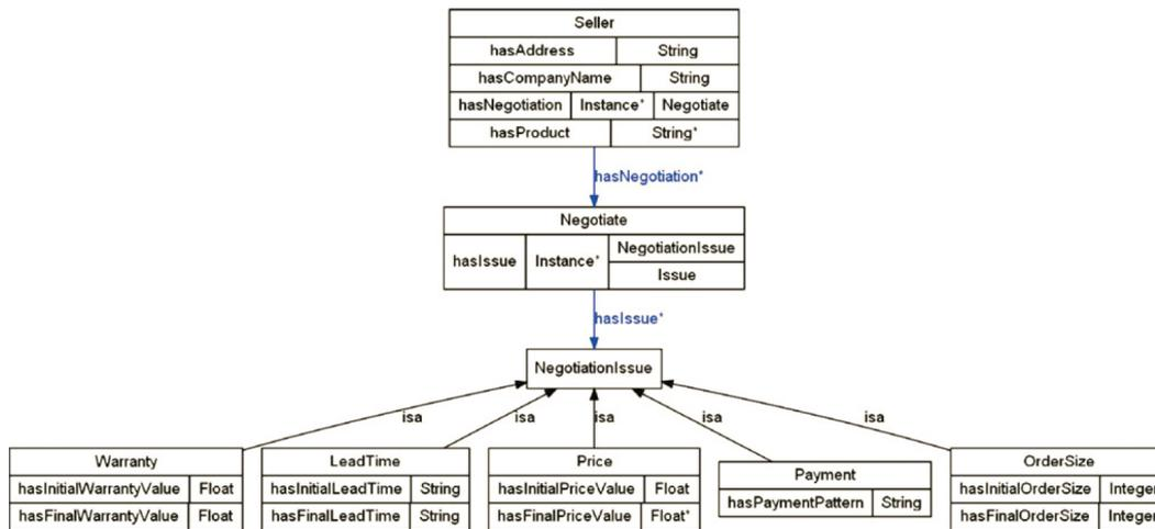
Figure 4.1: Ontology model for the Seller designed by Wang et al. [128]
