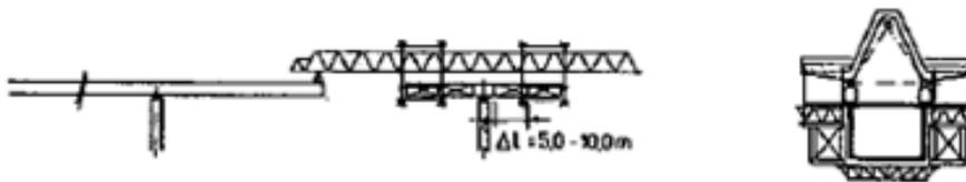
c) cantilever construction with launching gantry (Siegtal Bridge)
