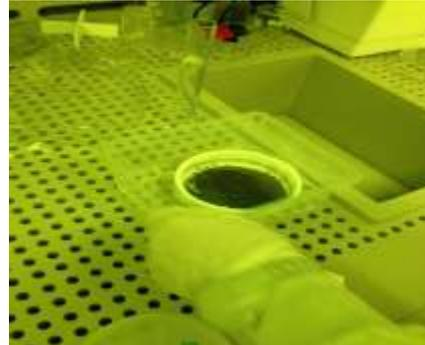
Figure 5.2 Cavity Patterned Wafer during developing
