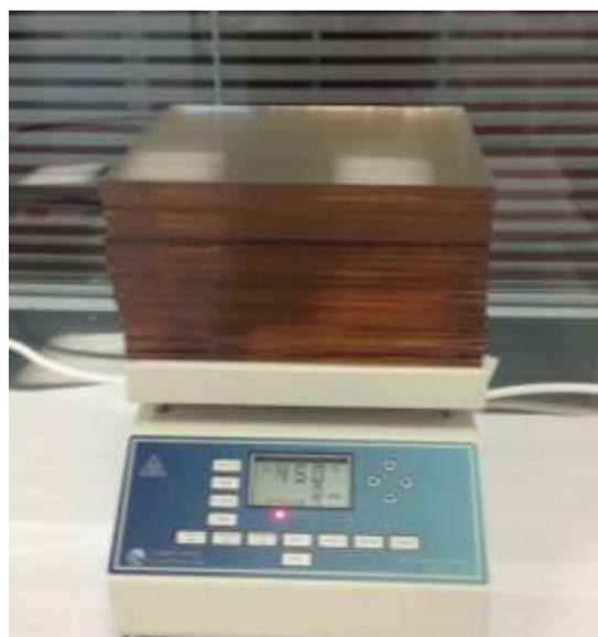
Figure 5.8 Wafer bonding annealing system
