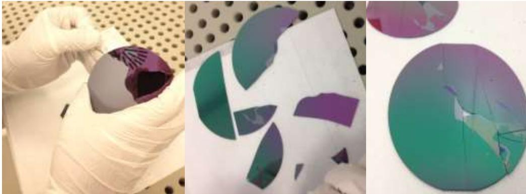
Figure 5.9 Wafer Bonding Results
