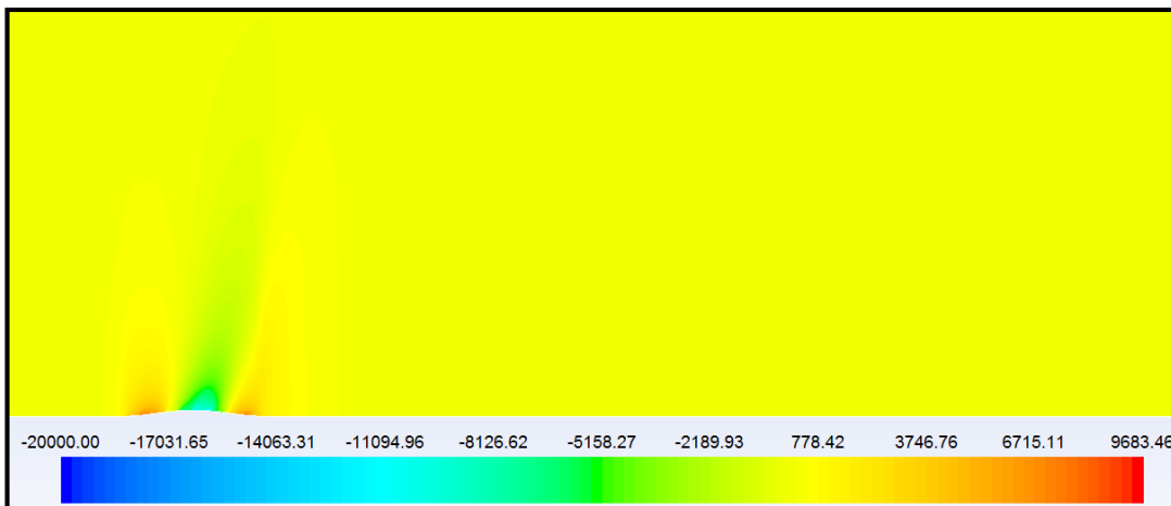
Figure 15-S-H Slender Body Static Pressure Contours at Mach=1 [Pa]
