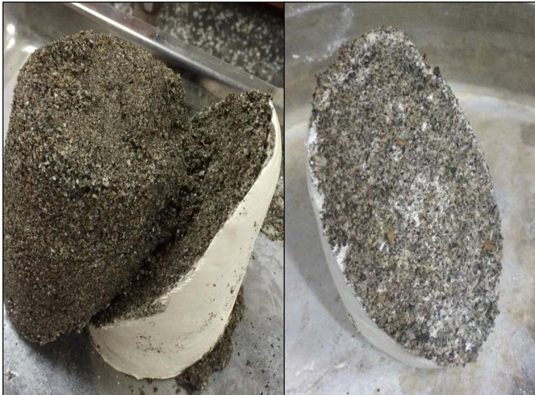
Figure 4.31 Sand-Clay Interfaces after Triaxial Tests
