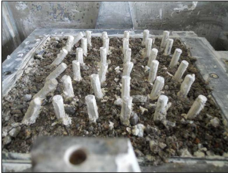
Figure 5.11 Improvement Tests with 36 Model Dowels-Dowel Length=6cm (I-6)
