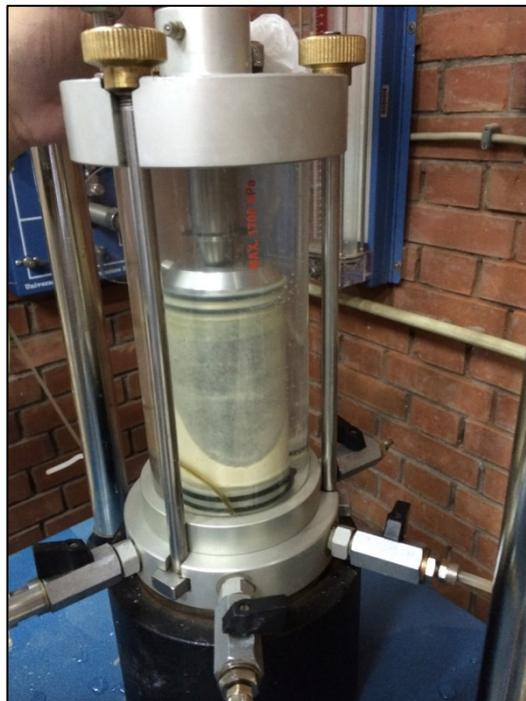
Figure 4.14 Triaxial Testing of Interfaces
