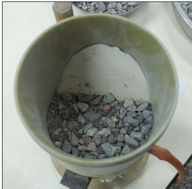
Figure 4.12 Filling Upper Part of Gravel-Clay Interface with Gravel
