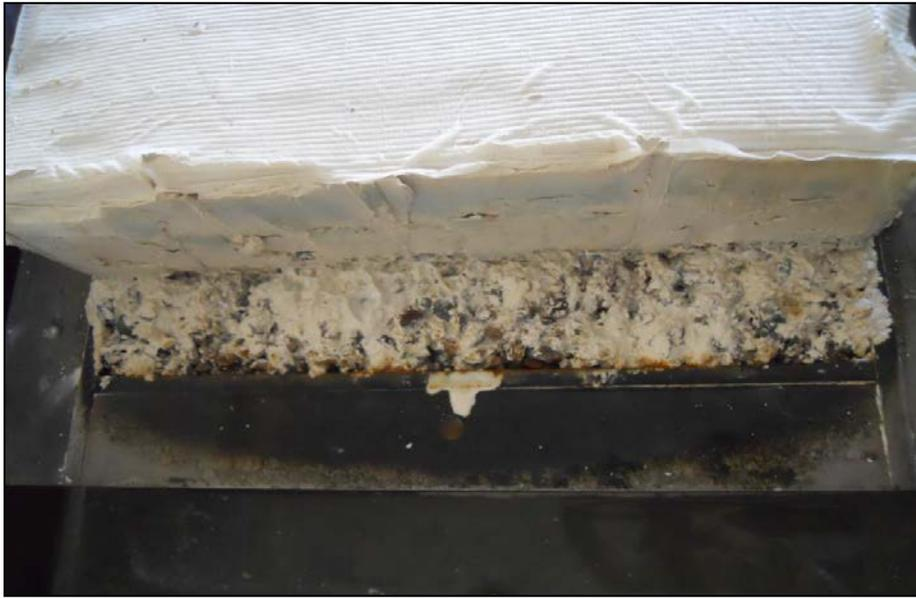
Figure 3.8 Large Shear Box Tests of Gravel-Clay Interface
