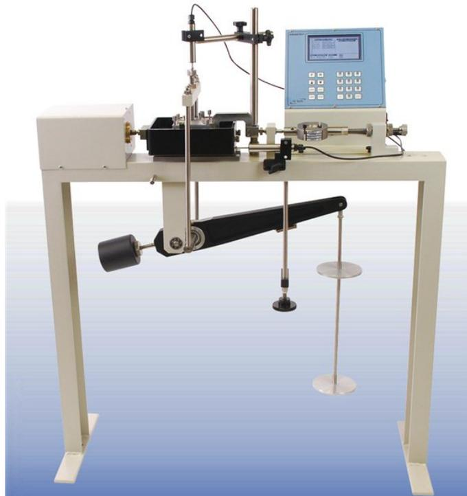
Figure 3.16 General View of Small Shear Box Machine
