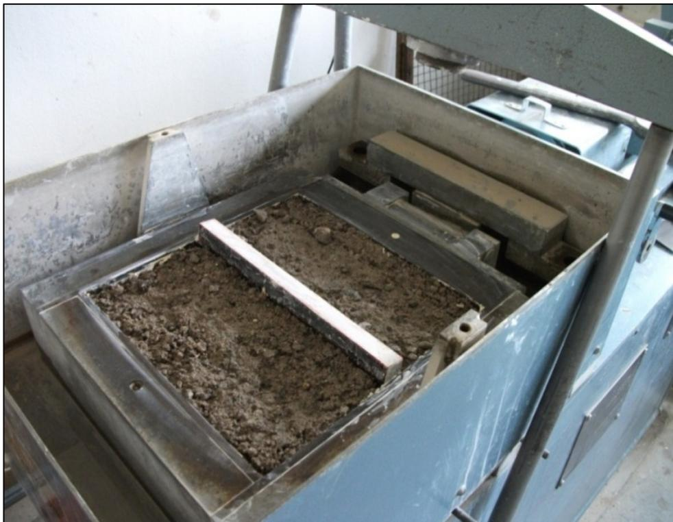
Figure 5.19 Improvement Tests with Continuous Wall
