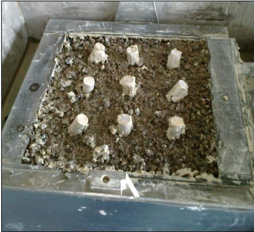
Figure 5.9 Improvement Tests with 9 Model Dowels-Dowel Length=4cm (I-4)
