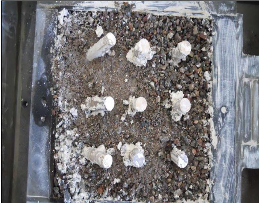
Figure 5.8 Improvement Tests with 9 Model Dowels-Dowel Length=8cm (I-3)
