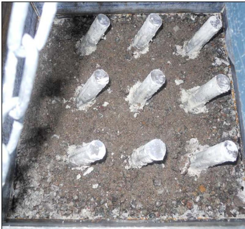
Figure 5.10 Improvement Tests with 9 Model Dowels-Dowel Length=12cm (I-5)
