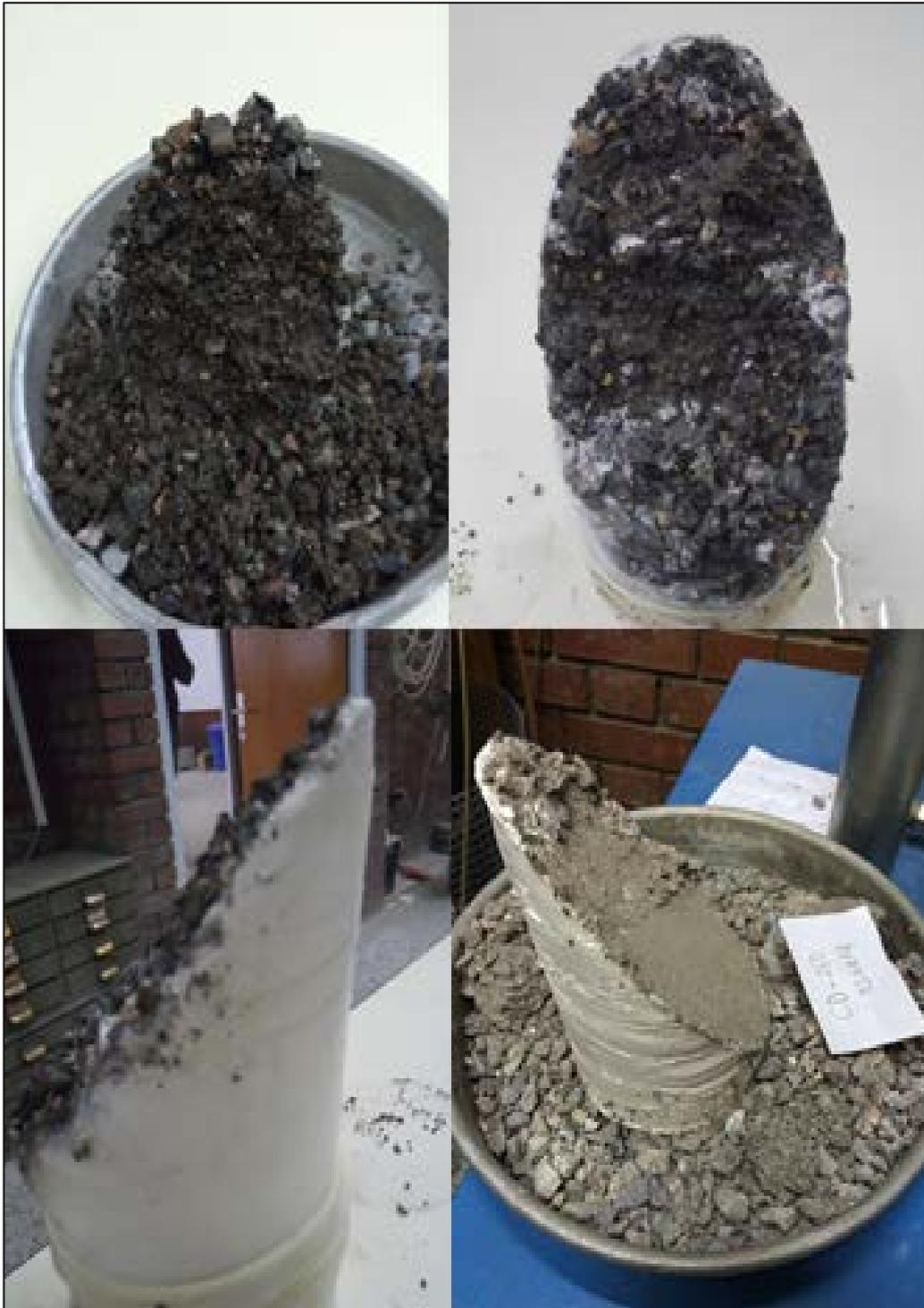
Figure 4.25 Gravel-Clay Interface Triaxial Tests-Shear Surface after Experiments
