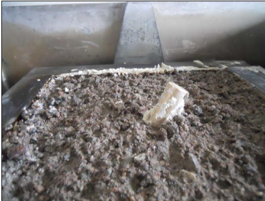
Figure 5.6 Improvement Tests with 1 Model Dowel-Dowel Length=8cm (I-1)
