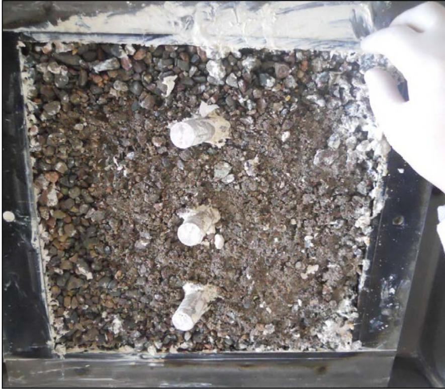
Figure 5.7 Improvement Tests with 3 Model Dowels-Dowel Length=8cm (I-2)
