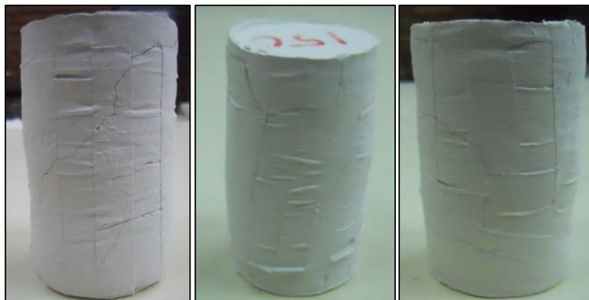
Figure 4.2 Clay Specimens after Triaxial Tests
