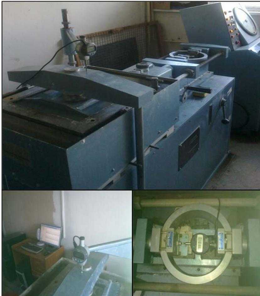
Figure 3.4 Instrumentation on Large Shear Box
