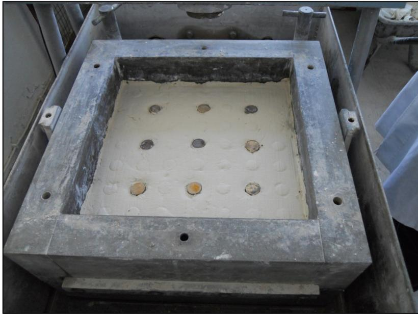
Figure 5.4 Dowels Placed to the Drilled Holes
