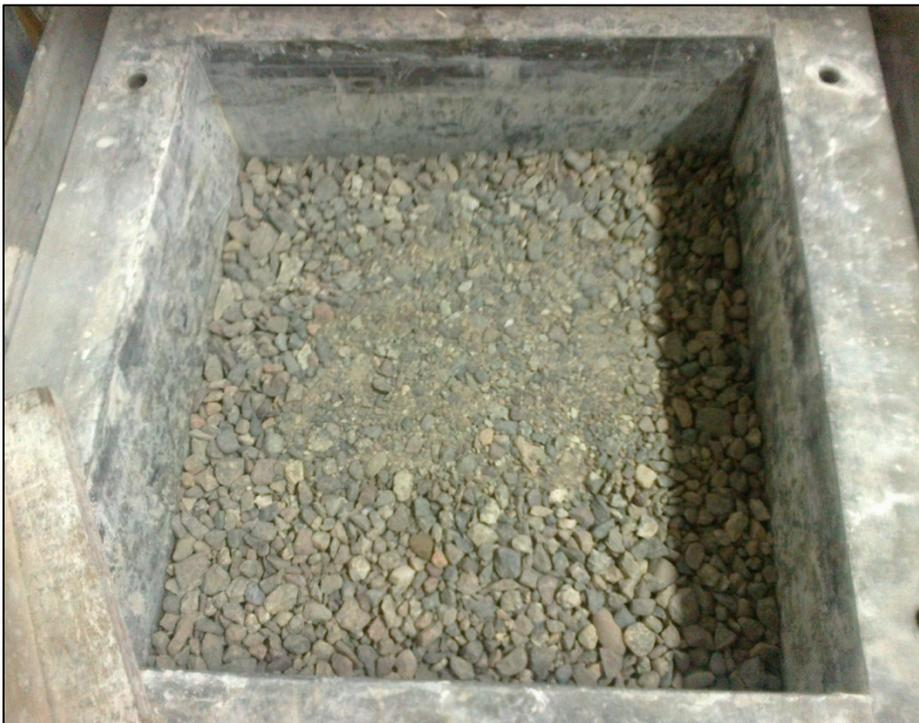
Figure 5.1 Gravel in the Lower Part of the Large Shear Box
