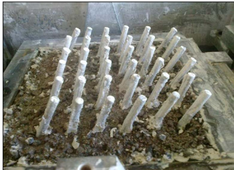
Figure 5.12 Improvement Tests with 36 Model Dowels-Dowel Length=12cm (I-7)
