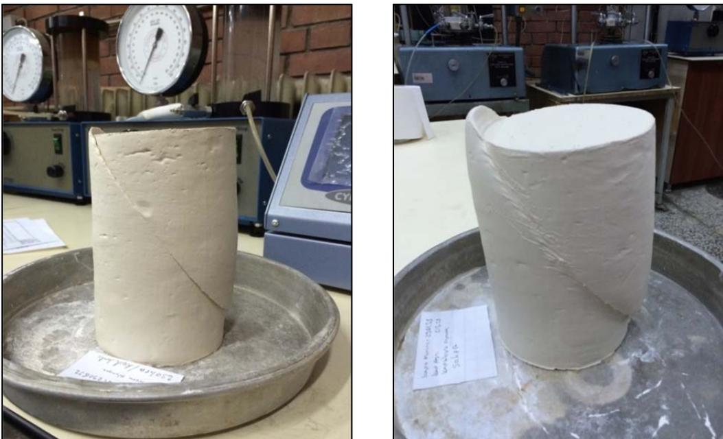
Figure 4.16 Clay-Clay Specimen after Triaxial Tests
