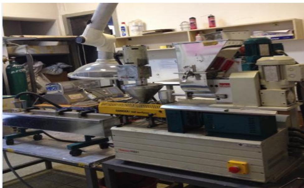
**Figure 3.8** Thermoprism TSE 16 TC twin screw extruder.
