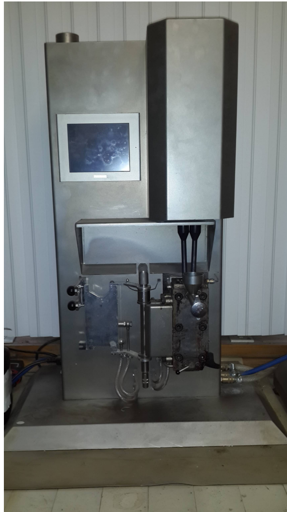
Figure 3. 3 The photograph of the twin screw extruder used for the composite production in this study
