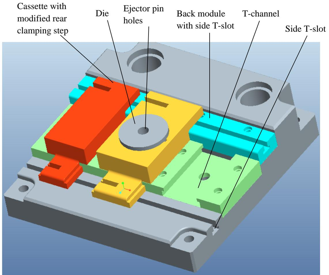
Figure 4.6 A view of the cassettes, cassette holder with T-channels, side T-slots and back support module (Version-3)
