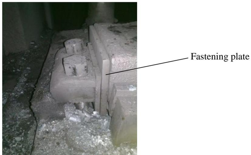
Figure 3.5 Use of fastening plates to fill the gap between shoes and cassettes
