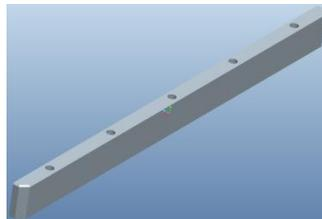
Figure 4.12 Side rail for guiding die holder on anvil adapter
