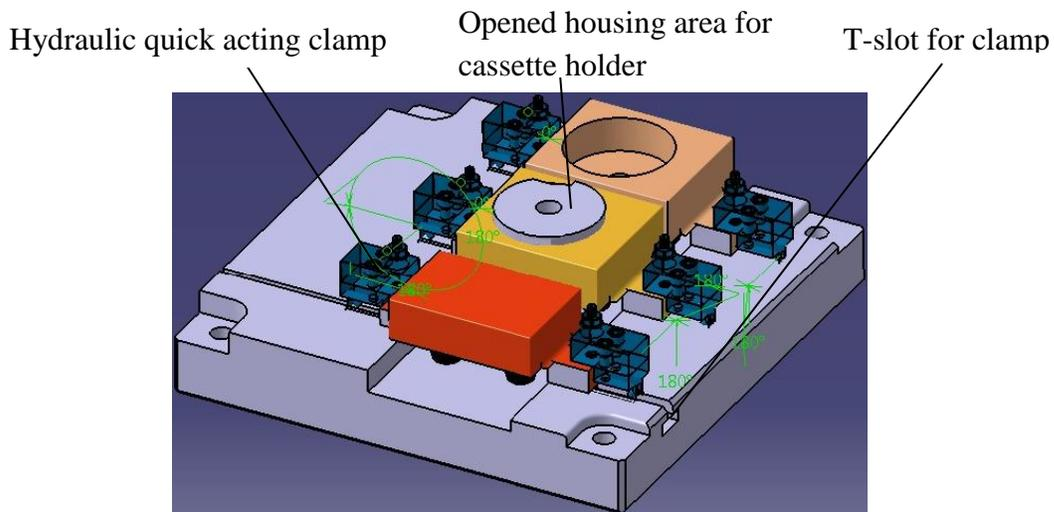
Figure 4.5 A view of the multiple quick acting hydraulic clamps used on the die holder (Version-3)
