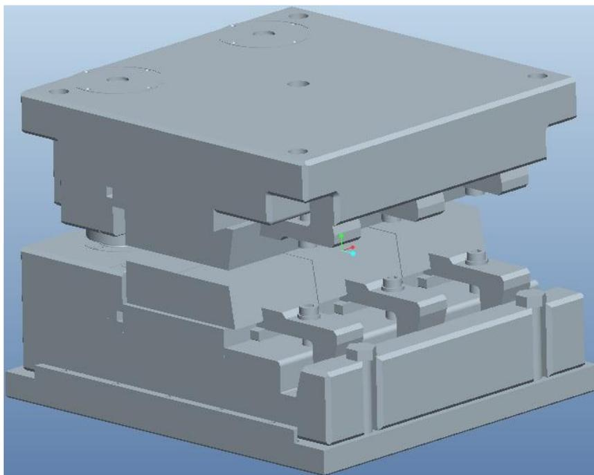
Figure 4.31 Solid model of the die holders complete assembly
