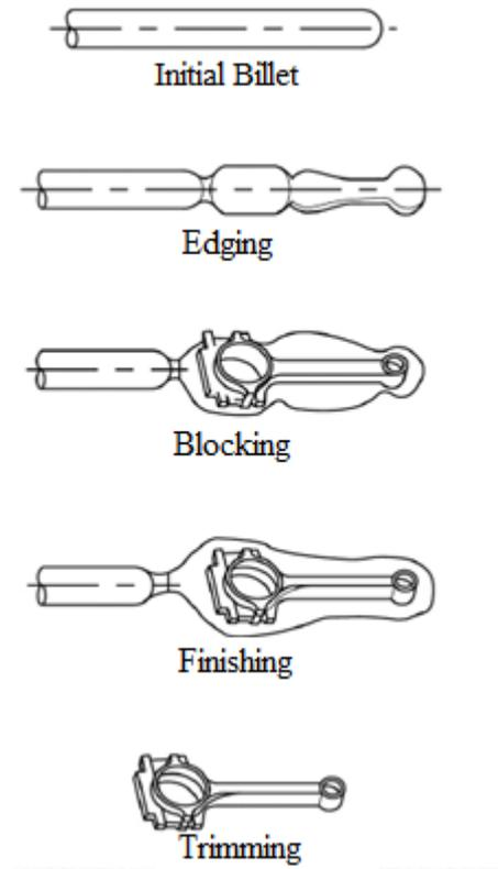
Figure 1.1 Stages in closed die forging of a connecting rod [1]
