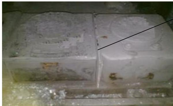
Sheet metal plates used for adjustment of cassettes
