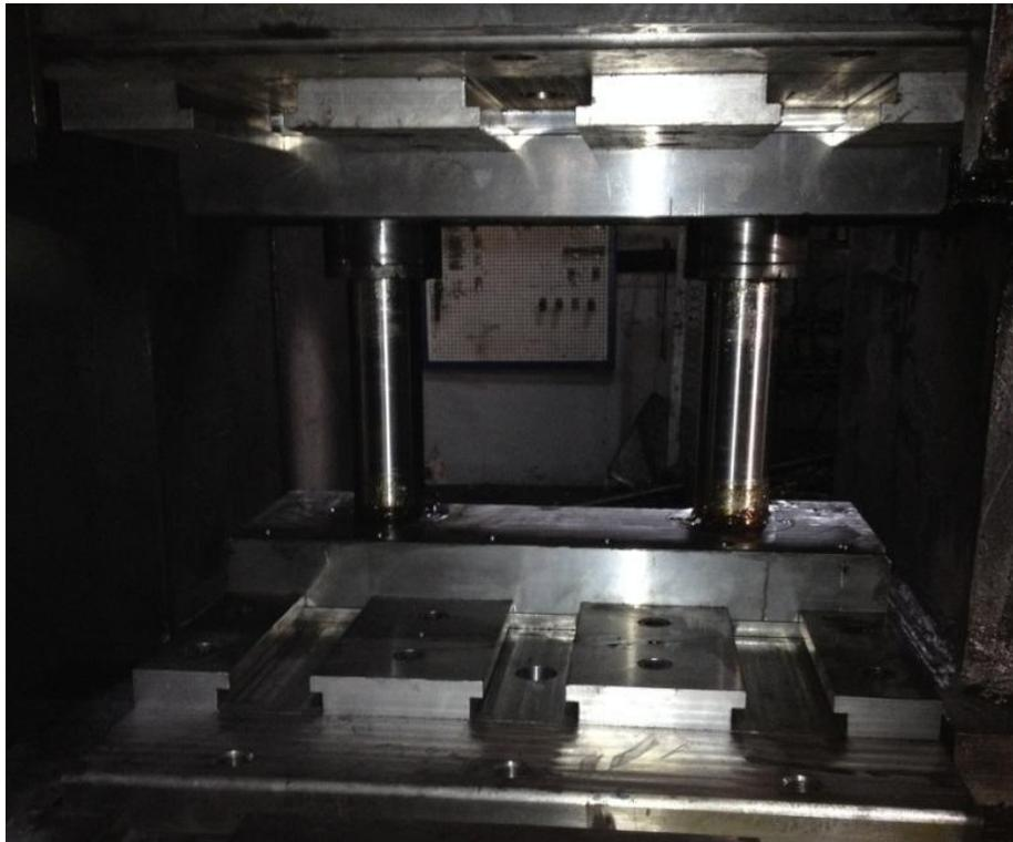
Figure 5.9 A view of the die holders assembled on the forging press
