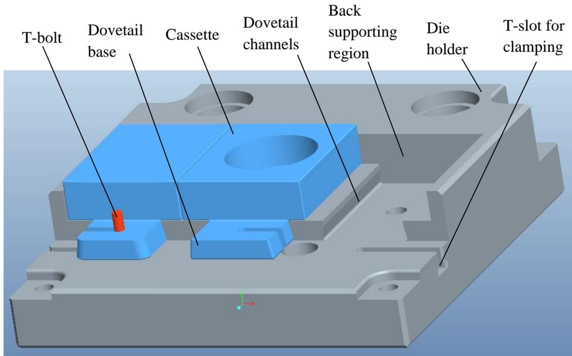
Figure 4.1 Die holder with dovetail form (Version-1)
