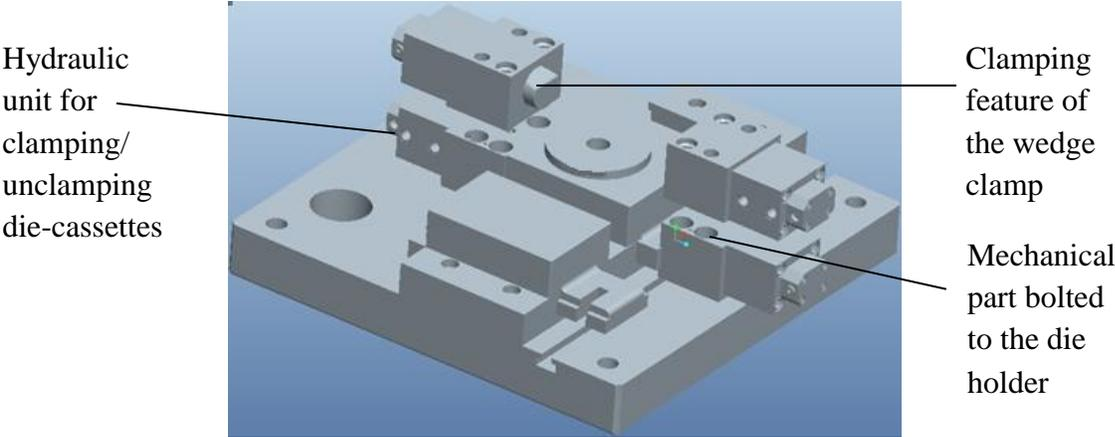
Figure 4.8 A view of the wedge clamps on the die holder
