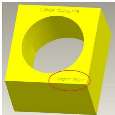
Figure 3.6 Marking for correct orientation of cassettes [11]
