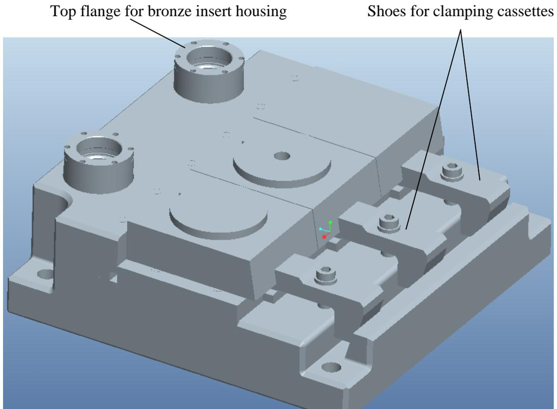
Figure 4.30 Solid model of the upper die holder assembly
