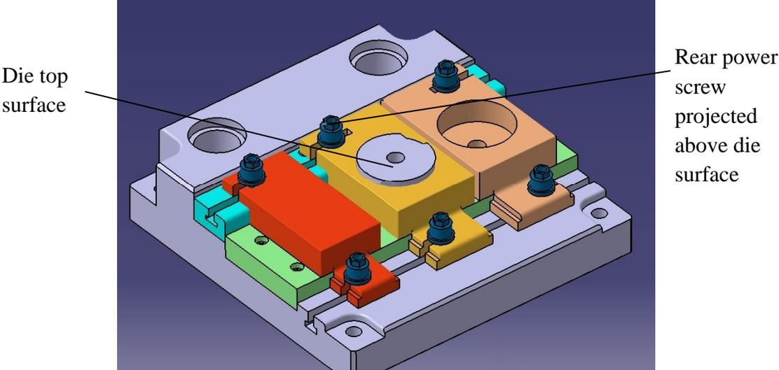
Figure 4.7 A view of the quick acting clamp (Power Screw) on the die holder
