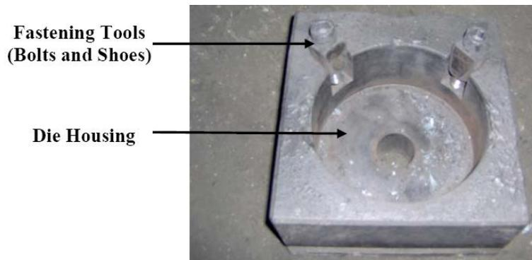
Figure 3.3 Conventional cassette design currently used for mounting the dies by using shoes and bolts in die housing [11]
