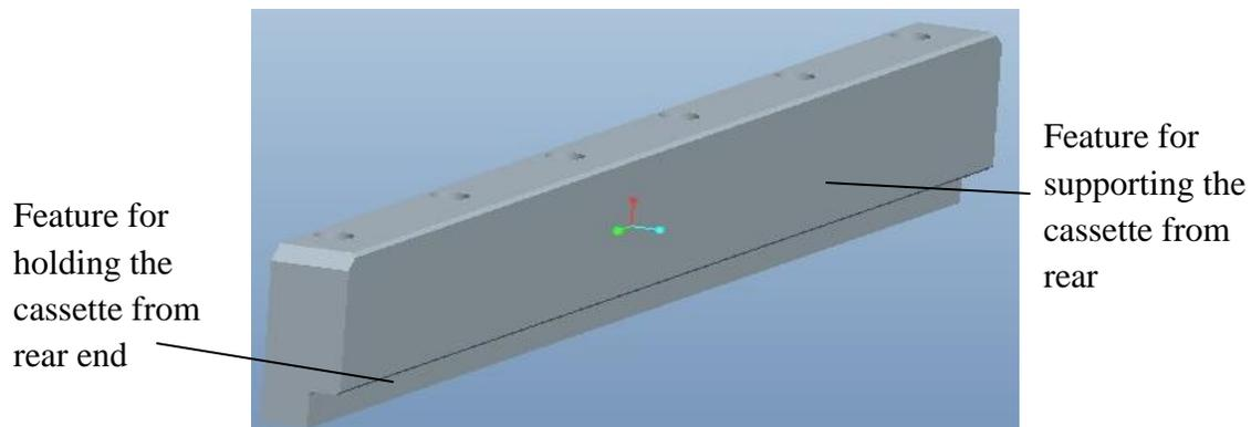
Figure 4.14 A view of the back support module
