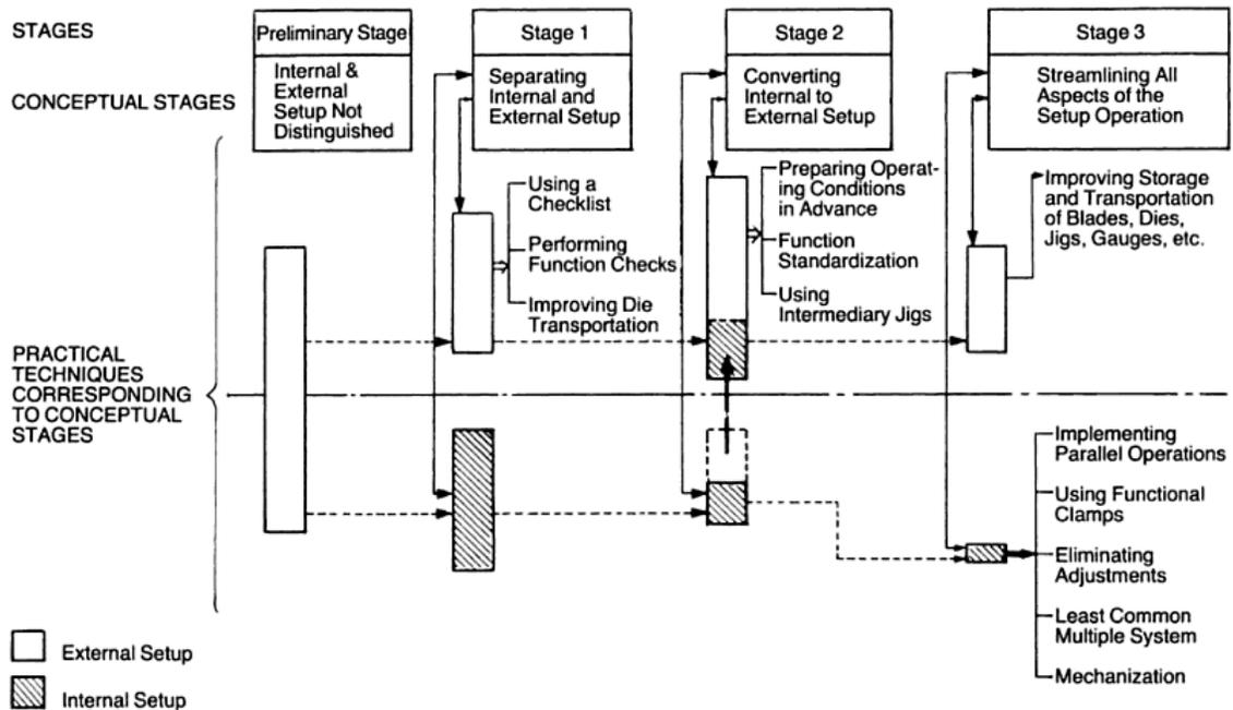
Figure 2.1 Single-Minute Setup (SMED): Conceptual Stage and Practical Techniques
