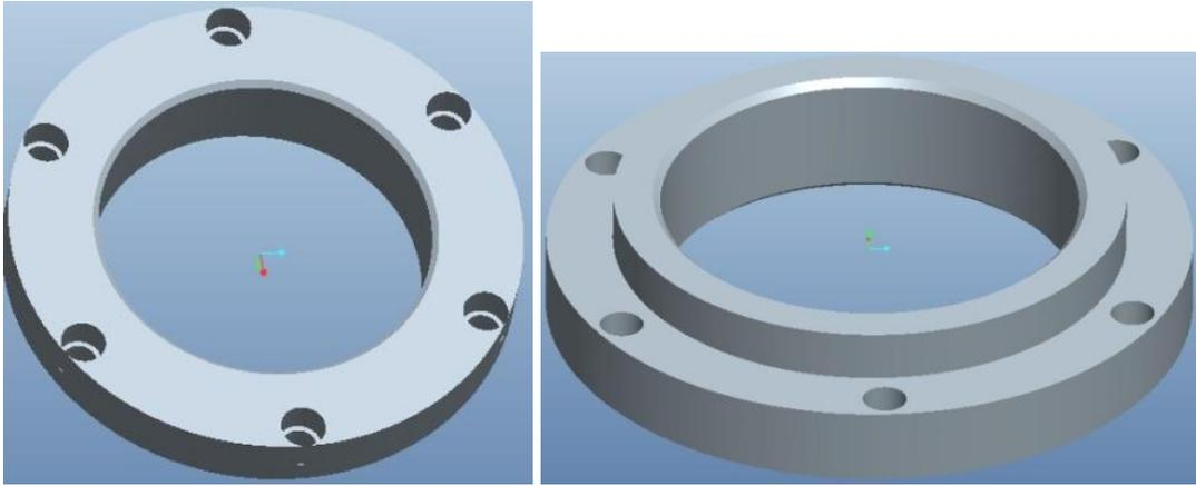
Figure 4.26 Top closing flange for bronze insert bushing
