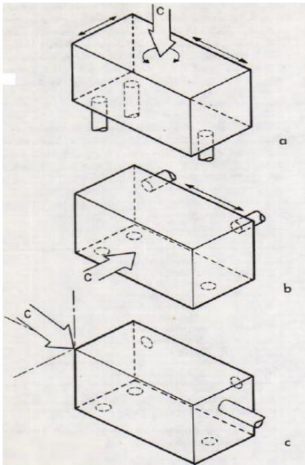
Figure 2.3 Principle of locating a part by 3-2-1 method [17]
