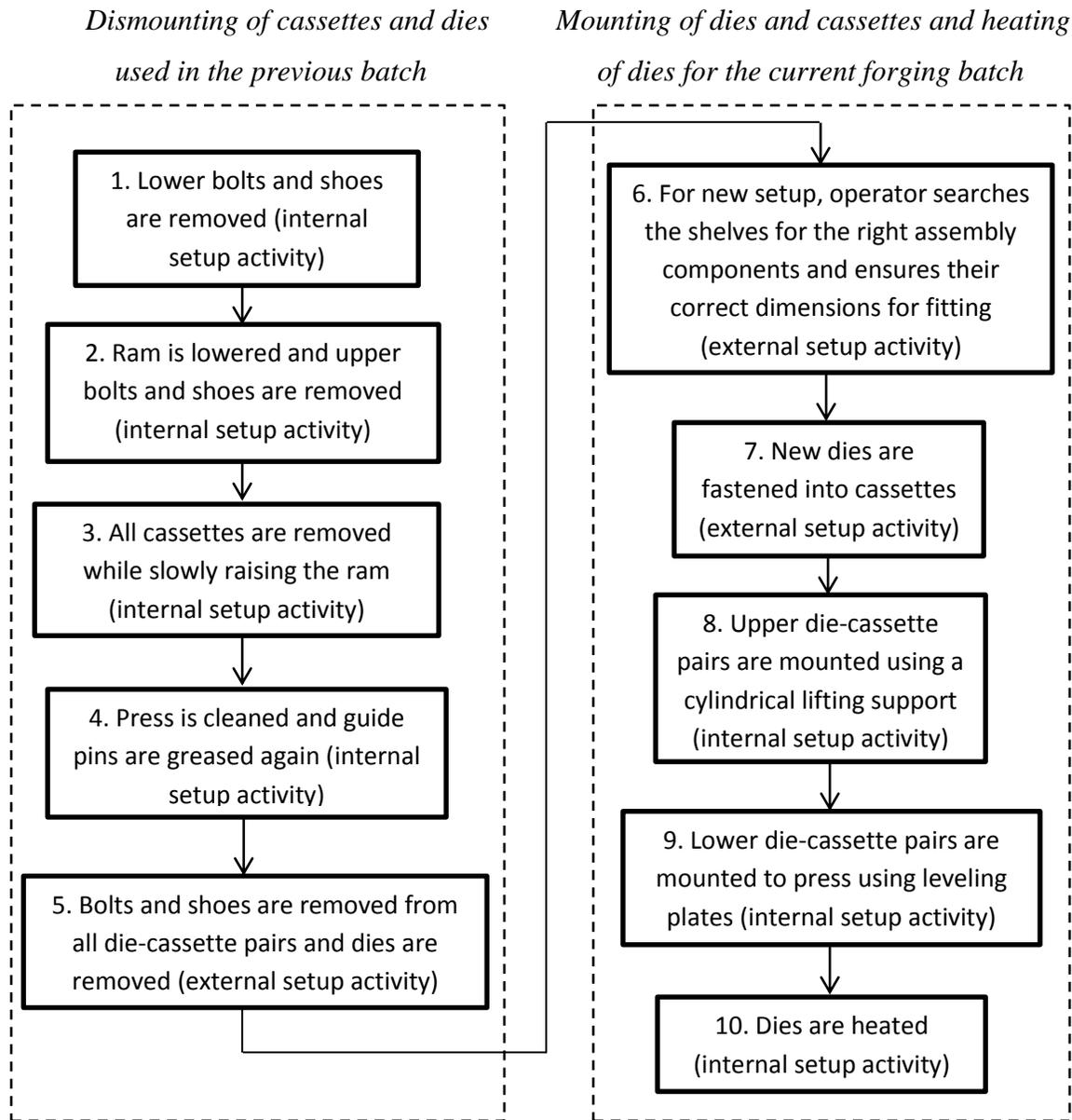
Figure 3.8 Sequence of setup change operations
