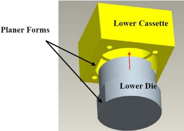
Figure 3.2 Planar forms suggested to eliminate rotational misalignment [11]
