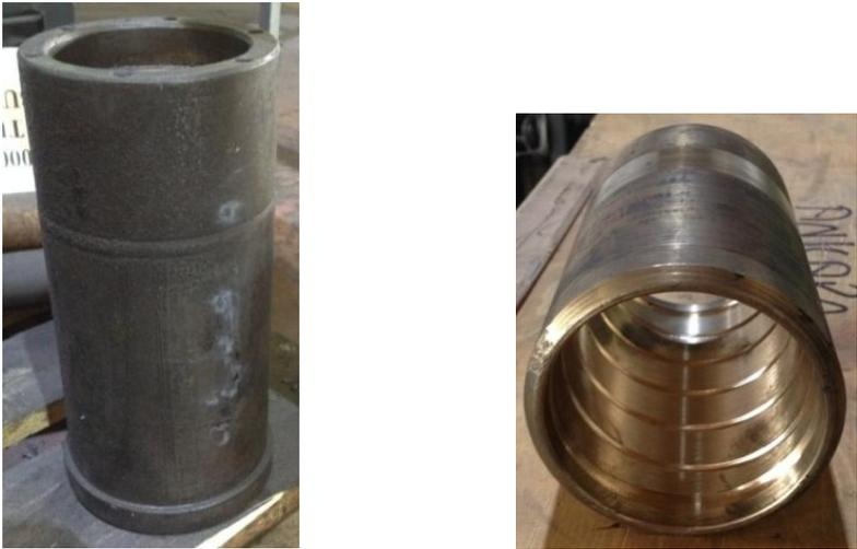
Figure 5.2 A view of the housing for bronze insert and the bronze insert
