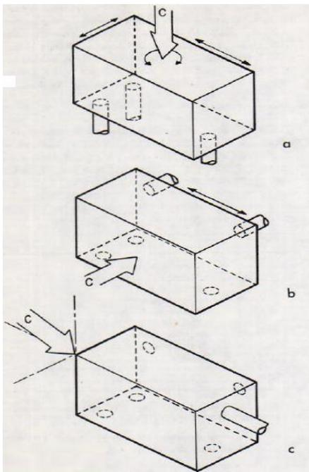
Figure 2.3 Principle of locating a part by 3-2-1 method [17]
