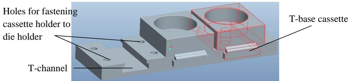
Figure 4.4 Cassette holder with T-channels (For Version-3)
