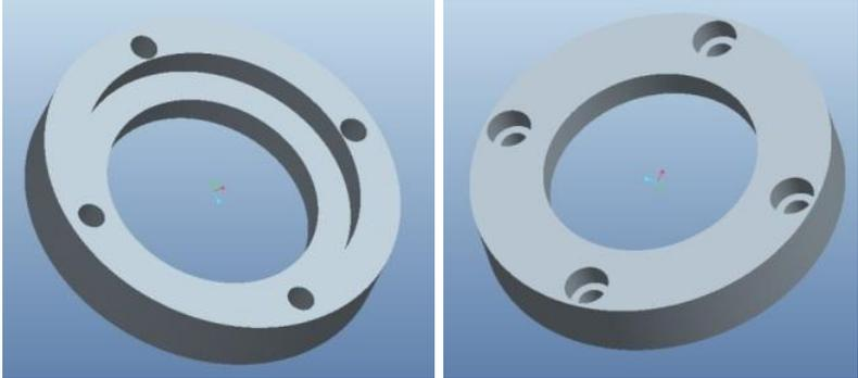
Figure 4.22 Top closing flange for guide pin bushing
