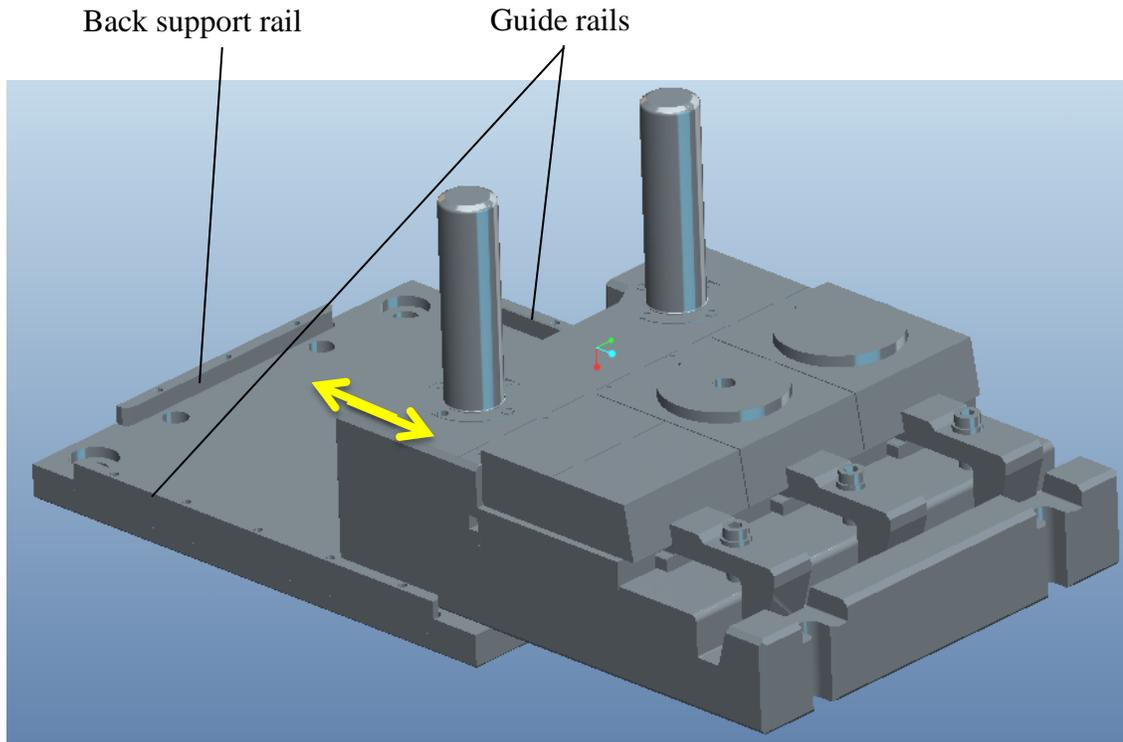
Figure 4.10 A view of the mounting or dismounting the die holder assembly from the anvil adapter
