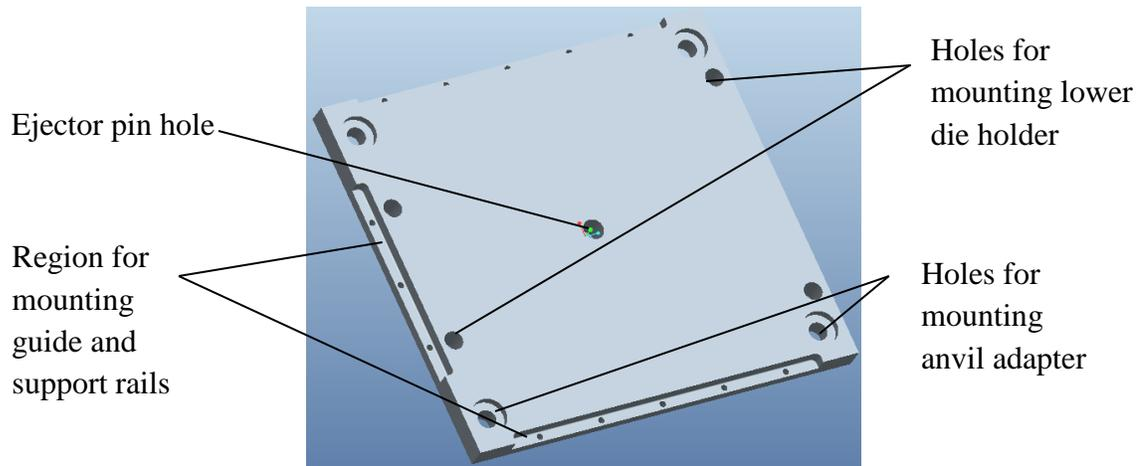
Figure 4.11 A view of the anvil adapter
