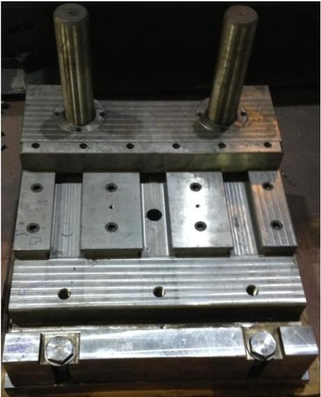
Figure 5.7 A view of the fully assembled lower die holder
