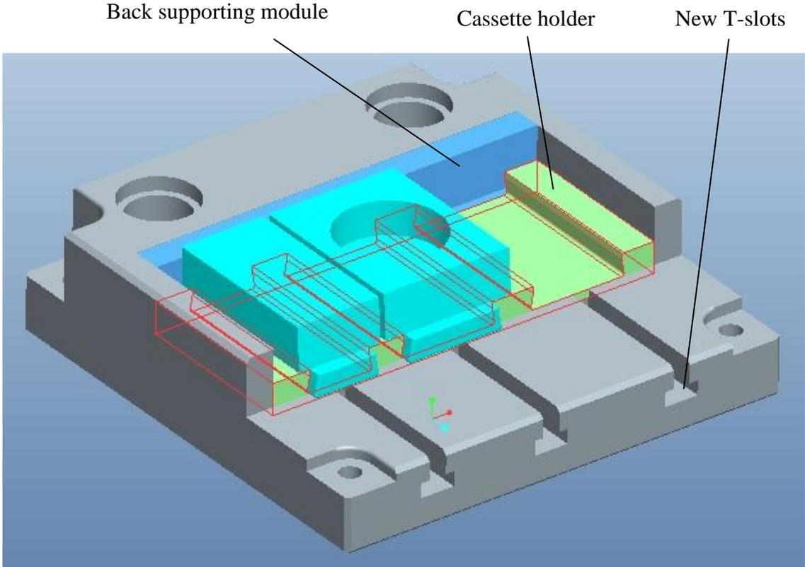
Figure 4.2 Dovetail cassettes, cassette holder, and back supporting module (Version-2)
