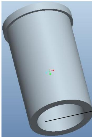
Conical internal part of the guide pin bushing
