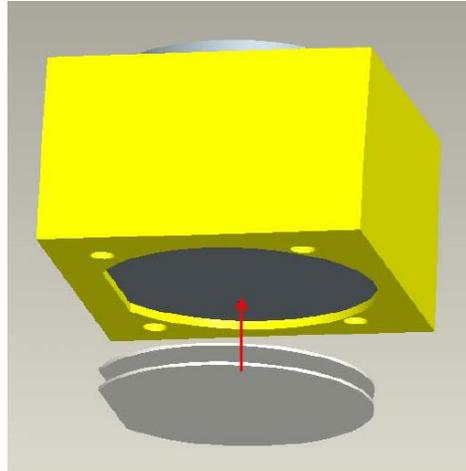
Figure 3.4 Height adjustment plates [11]
