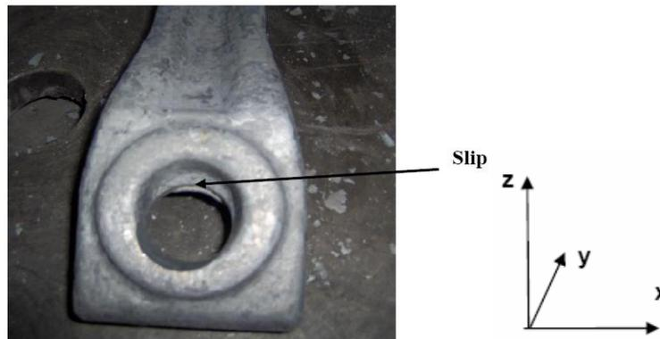
Figure 3.1 Slip problem due to horizontal misalignment [11]
