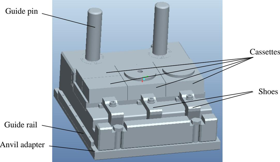
Figure 4.9 A view of the final die holder design (Version-4)
