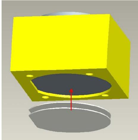
Figure 3.4 Height adjustment plates [11]
