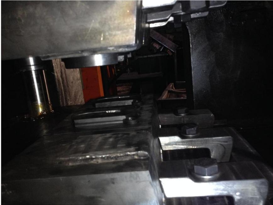
Figure 5.10 Die holders fully assembled with upper and lower die-cassette pairs on the 1000 ton hot forging press for production
