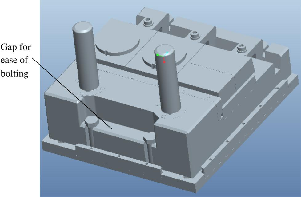
Figure 4.23 Lower die holder assembly
