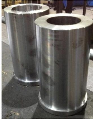
Figure 5.4 A view of the guide pin bushings
