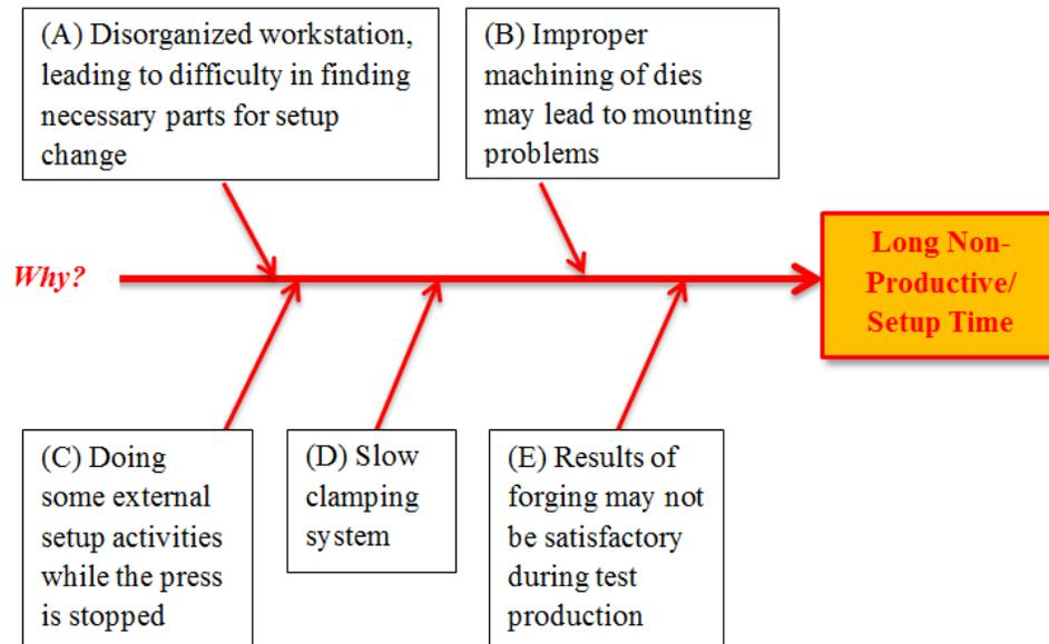
Figure 3.9 Fishbone diagram for the causes of long setup time on the 1000 ton forging press
