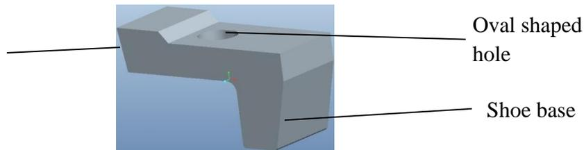
Figure 4.18 A view of the shoe for clamping cassettes
