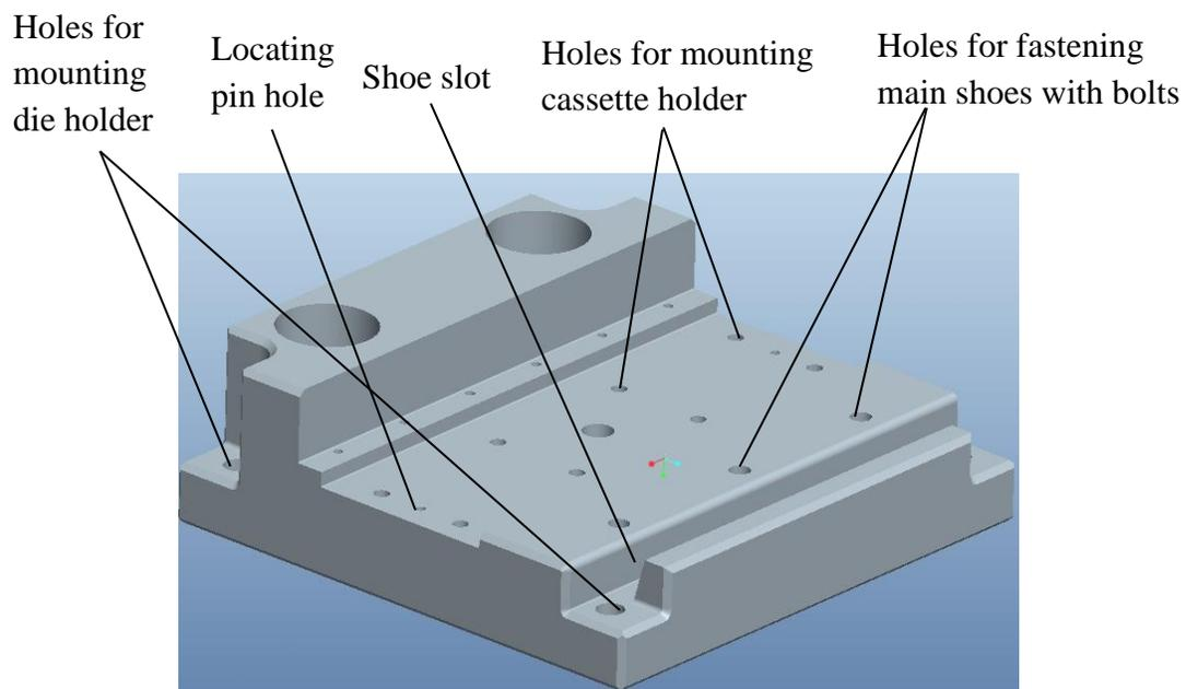
Figure 4.27 Solid model of the upper die holder
