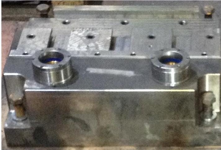
Figure 5.8 A view of the fully assembled upper die holder (rear view)
