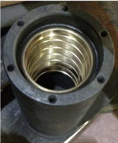
Figure 5.3 A view of the bronze insert fitted inside housing
