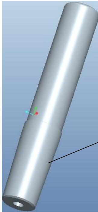
Conical lower part of the guide pin to be fixed in bushing
