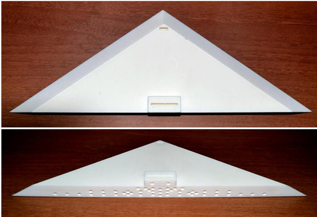
Figure 2-7 Photograph of the fabricated wing model
