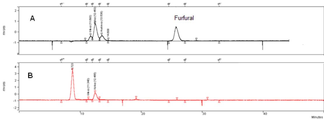
**Figure H.1** Chromatograms: A: furfural standard, B: After acid hydrolysis.
