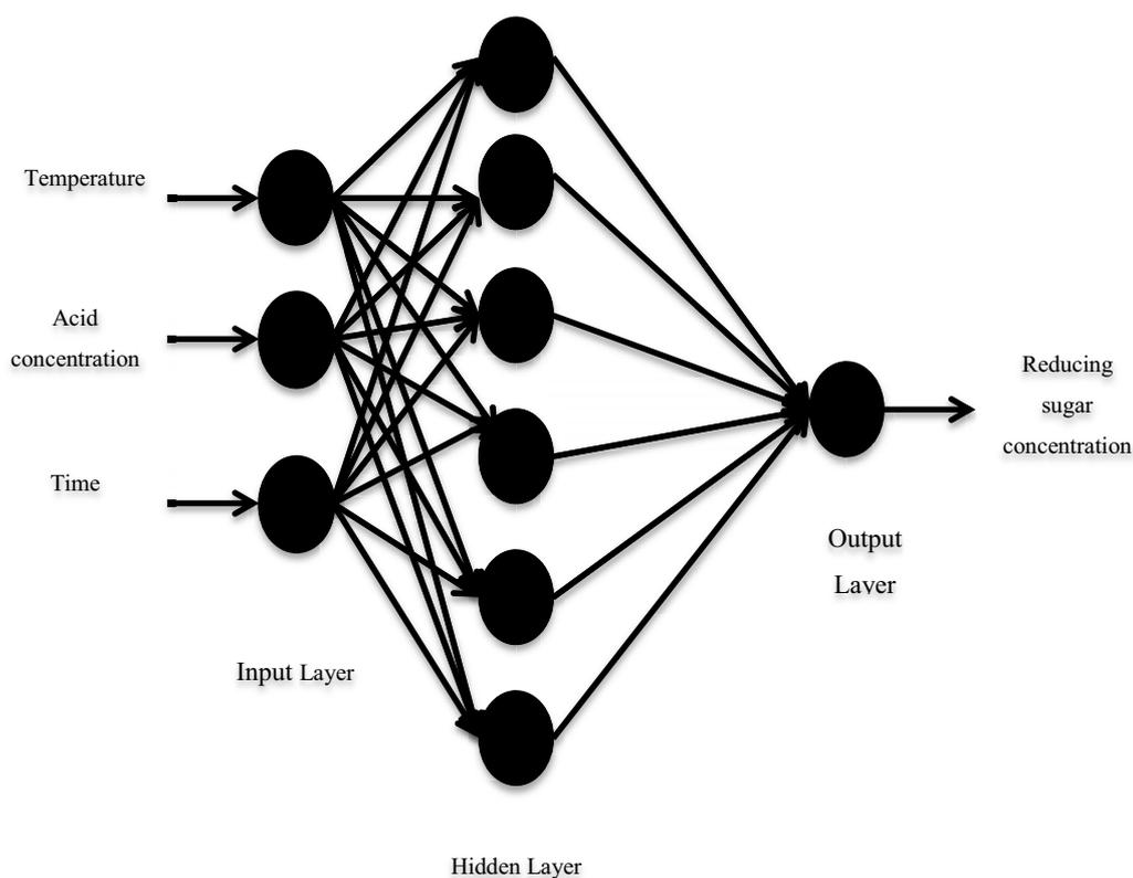
**Figure 4.10** Schematic representation of ANN to simulate the dilute acid pretreatment of hazelnut shells.
