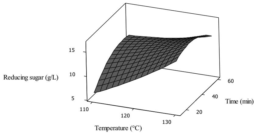
**Figure 4.6** Response surface plot for the effects of temperature and time on reducing sugars (acid concentration is constant at 3%, w/w).
