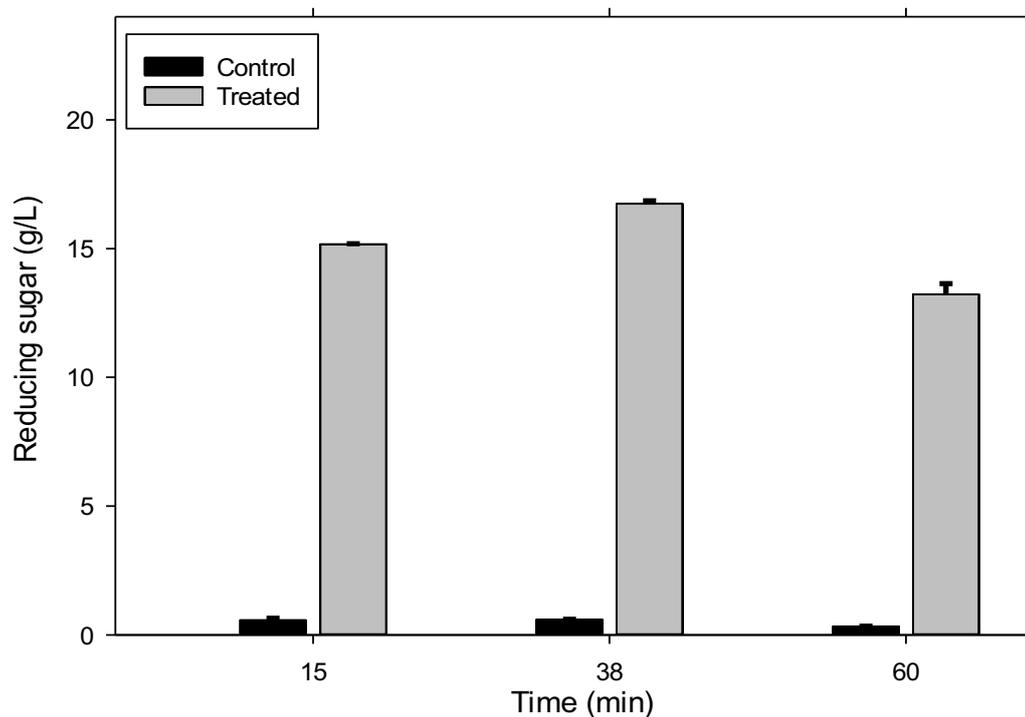
**Figure 4.4** Hydrolysis of hazelnut shells at various time (130 °C, 3%, w/w, acid)
