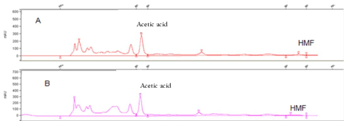
**Figure H.2** Chromatograms: A: HMF and acetic acid, B: After acid hydrolysis
