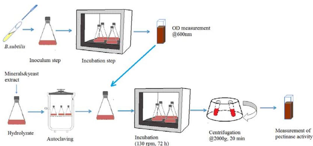
**Figure 3.4** Schematic of pectinase production steps
