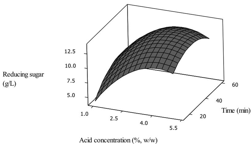
**Figure 4.5** Response surface plot for the effects of acid concentration, and time on reducing sugar (temperature is constant at 120 °C)
