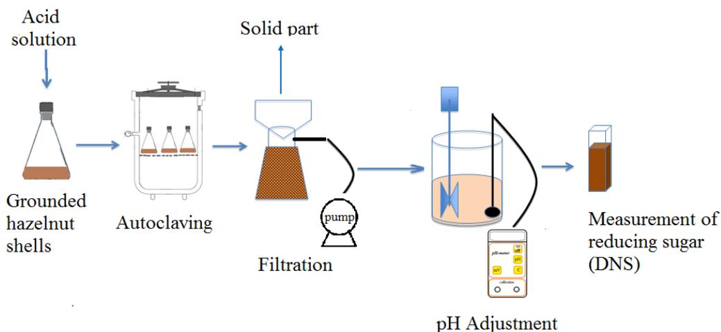
**Figure 3.1** Schematic of dilute acid pretreatment set up
