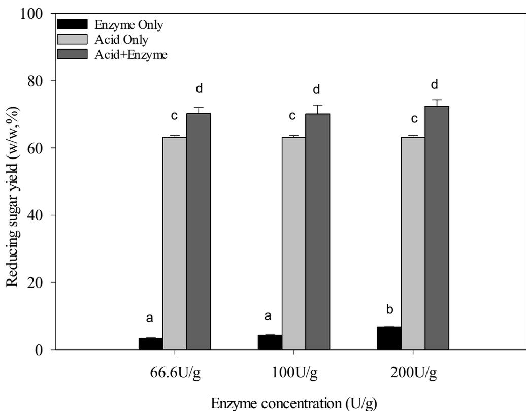
**Figure 4.14** Acid hydrolysis and combination of acid and enzymatic hydrolysis at 5% solid concentration and various enzyme loadings (50 °C, pH 5.0, 20 h at 130 rpm)
