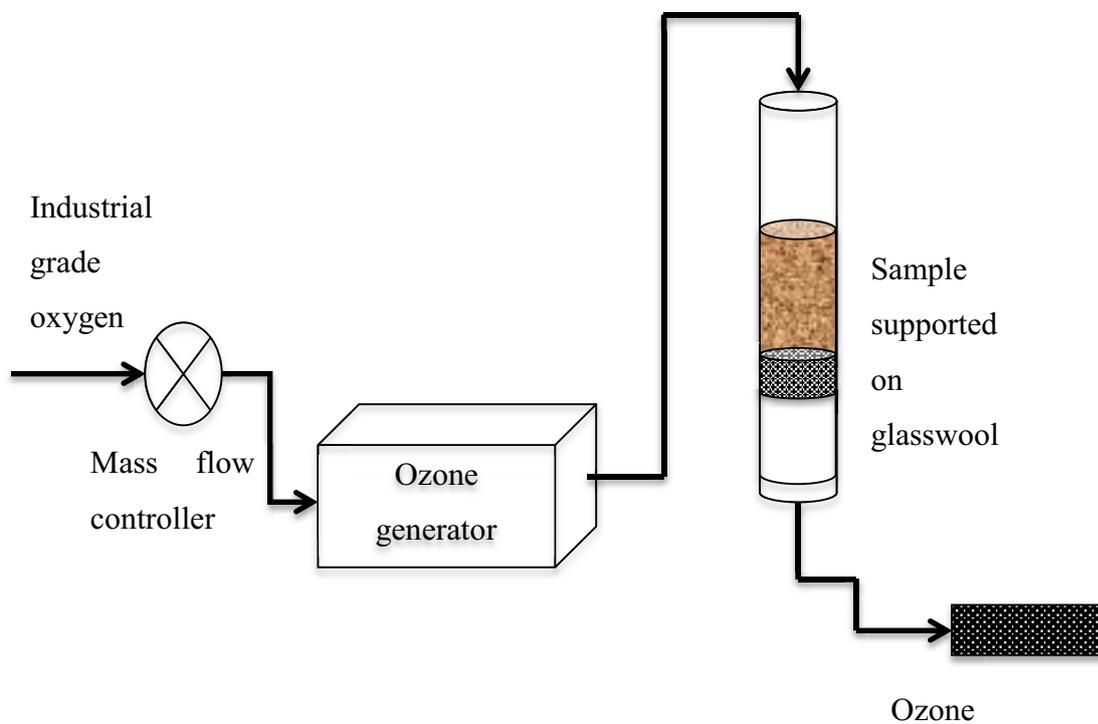
**Figure 3.3** Schematic of ozonolysis reactor set up –adapted from Panneerselvam et al. (2013)
