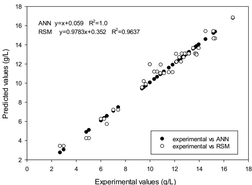
**Figure 4.11** Combined training, validation and testing predicted versus actual experimental values for an ANN with 6 neurons in the hidden layer and RSM
