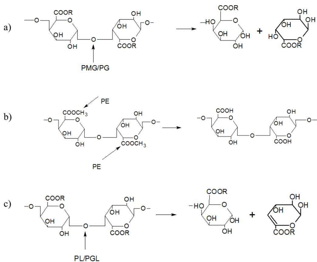
**Figure 2.1** Mode of action of pectinases: (a) R = H for PG and CH<sub>3</sub> for PMG; (b) PE; and (c) R = H for PGL and CH<sub>3</sub> for PL. The arrow indicates the place where the pectinase reacts with the pectic substances. PMG, polymethylgalacturonases ; PG, polygalacturonases ; PE, pectinesterase ; PL, pectin lyase (Jayani et al., 2005).
