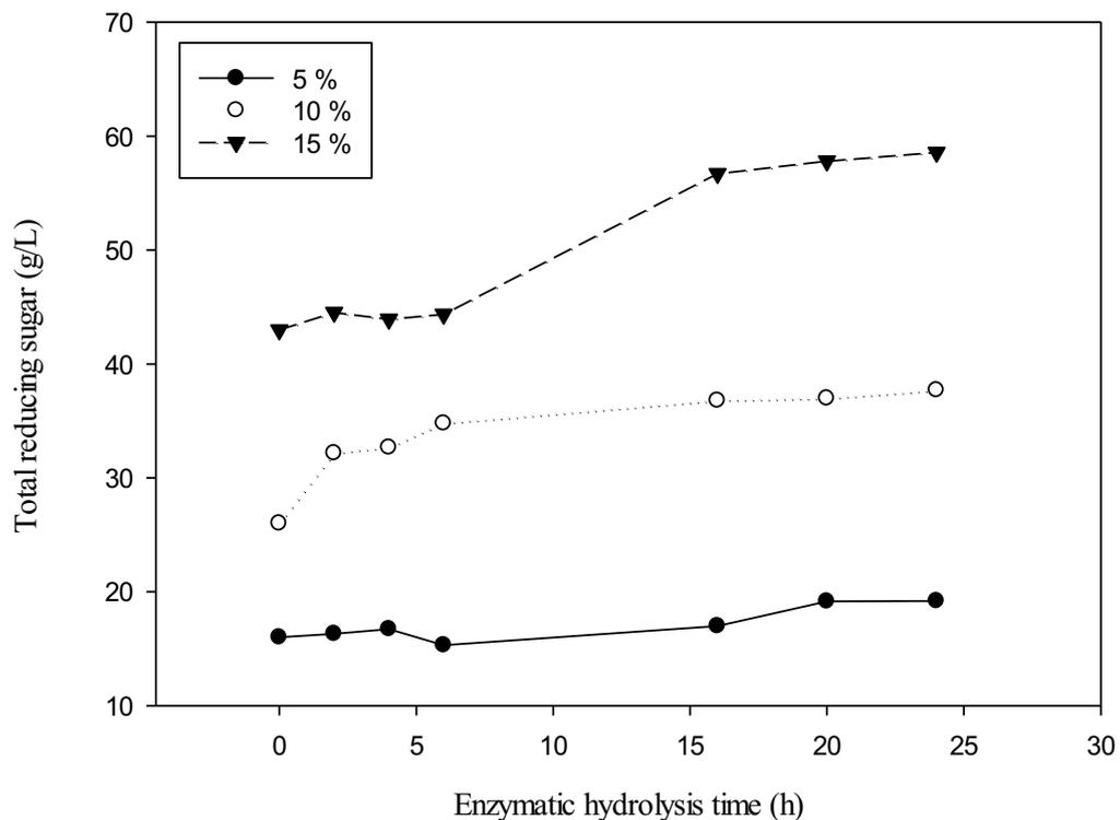
**Figure 4.12** Effect of solid/liquid ratio on the enzymatic hydrolysis time of hazelnut shells.
