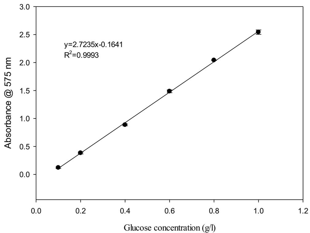
**Figure C.1** The standard curve for DNS method
