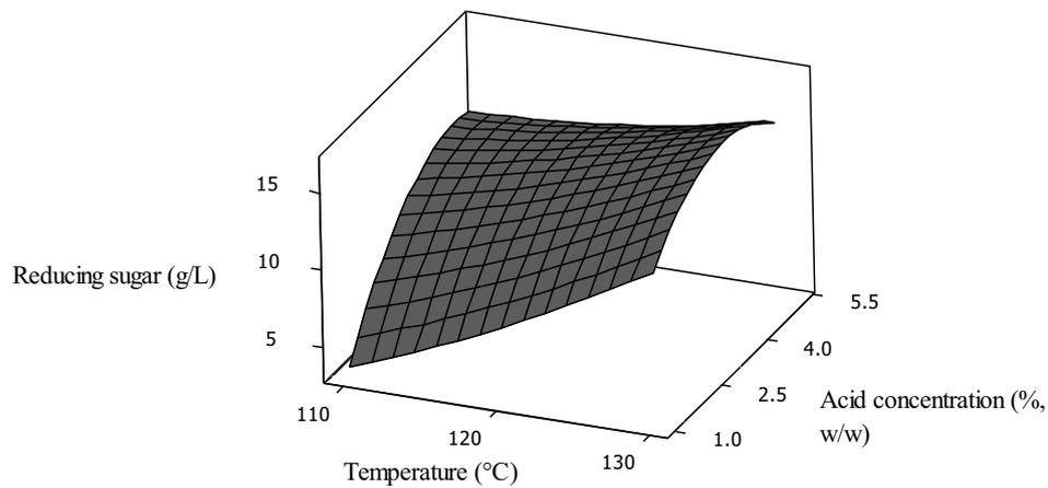
**Figure 4.7** Response surface plot for the effects of temperature and acid concentration on reducing sugars (time is constant at 37.5 min).
