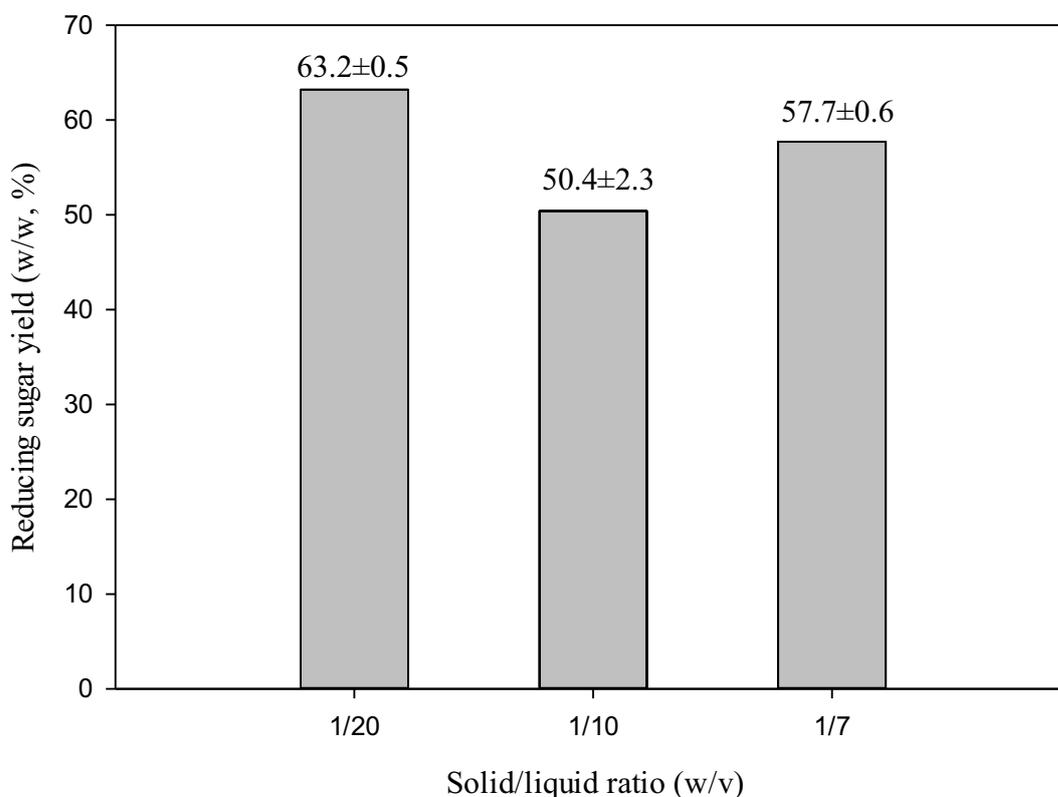
**Figure 4.1** Reducing sugar yield with respect to solid/liquid ratio (3%, w/w, acid, 130 °C, 30 min)
