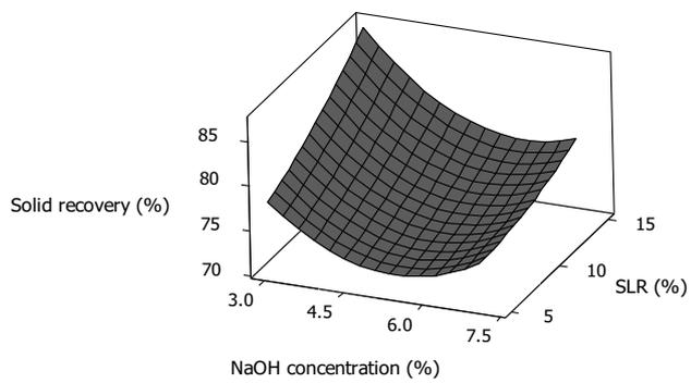
**Figure 4.15** Response surface plots for the effects of alkaline pretreatment conditions on solid recovery
