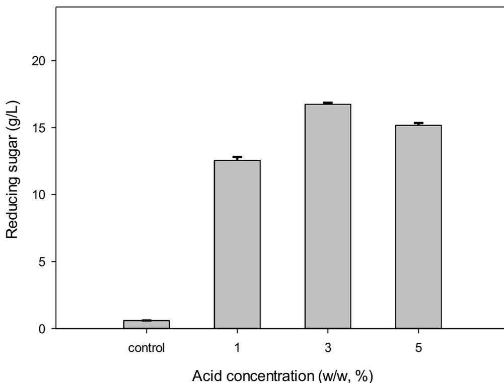
**Figure 4.3** Hydrolysis of hazelnut shell at various acid concentrations (130 °C, 37.5 min)
