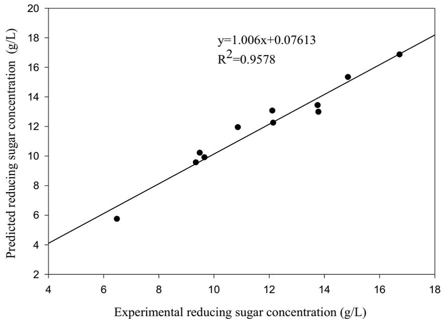
**Figure 4.9** Predicted vs. experimental reducing sugar concentration for validation of the response surface model.
