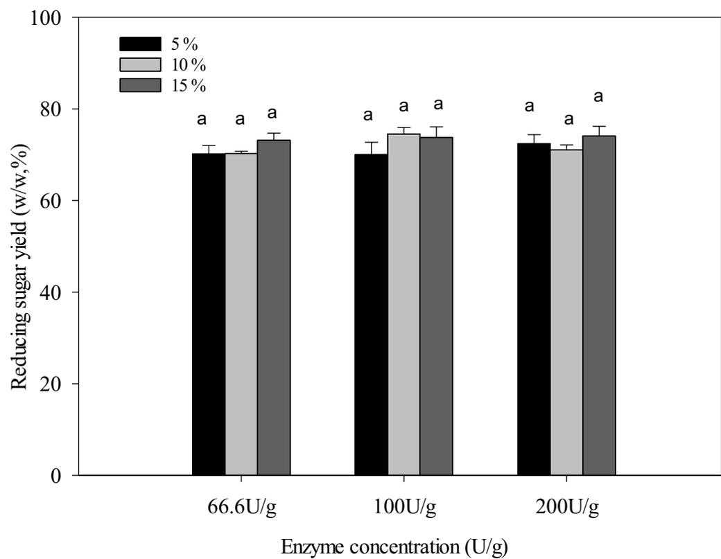
**Figure 4.13** Enzymatic hydrolysis at various solid concentration (5, 10 and 15%) of hazelnut shell and enzyme loadings (50 °C, pH 5.0, 20 h at 130 rpm)
