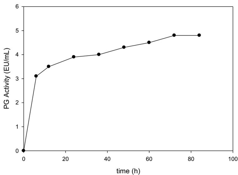
**Figure 4.22** Time course of pectinase production by *B.subtilis* at pH 7.0, 30 °C and with shaking at 130 rpm.
