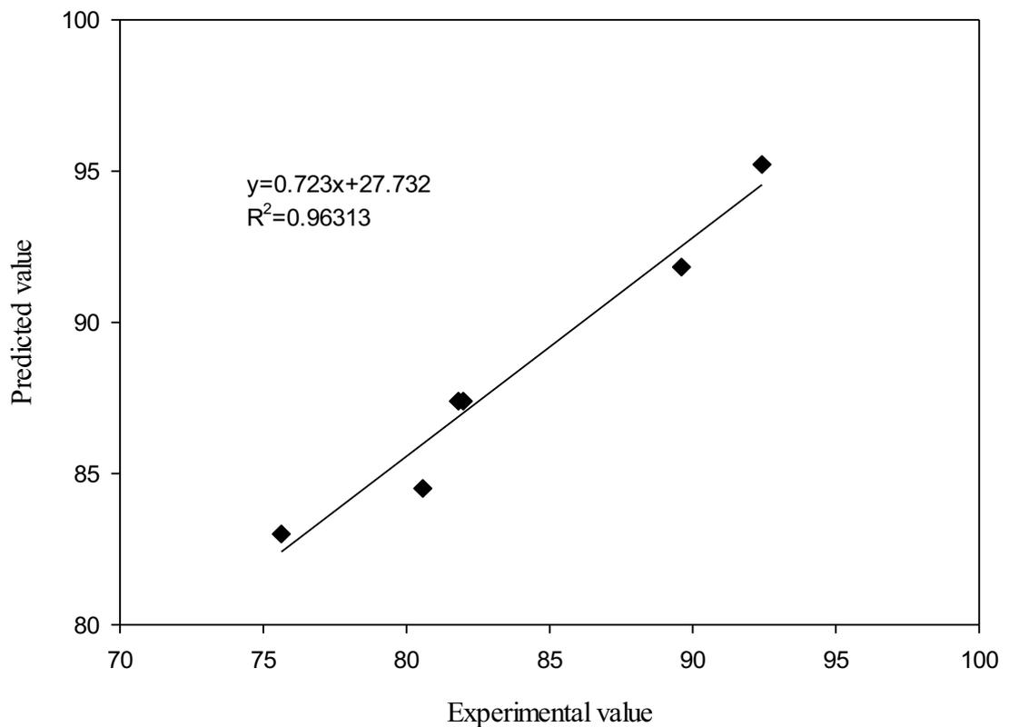
**Figure 4.31** Verification of the model obtained by RSM
