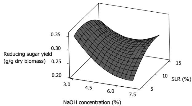
**Figure 4.19** Response surface plots for the effects of alkaline pretreatment conditions on reducing sugar yield (g/g dry biomass)
