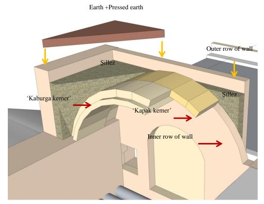
Figure 4. 23 Roof structure on vault system
