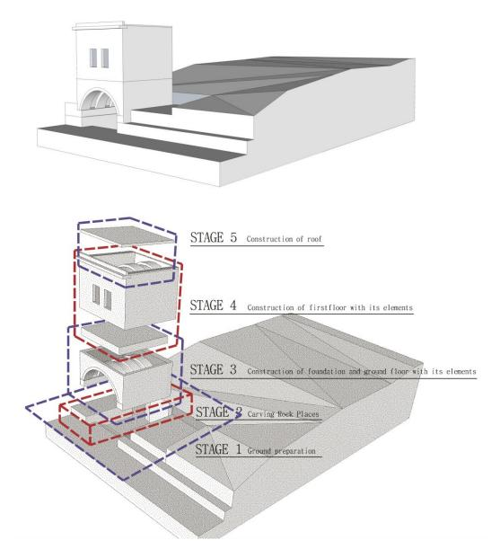
Figure 4. 1 Construction stages of scenario
