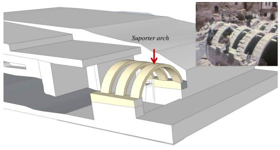
Figure 4. 15 Supporter arches of vault
