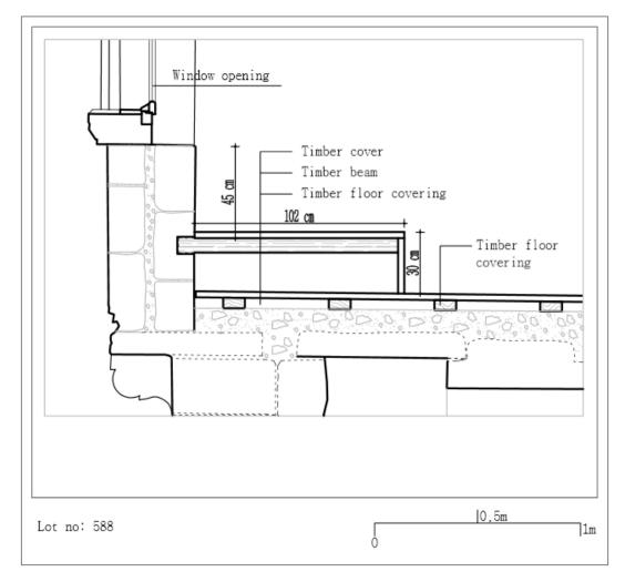
Figure 3. 124 Timber seki drawing
