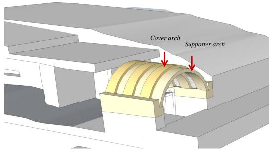
Figure 4. 16 Cover arch added to supporter arches
