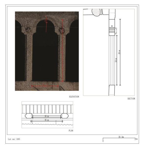
Figure 3. 110 Aiwan arch spanned openning
