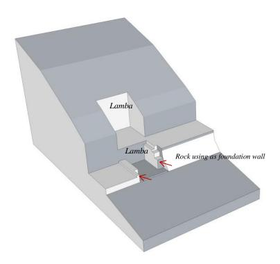
Figure 4. 2 'Lamba' and rock using as foundation wall
