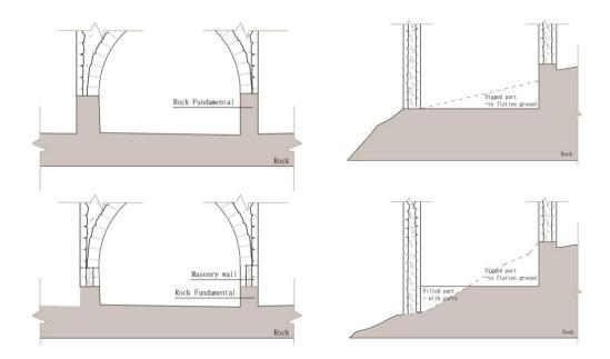
Figure 3.19 Flat land with rock foundation walls - Low-sloped land preparation
