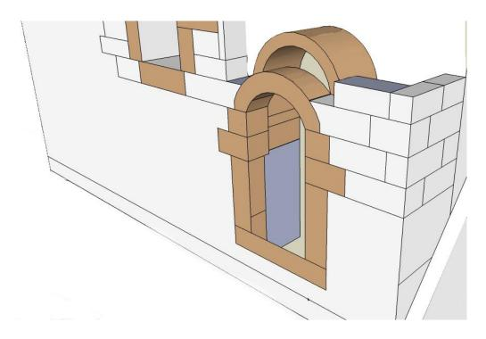
Figure 4. 9 Double arched door during construction process
