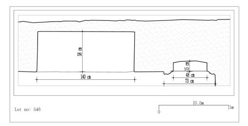
Figure 3. 146 Orthophoto elevation and plan of yüklük and lambalık
