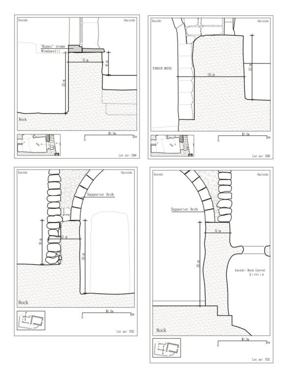
Figure 3. 25 Variations of rock as foundation wall
