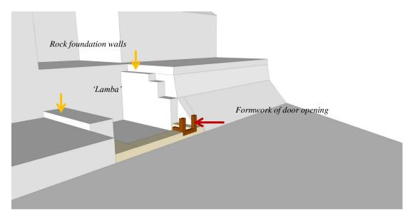
Figure 4. 7 Door formwork with side stones
