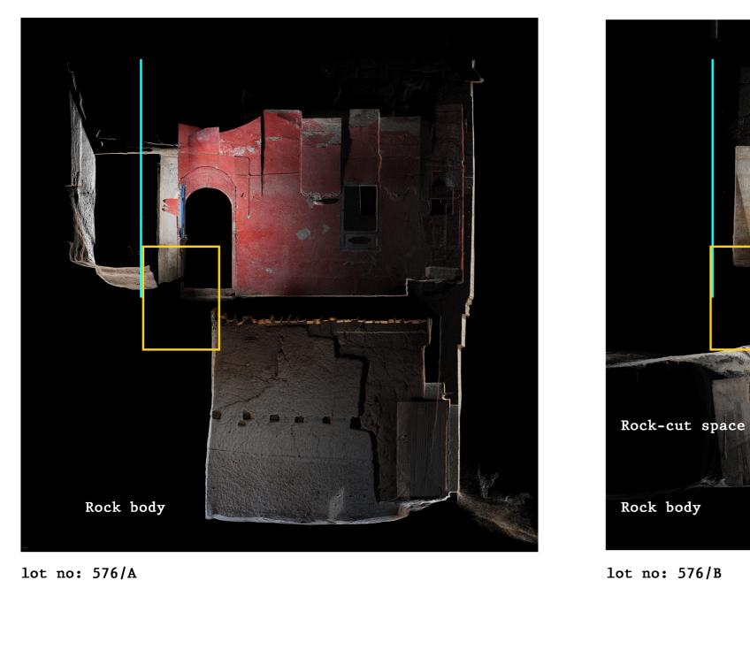
Upper storey back wall draw back from the line of ground storey and set up on rock base
