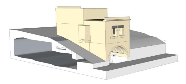
Figure 4. 5 Rock-cut places underneath of masonry structure
