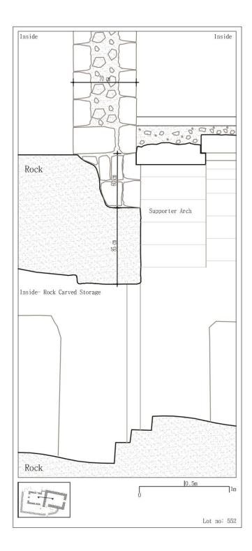
Figure 3. 75 Masonry structure connection with rock carved place
