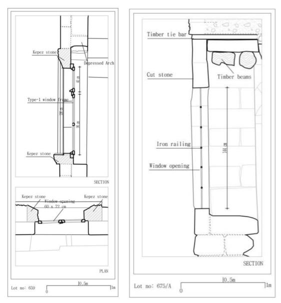
Figure 3. 103 Stone Arch Lintel window
