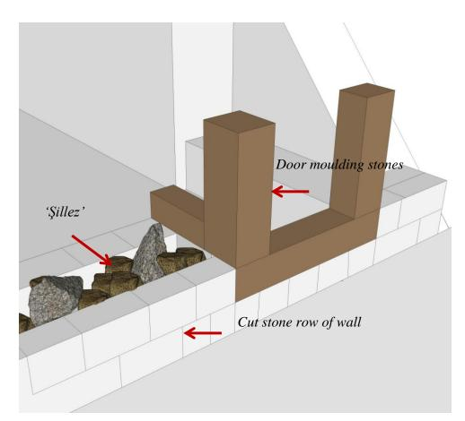
Figure 4. 6 Wall section of double sided wall filled with sillez and door formwork
