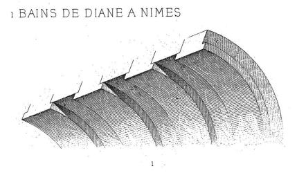
Figure 2. 12 Vault system that is used in Roman bath structure (Choisy, 1873)
