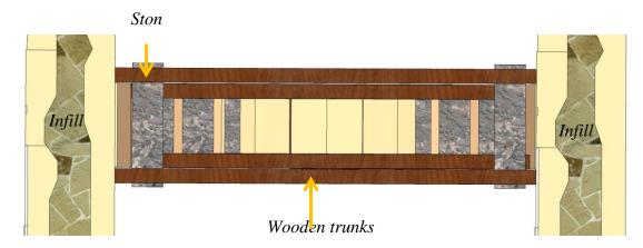
Figure 4. 11 Formwork of vault
