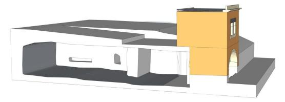
Figure 4. 19 Upper storey back wall extending back through on rock base
