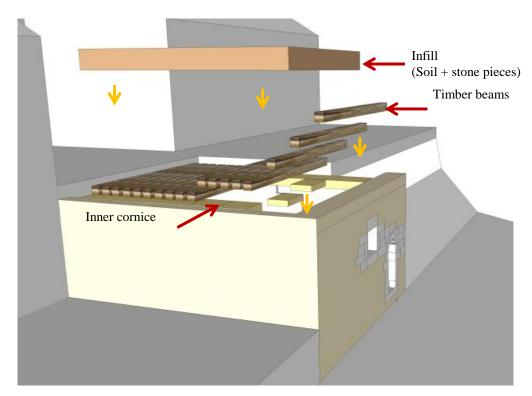
Figure 4. 18 Timber superstructure process
