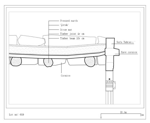
Figure 3. 62 Earth roof on timber beam superstructure
