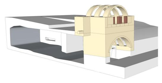
Figure 4. 22 Upper floor window formwork and supporter arches
