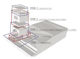
Figure 1. 5 A script of a building visualized within 3D models
