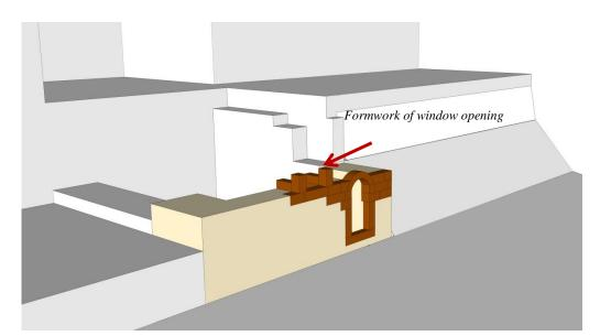
Figure 4.8 Window formwork in ground floor
