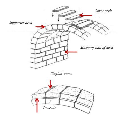
Figure 4. 17 Cover arch added to supporter arches (Contunie)
