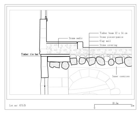
Figure 3. 48 Timber beam superstructure drawing
