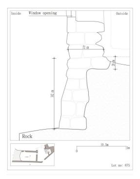
Figure 3. 27 Masonry wall placed in front of rock mass
