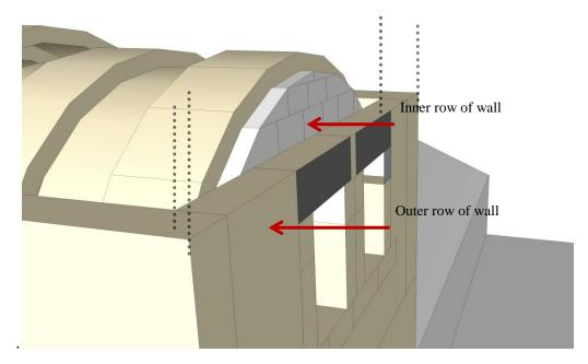
Figure 4. 20 Cover vault is placed on inner row of double sided wall of front façade
