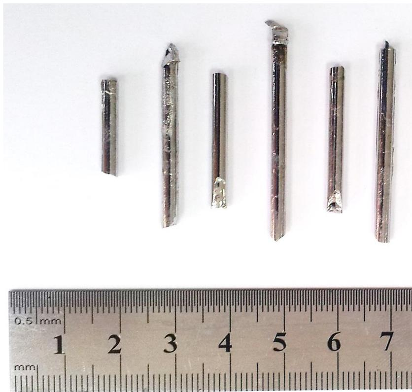
**Figure 5.1**  $M_{60}Cr_{13}Mo_{17-x}B_8Y_2Mn_x$  samples fabricated by suction casting
