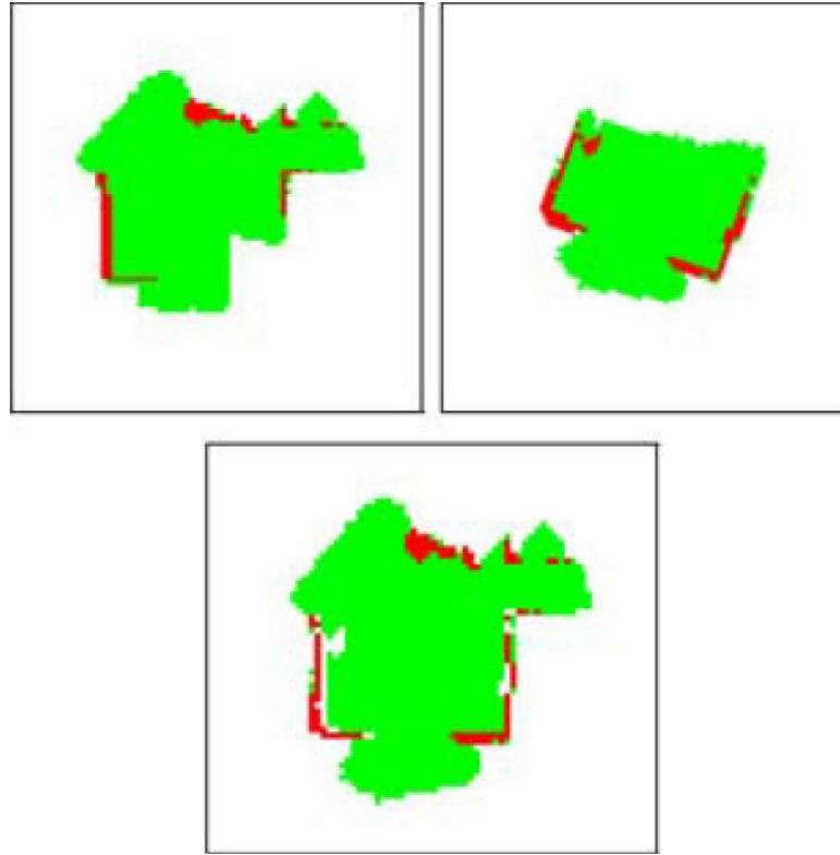
Figure 7 The upper two maps explored by different robots are merged into the lower resultant map [11].
