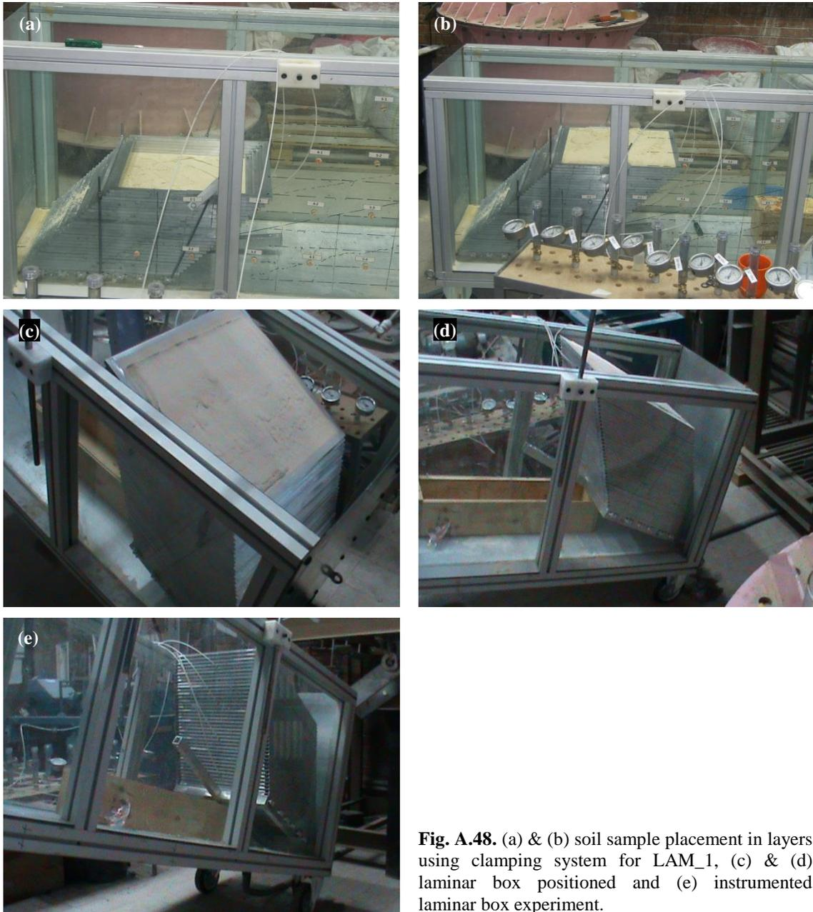
**Fig. A.48.** (a) & (b) soil sample placement in layers using clamping system for LAM\_1, (c) & (d) laminar box positioned and (e) instrumented laminar box experiment.
