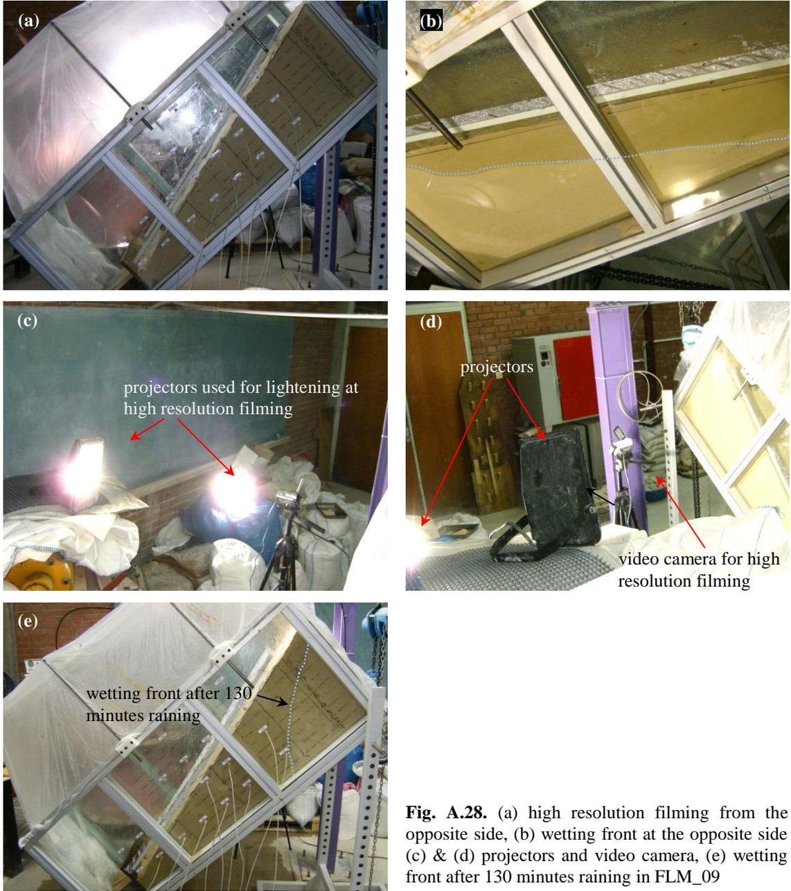
**Fig. A.28.** (a) high resolution filming from the opposite side, (b) wetting front at the opposite side (c) & (d) projectors and video camera, (e) wetting front after 130 minutes raining in FLM\_09
