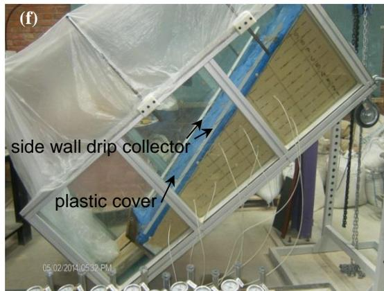
**Fig. A.15.** Geonet in the base of flume, (b) filter material and soil layer placement, (c) placement of tensiometers and dry density checkup tares, (d) fully placed sample, (e) trimmed soil sample and (f) tilted flume, covered surface and left for equalization in FLM\_05
