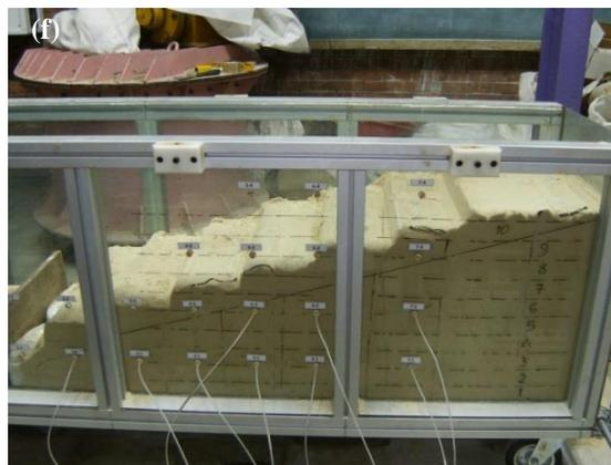
**Fig. A.21.** (a) wall inclinometers, (b) placement of tensiometers, (c), (d), (e) & (f) placement of soils for FLM\_07
