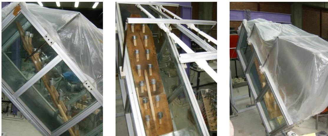
**Fig. 4.19.** Rainfall intensity checkup over inclined surface
