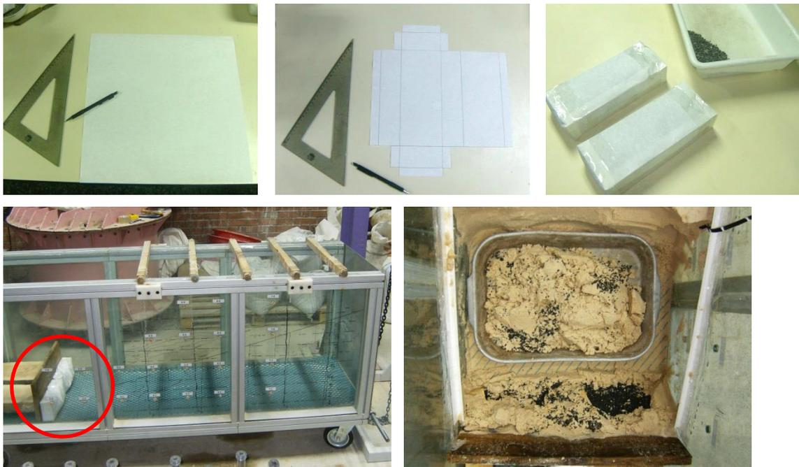
Fig. 4.27. Filter material preparation, placement and removing after test.
