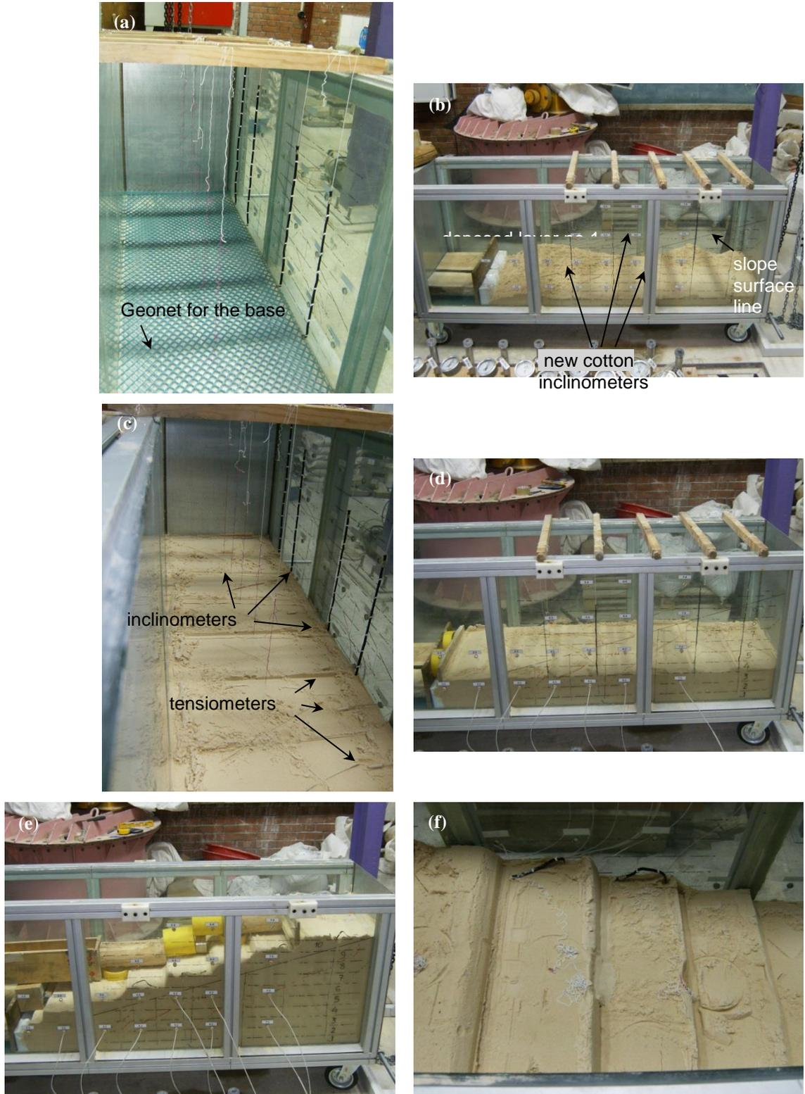
**Fig. A.18.** (a), (b) & (c) mounted new inclinometers, placement of tensiometers and relative density checkup tares, (d) placed of soil layers, (e) & (f) fully placed sample for FLM\_06
