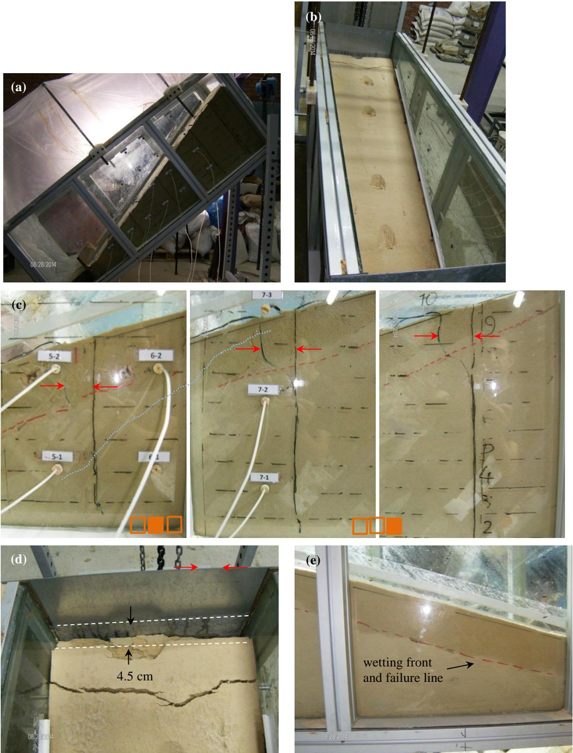
**Fig. A.40.** (a) high resolution filming from the opposite side, (b) slipped slope surface (c) inclinometers showing deformation at the time of failure, (d) slipped soil (top view), (e) wetting front and failure line at FLM\_13
