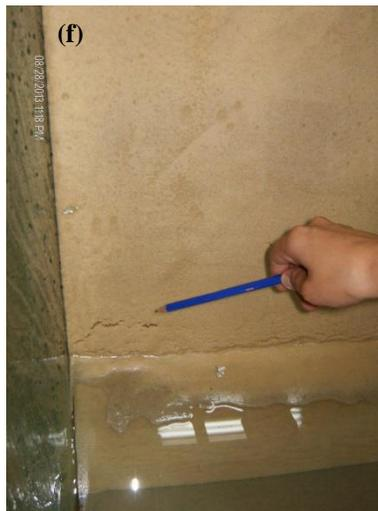
**Fig. A.3.** (a) positioned flume (slope), (b) rainfall spraying, (c) measurement of wetting front progress, (d) wetting front at the time of failure, (e) accumulation of water at toe of slope, (f) no failure in slope due to raining in FLM\_00
