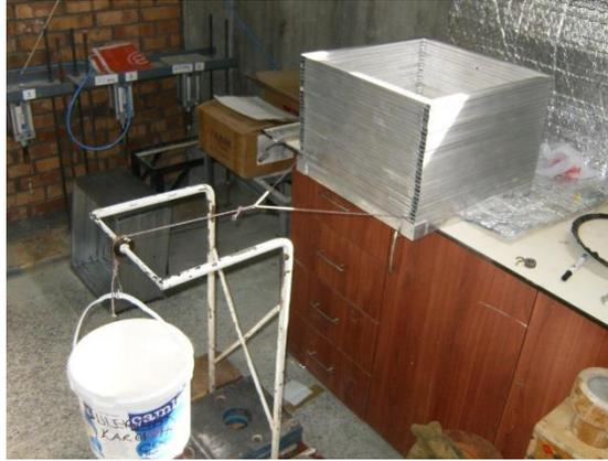
**Fig. 4.40.** Setup for assessing friction between laminates
