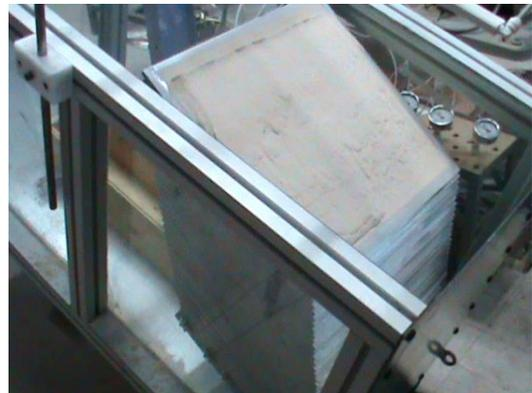
**Fig. 5.1.** Laminar box test setup representing a vertical slice in an infinite slope
