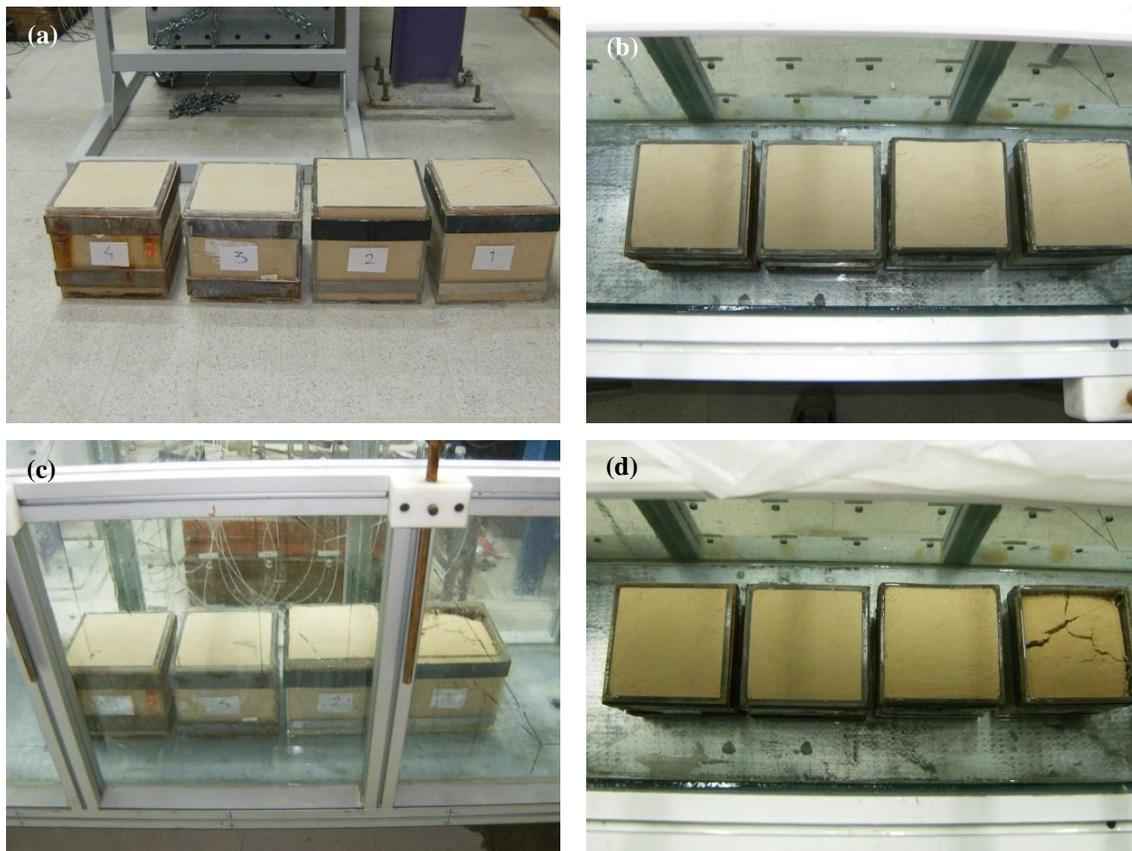
**Fig. 4.2.** Cubic samples subjected to rainfall to obtain minimum dry density with no volume change under rainfall, (a) & (b) before and (c) & (d) after applying rainfall
