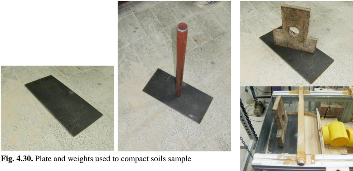
**Fig. 4.30.** Plate and weights used to compact soils sample
