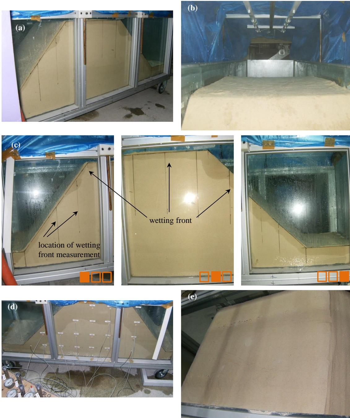
**Fig. A.5.** (a) Constructed 2-sided slope subjected to rainfall for FLM\_01, (b) covering flume box to have more controlled intensity for rainfall, (c) wetting front and locations of measurement, (d) instrumentations (pore pressure transducers and PCDR devices and (e) crest of the slope after raining, no failure crack (FLM\_01).
