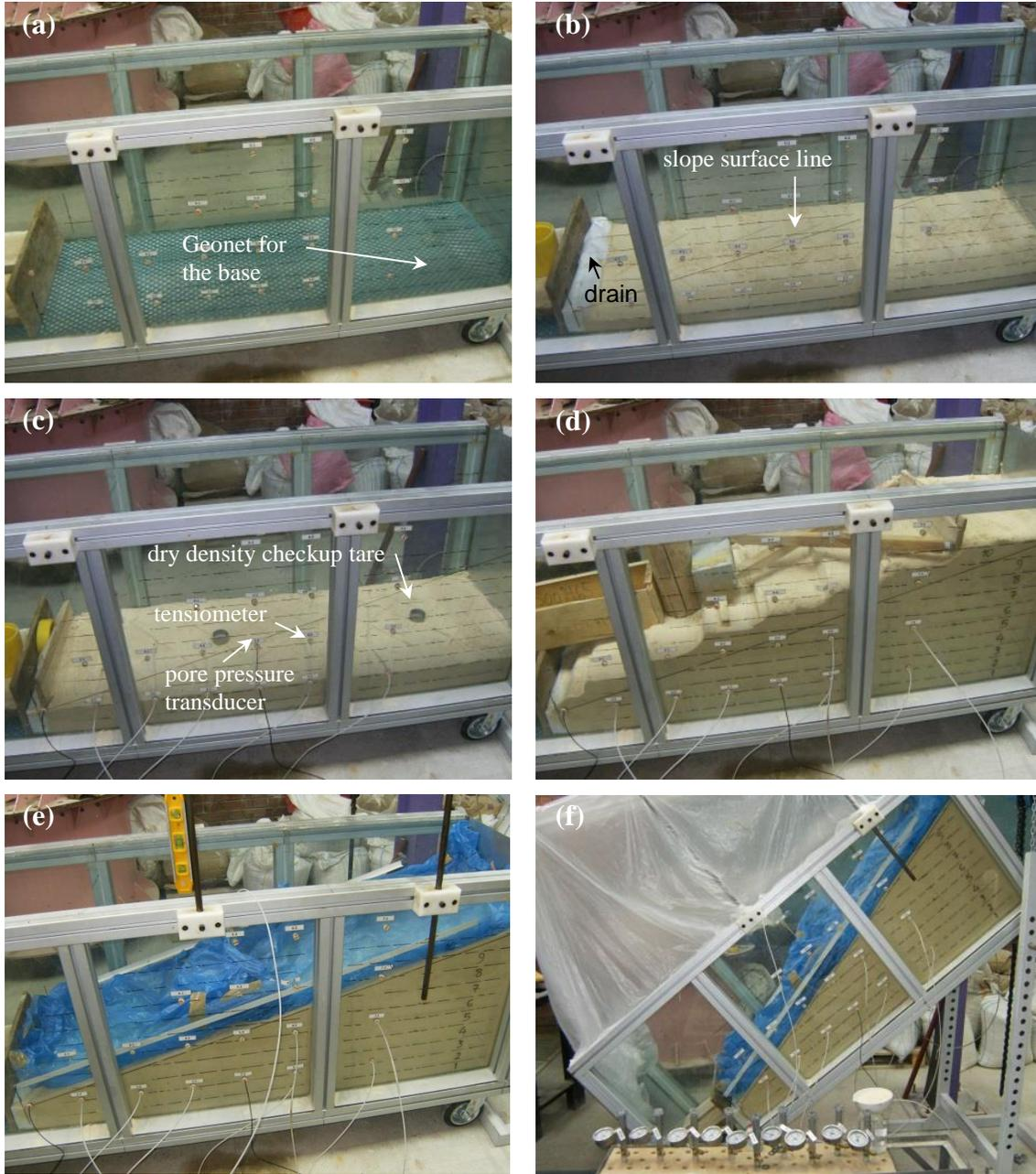
**Fig. A.9.** (a) Geonet in the base of flume, (b) filter material and soil layer placement, (c) placement of tensiometers and dry density checkup tares, (d) fully placed sample, (e) trimmed soil sample and (f) tilted flume, covered surface and left for equalization in FLM\_03
