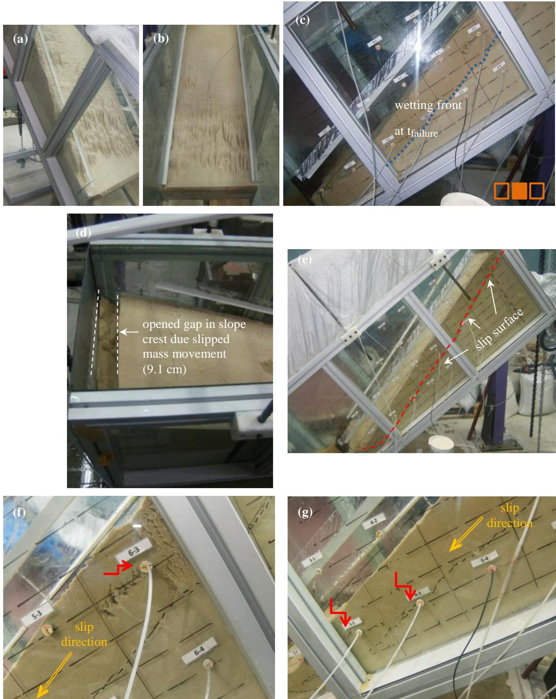
**Fig. A.10.** (a) & (b) desiccated soil surface, (c) wetting front at the time of failure, (d) slipped soil (top view), (e) slipped soil (side view), (f) & (g) disturbance in slipped mass in vicinity of tensiometers in FLM\_03
