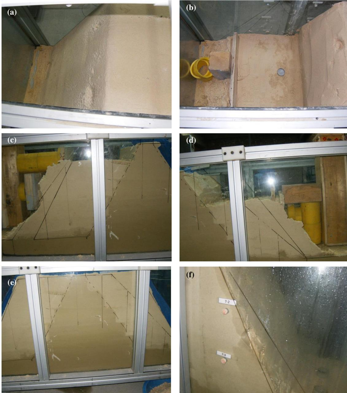
**Fig. A.7.** (a) & (b) Right slope surface from FLM\_01 which is trimmed in FLM\_02, (c) & (d) controlled deposition of right and left slopes for FLM\_02, (e) slope shape (covered till test date) and (f) slope subjected to rainfall for FLM\_02
