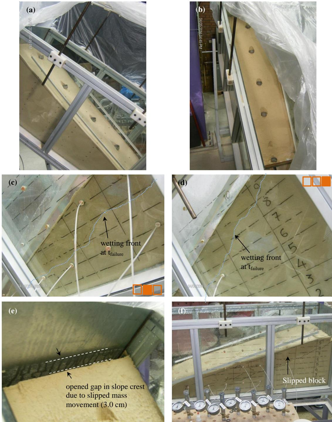
**Fig. A.13.** (a) & (b) placement of intensity checkup tares on soil surface, (c) & (d) wetting front at the time of failure, (e) deformation in slope crest (top view), (f) slipped soil block in FLM\_04
