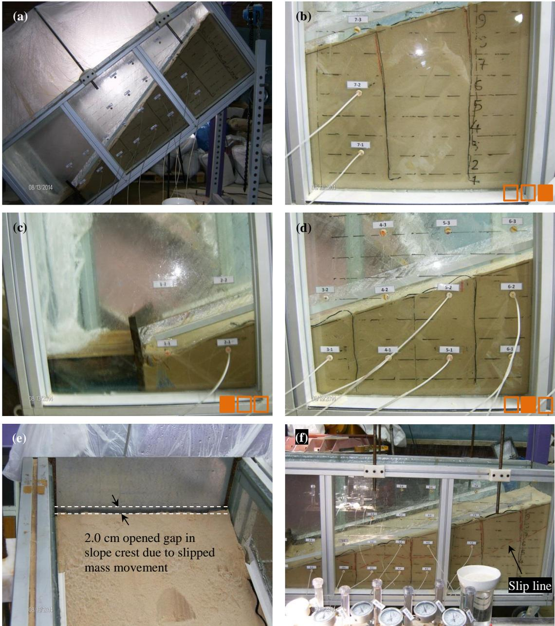
**Fig. A.34.** (a) high resolution filming from the opposite side, (b), (c) & (d) no failure in the slope subjected to 28 mm/hr rainfall intensity, (e) & (f) failure after 66 mm/hr rainfall application in FLM\_11
