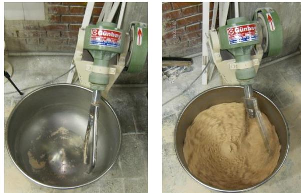
**Fig. 4.29.** Bakery blender used to mix misted soil
