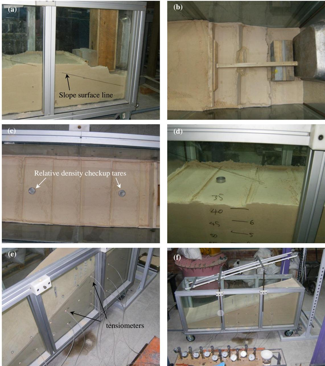
**Fig. A.2.** (a) Sample placement in layers with no drain in slope toe, (b) soil layer placement, (c) placement of relative density checkup tares, (d) controlled compaction of soil layers, (e) placed instrumentation (tensiometers) and (f) trimmed soil slope for FLM\_00
