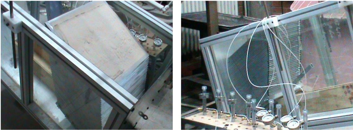
**Fig. 4.44.** Positioning laminar box setup within flume box
