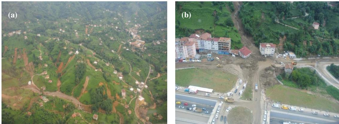
**Fig. 1.3.** (a) Shallow landslides occur after an intense rainfall in a part of Black Sea Region, (b) threatening and destroying buildings
