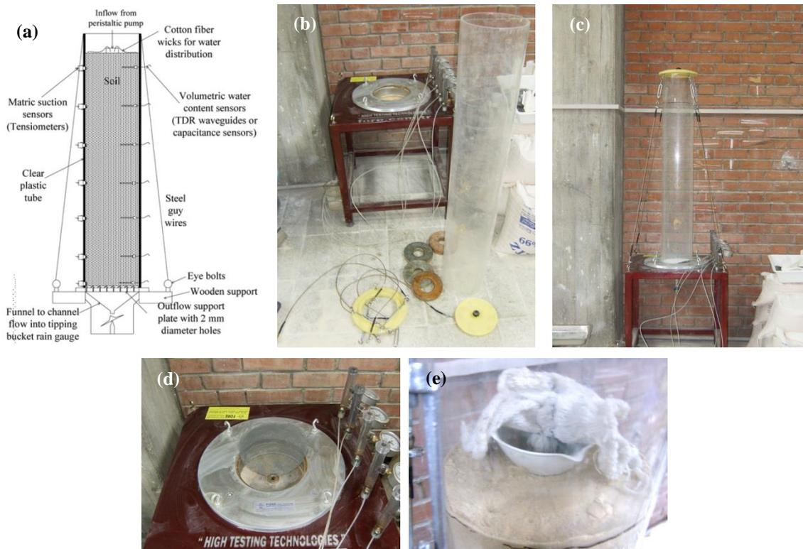
**Fig. 4.9.** Infiltration column setup designed, manufactured for METU geotechnical laboratory (a) sketch proposed by ASTM D7664, (b) dispatched parts and (c) montaged infiltration column setup, (d) water drain on pedestal and filter close up and (e) tools for ponding into the sample (water cup + cotton wicks).
