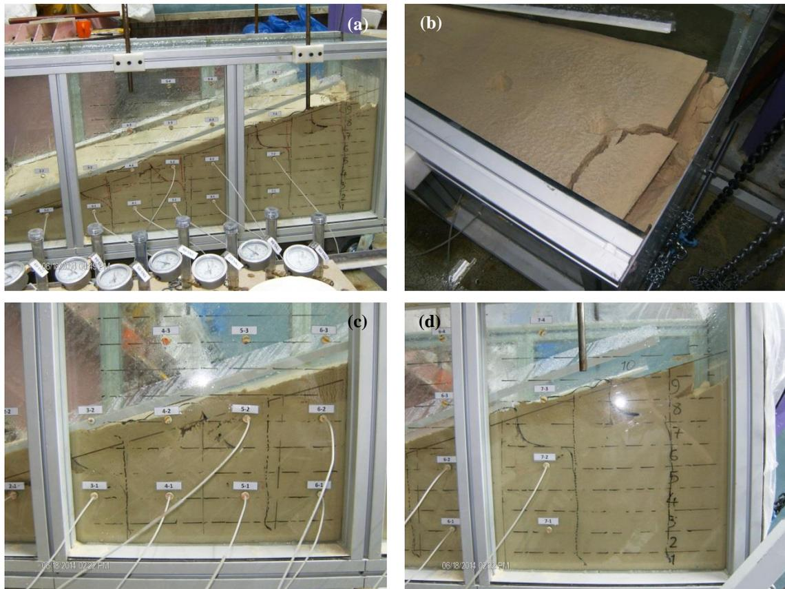
**Fig. 6.10.** (a) Failure surface projection on monitoring side wall of the flume box, (b, c & d) side and top views of the failed mass (M: middle inclinometers, W: wall inclinometers) for FLM\_08 flume test and (e) plot of inclinometers and emerging failure surface
