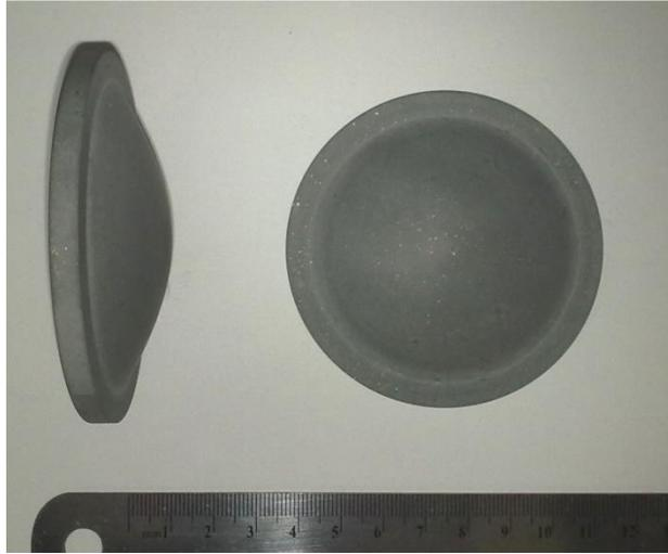
Figure 3.9 Polymeric lenses used in free-space measurement system.
