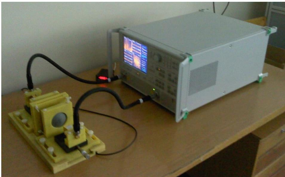
Figure 3.11 Custom-designed and built free-space measurement system and the utilized network analyzer.
