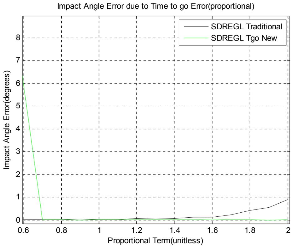
Figure 60 Impact Angle Error due to Time to go Error (proportional/ stationary)
