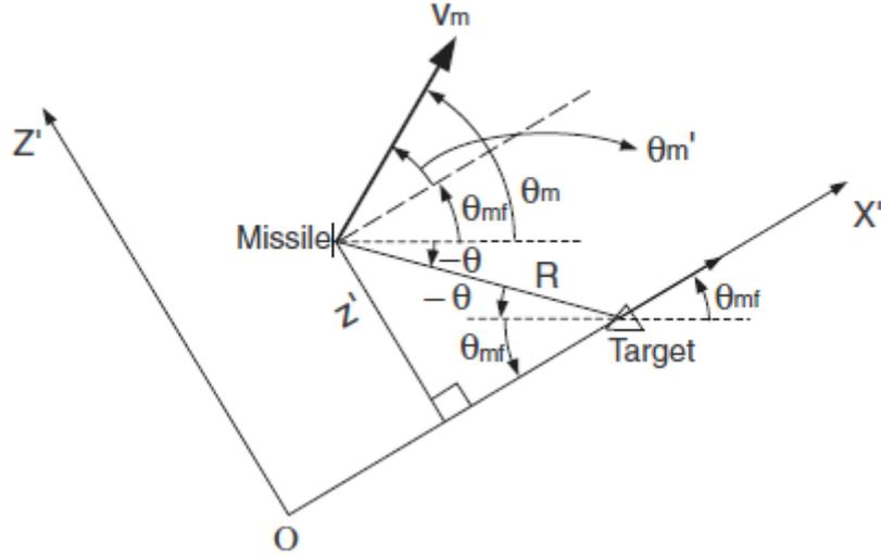
Figure 10 New Reference Frame for SDREGL
