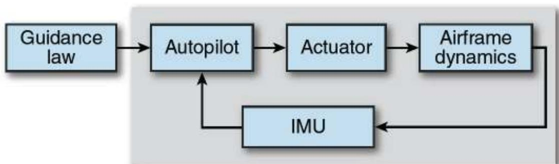
Figure 5 Missile Flight Control System
