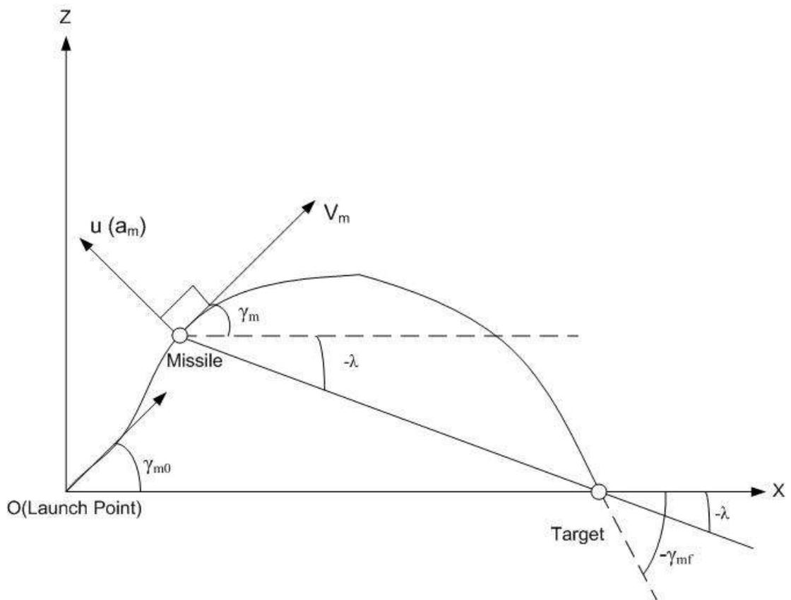
Figure 6 Engagement Schematic for Stationary Target
