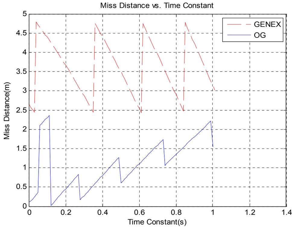
Figure 43 Miss Distance vs. Time Constant (non-stationary target)
