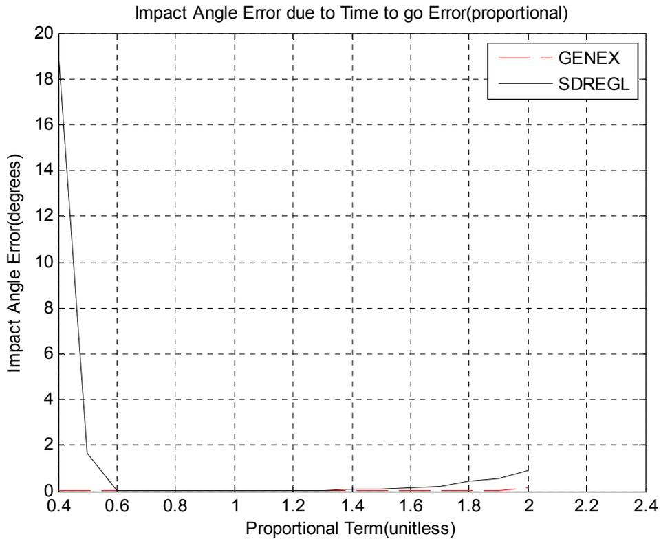
Figure 50 Impact Angle Error due to Time to go Error (proportional/stationary)
