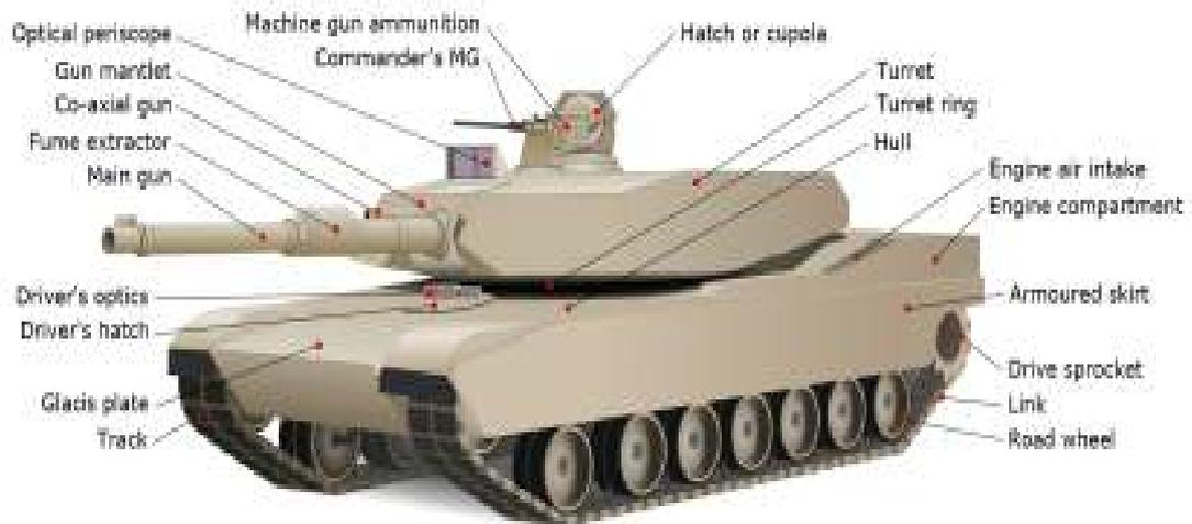
Figure 1 Main Battle Tank Components
