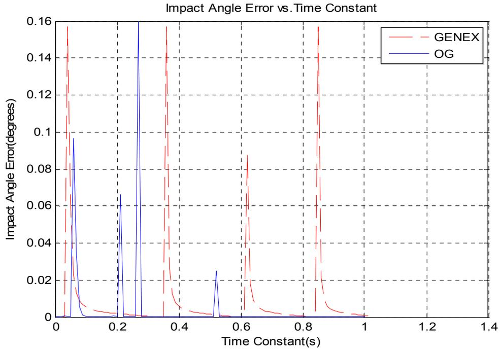
Figure 44 Impact Angle vs. Time Constant (non-stationary target)
