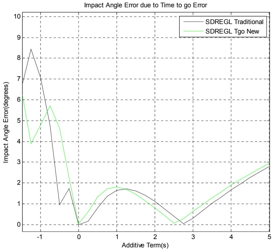
Figure 56 Impact Angle Error due to Time to go Error (additive/stationary)
