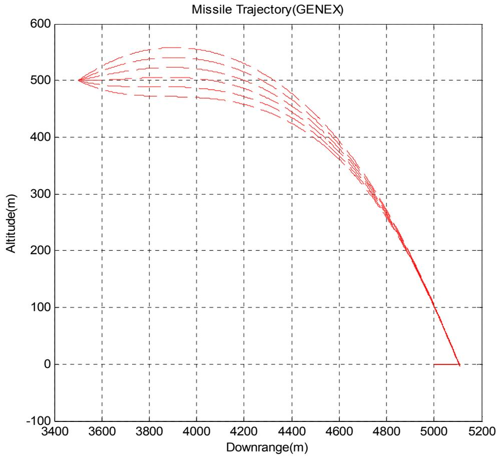
Figure 34 Missile Trajectory for Various TGH Angles
