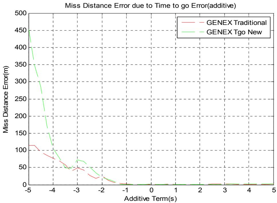
Figure 53 Miss Distance Error due to Time to go Error (additive/non-stationary)
