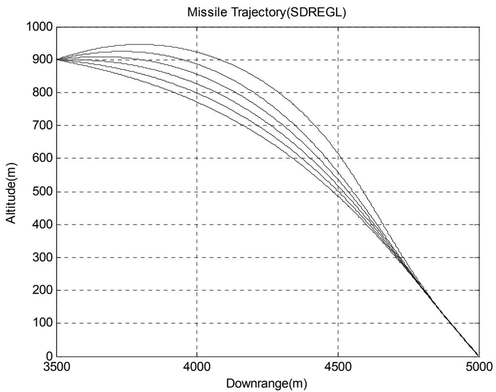
Figure 25 Missile Trajectories for Various TGH Angles (SDREGL)
