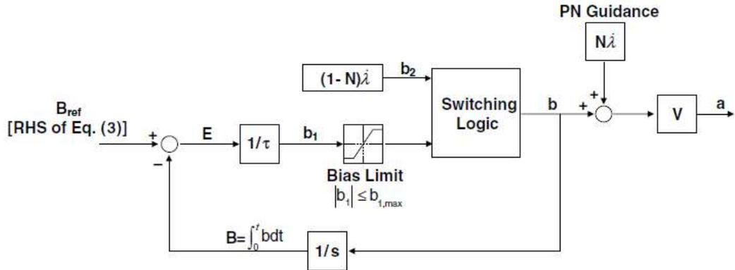
Figure 9 Bias Switching Logic
