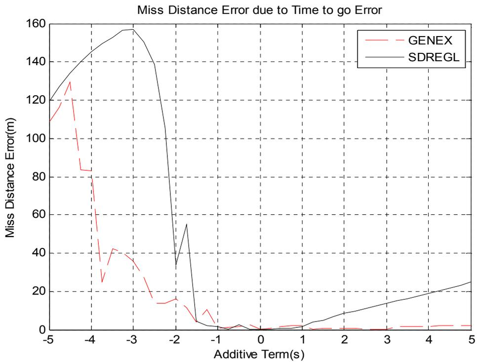
Figure 45 Miss Distance Error due to Time to go Error (additive/ stationary target)
