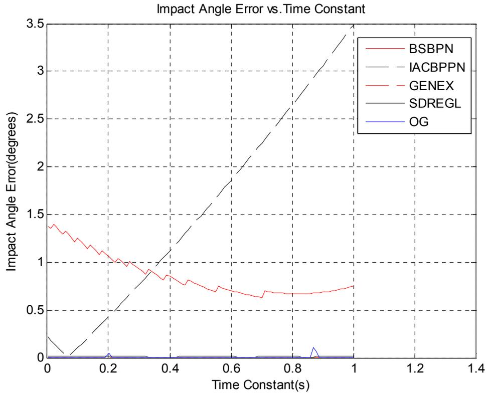
Figure 42 Impact Angle Error vs. Time Constant (stationary target)
