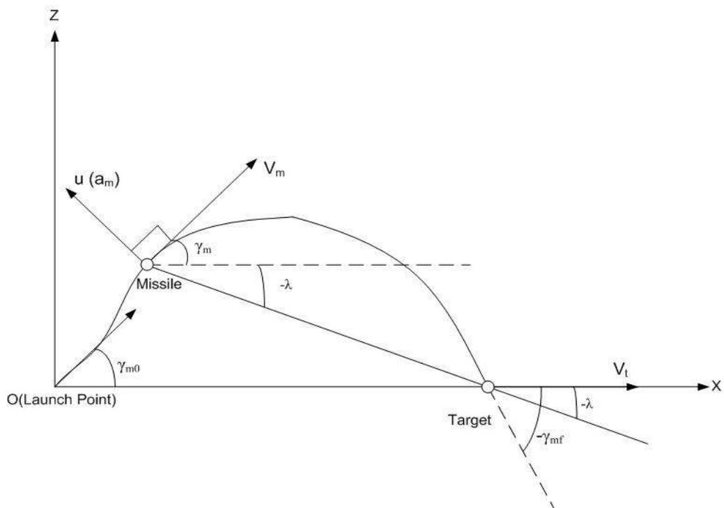
Figure 7 Engagement Schematic for a Non Stationary Target
