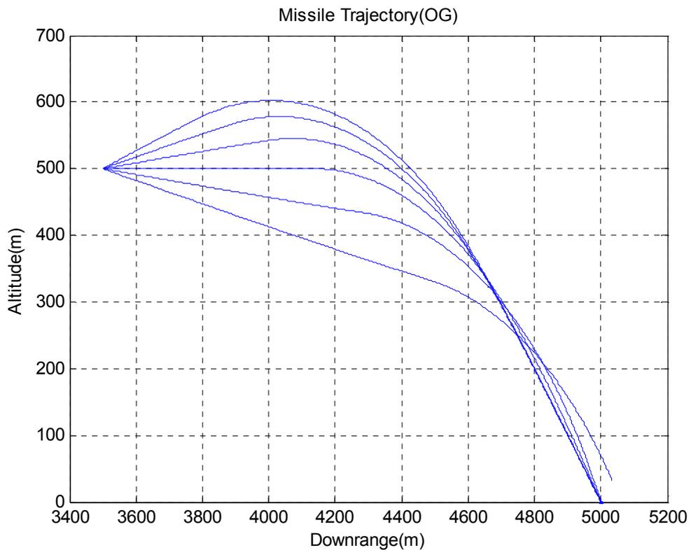
Figure 26 Missile Trajectories for Various TGH Angles (OG)
