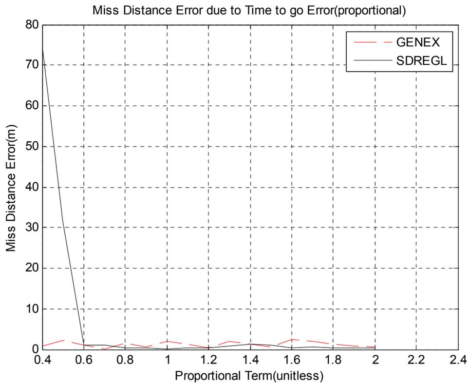
Figure 49 Miss Distance Error due to Time to go Error (proportional/stationary)
