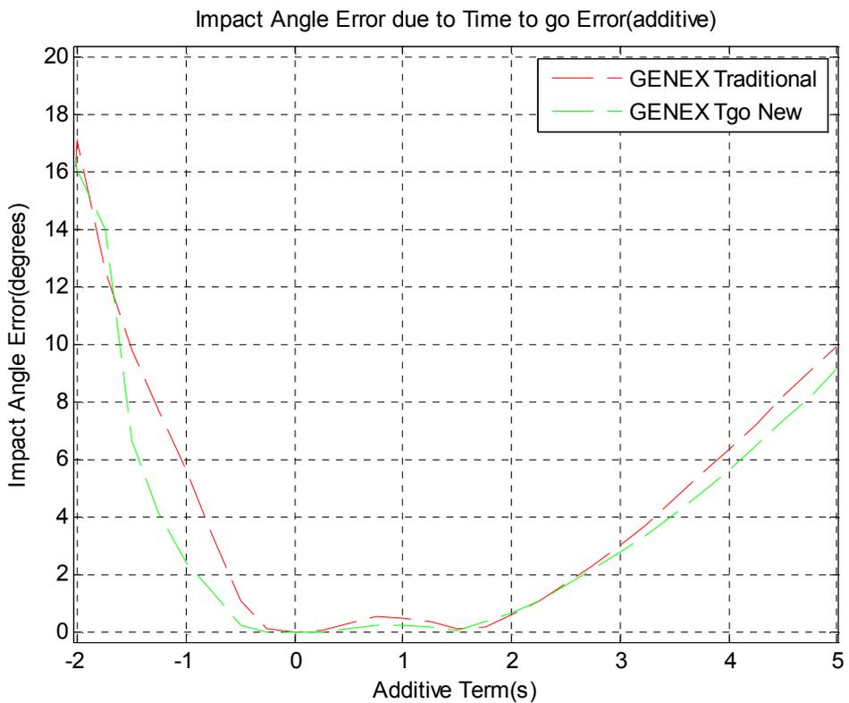
Figure 54 Impact Angle Error due to Time to go Error (additive/non-stationary)
