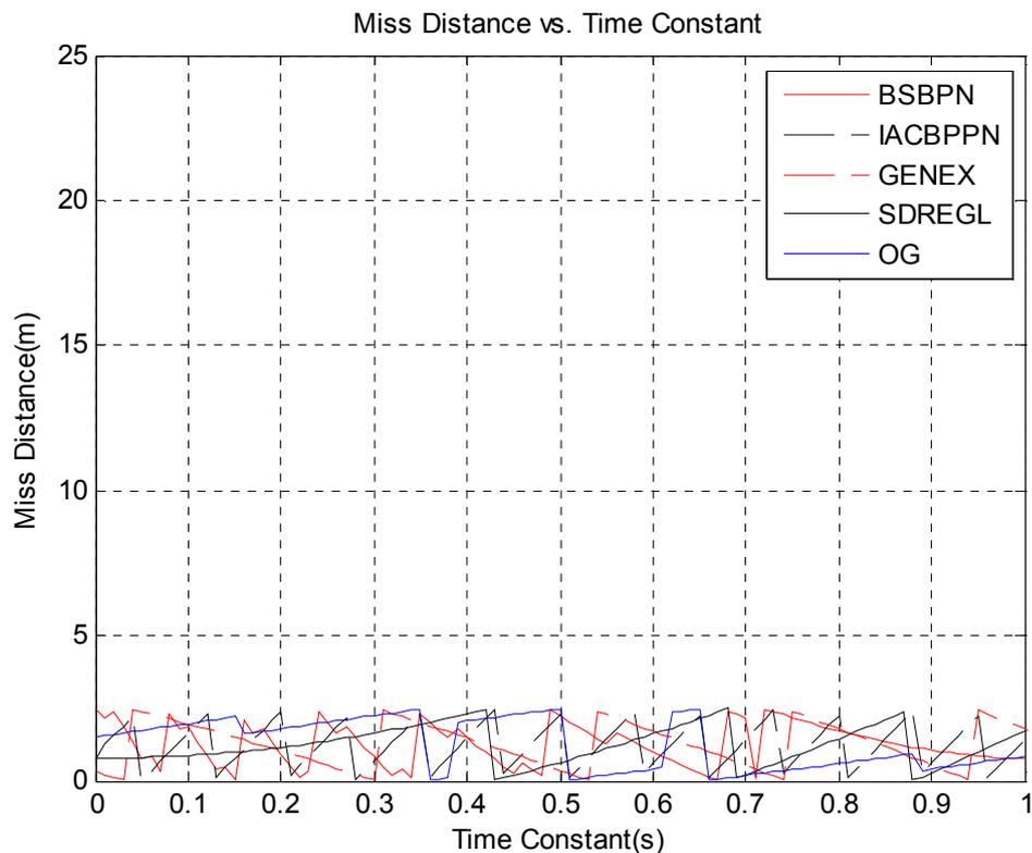
Figure 41 Miss Distance vs. Time Constant (stationary target)
