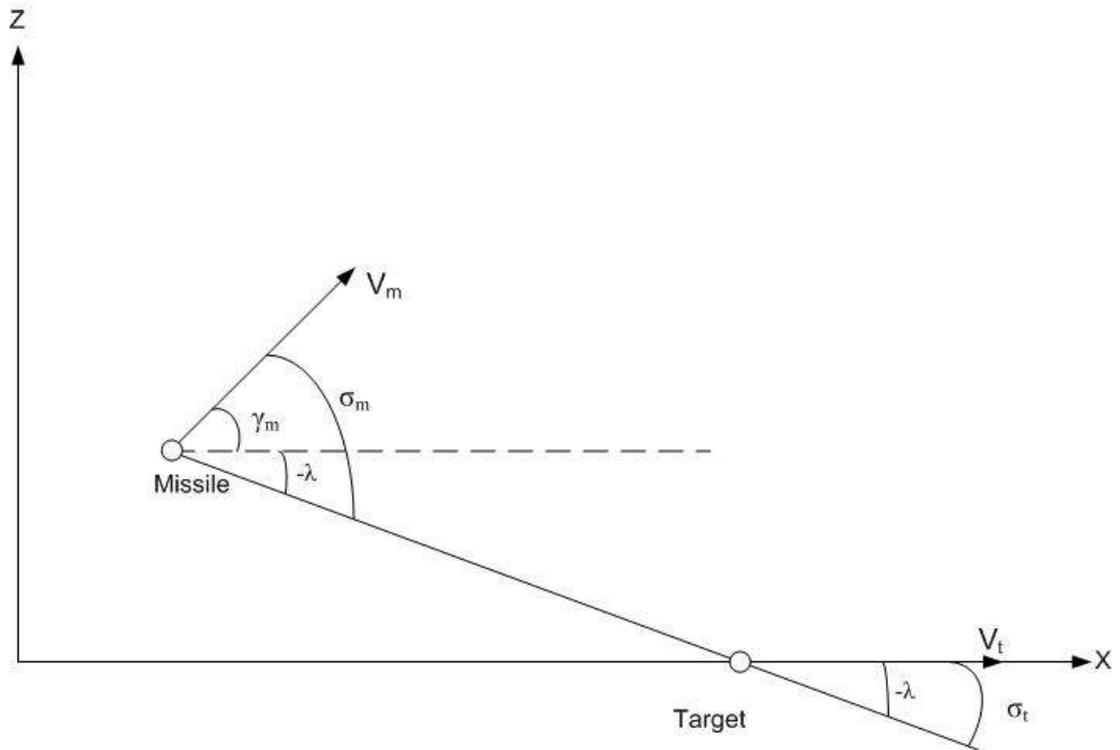
Figure 8 Engagement Schematic (refined)
