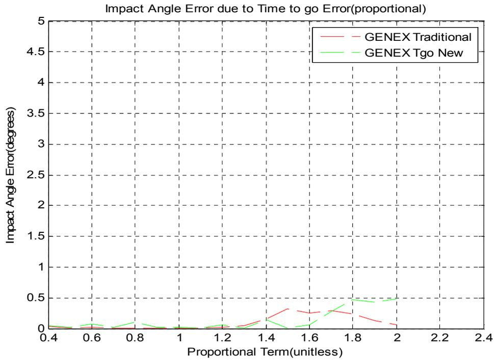
Figure 58 Impact Angle Error due to Time to go Error (proportional/non-stationary)
