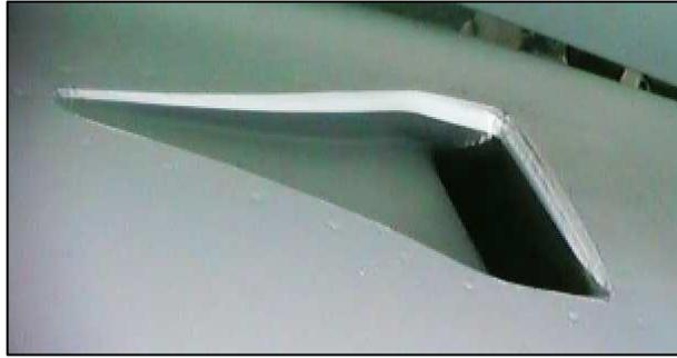
Figure 1-2 NACA-type Air Intake [5]
