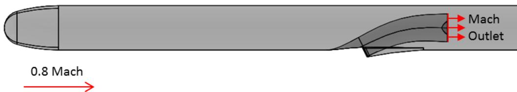
Figure 4-13 Mach Outlet Boundary Condition Surface
