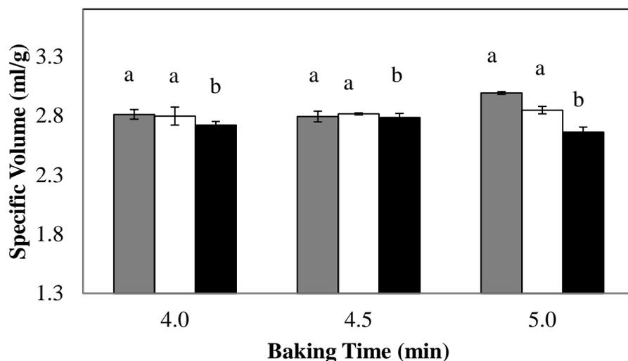
**Figure 3.6** Effect of baking time and lentil flour concentration on specific volume of cakes baked in MW-IR combination oven; (■):10%, (□):20%, (■):30%
