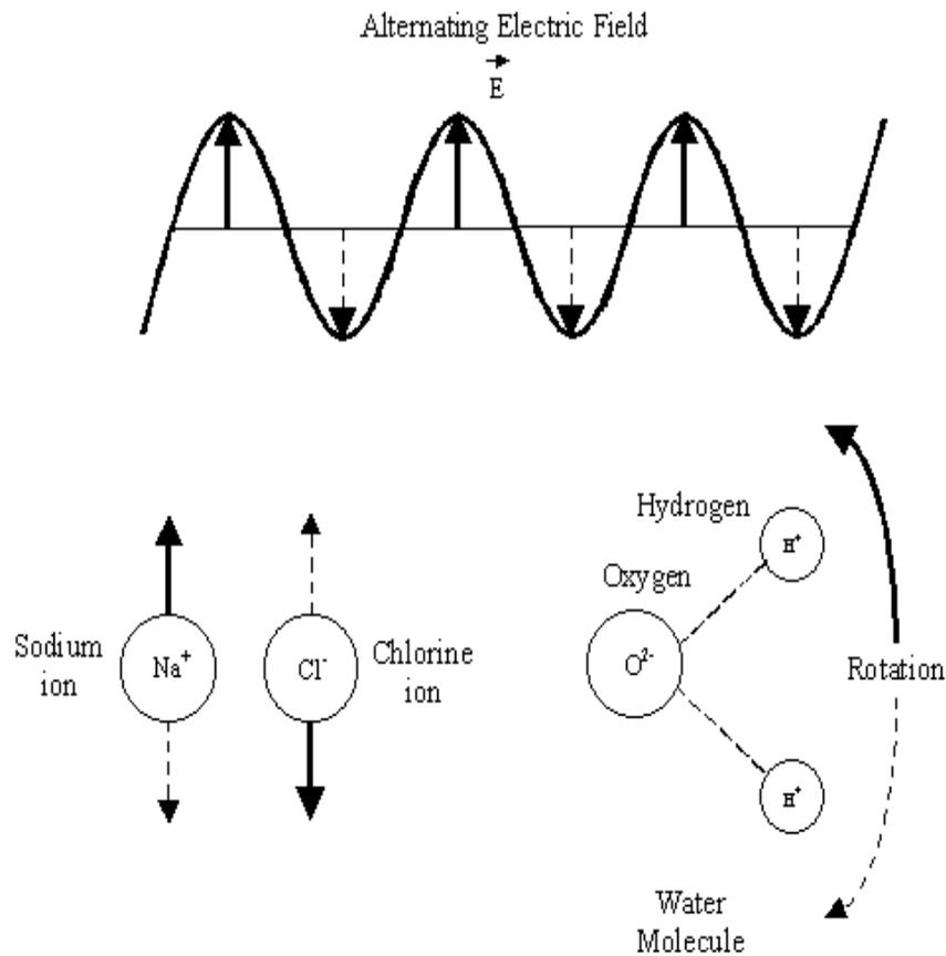
**Figure 1.4** Ionic conduction and dipolar rotation (Sahin & Sumnu, 2006)
