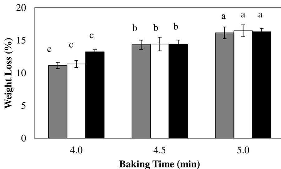
**Figure 3.3** Effect of baking time and chickpea flour concentration on weight loss of cakes baked in MW-IR combination oven; (■):10%, (□):20%, (■):30%
