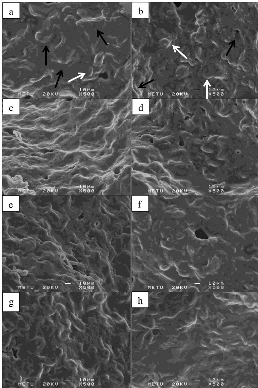
**Figure 3.33** SEM micrographs (500×) of cake samples baked in different ovens. a-wheat cake baked in conventional oven, b- wheat cake baked in MW-IR oven, c- lentil cake baked in conventional oven, d- lentil cake baked in MW-IR oven, e- chickpea cake baked in conventional oven, f- chickpea cake baked in MW-IR oven, g- pea cake baked in conventional oven, h- pea cake baked in MW-IR oven (Black arrows represent deformed starches, white arrows represent granular starches)
