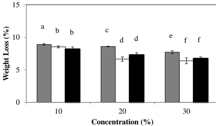
**Figure 3.1** Effect of legume flour type and concentration on weight loss of cakes baked in conventional oven for 24 min; (■): lentil flour, (□): chickpea flour, (▣): pea flour
