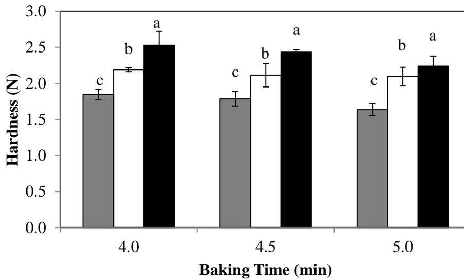
**Figure 3.15** Effect of baking time and chickpea flour concentration on hardness of cakes baked in MW-IR combination oven; (■):10%, (□):20%, (■):30%
