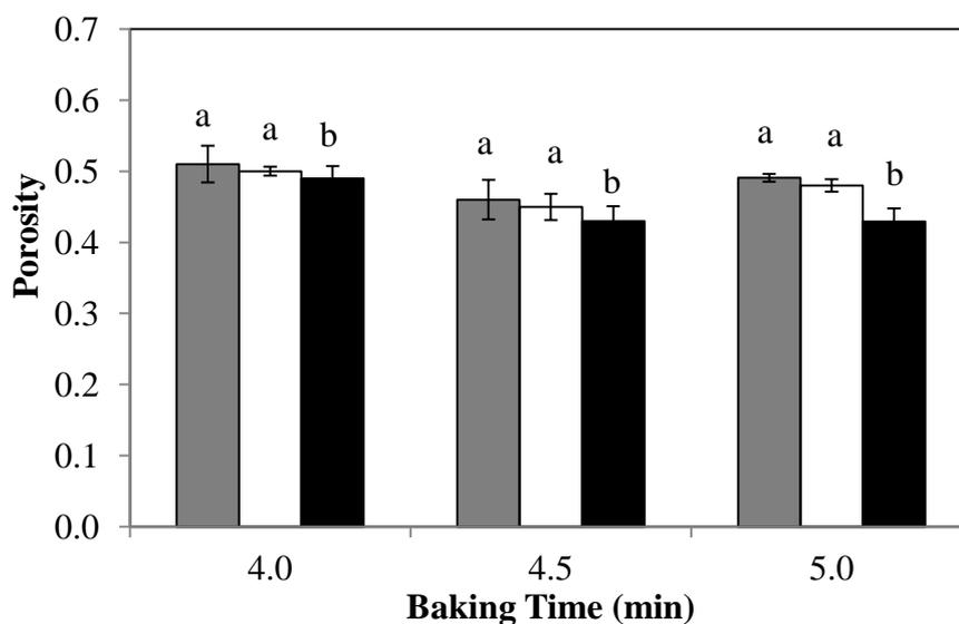
**Figure 3.10** Effect of baking time and lentil flour concentration on porosity of cakes baked in MW-IR combination oven; (■):10%, (□):20%, (■):30%
