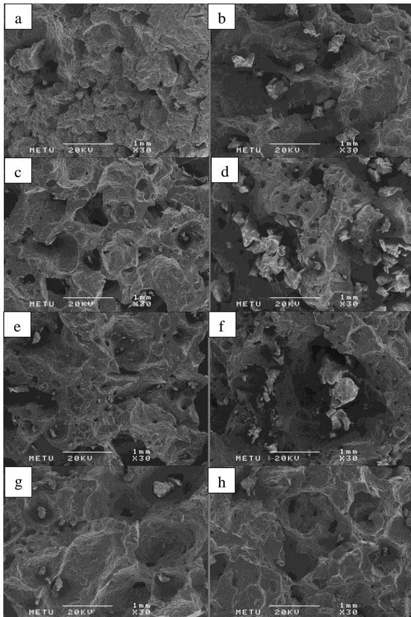
**Figure 3.32** SEM micrographs (30 $\times$ ) of cake samples baked in different ovens. a- control cake baked in conventional oven, b- control cake baked in MW-IR oven, c- lentil cake baked in conventional oven, d- lentil cake baked in MW-IR oven, e- chickpea cake baked in conventional oven, f- chickpea cake baked in MW-IR oven, g- pea cake baked in conventional oven, h- pea cake baked in MW-IR oven
